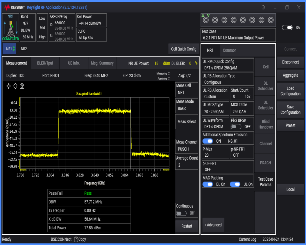
n77(3700-3980) SCS=30kHz DFT_QAM256 BW=90MHz Channel=656000 RB=240@0
