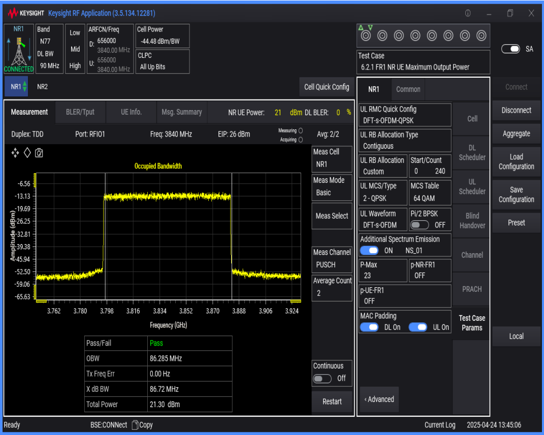
n77(3700-3980) SCS=30kHz DFT_QPSK BW=80MHz Channel=656000 RB=216@0
