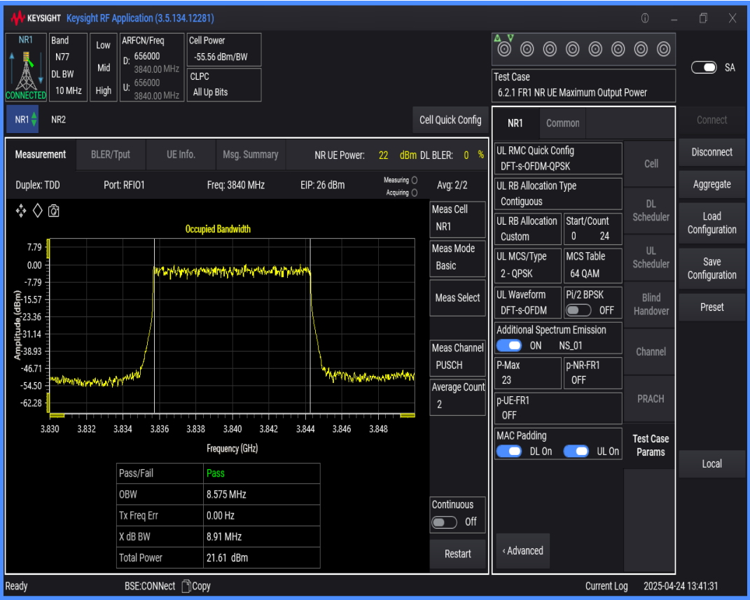
n77(3700-3980) SCS=30kHz DFT_QPSK BW=50MHz Channel=656000 RB=128@0
