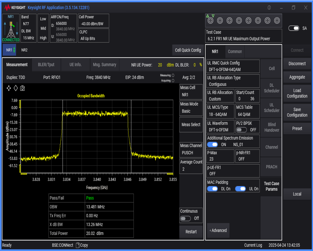
n77(3700-3980) SCS=30kHz DFT_QAM64 BW=100MHz Channel=656000 RB=270@0
