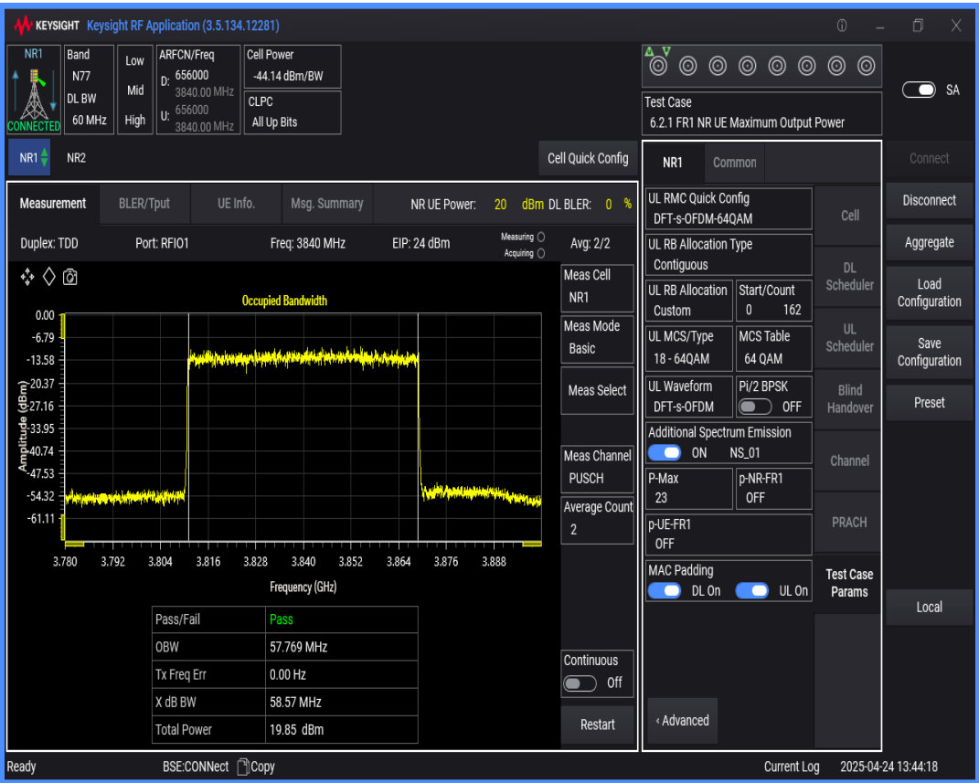
n77(3700-3980) SCS=30kHz DFT_QPSK BW=15MHz Channel=656000 RB=36@0
