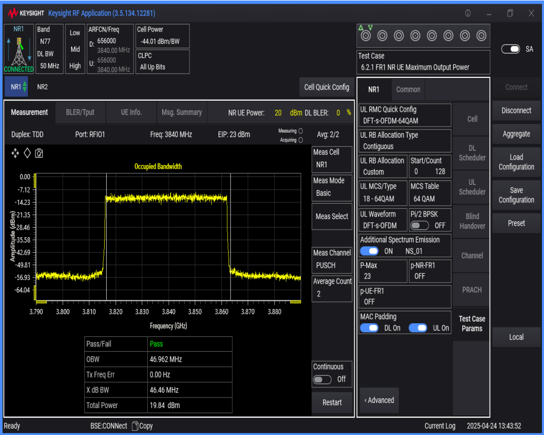
n77(3700-3980) SCS=30kHz DFT_QAM64 BW=60MHz Channel=656000 RB=162@0
