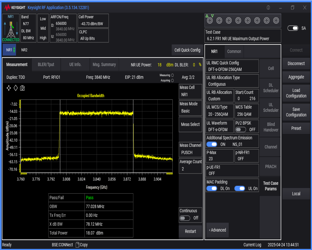
n77(3700-3980) SCS=30kHz DFT_QAM256 BW=60MHz Channel=656000 RB=162@0
