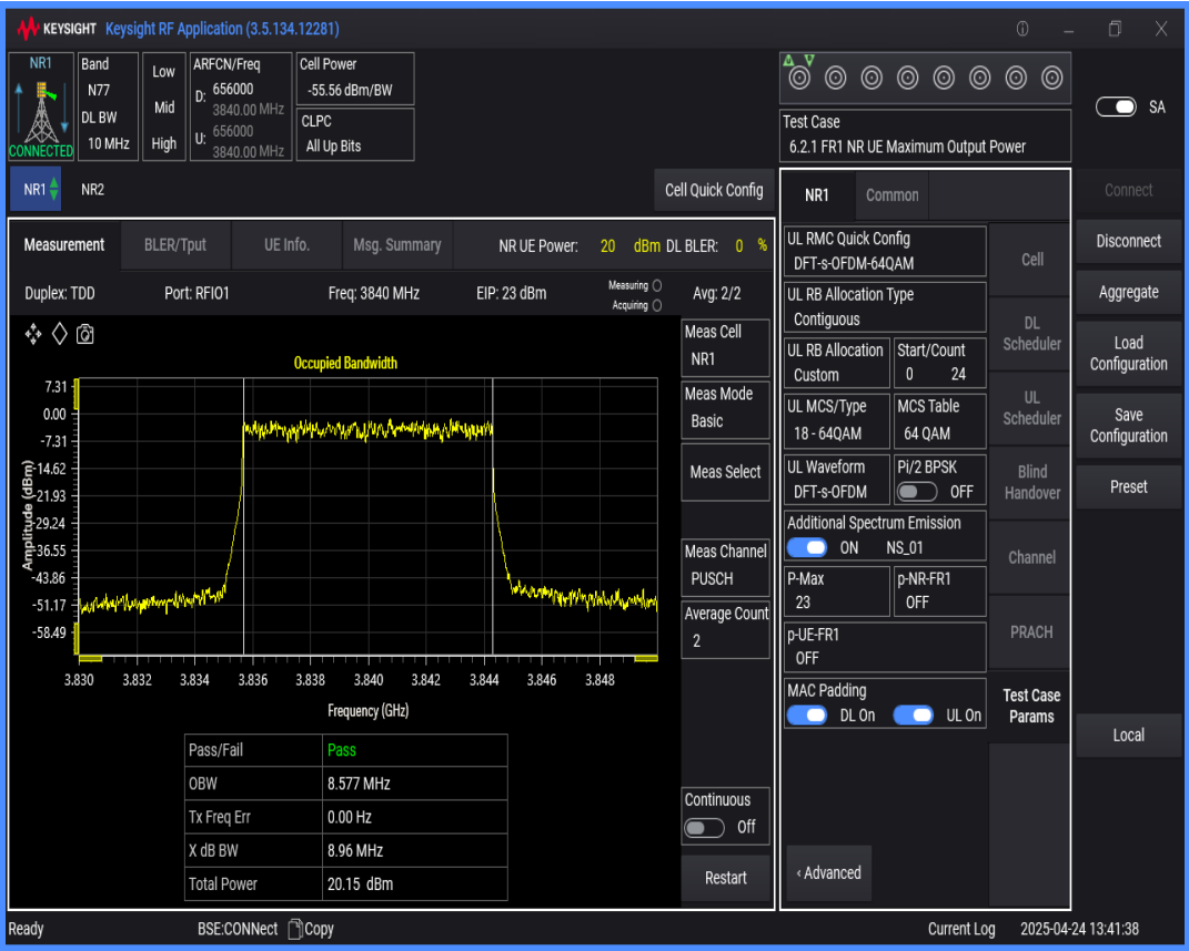
n77(3700-3980) SCS=30kHz DFT_QAM64 BW=40MHz Channel=656000 RB=100@0
