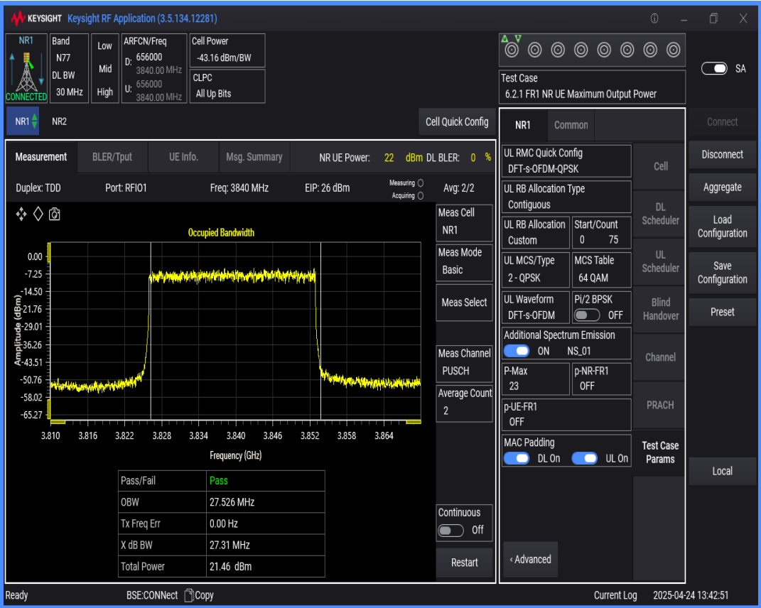
n77(3700-3980) SCS=30kHz DFT_QPSK BW=90MHz Channel=656000 RB=240@0
