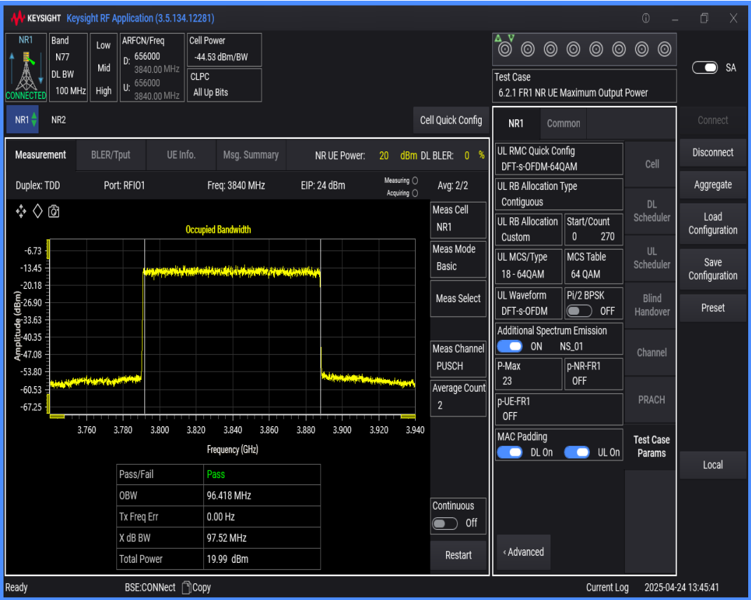
n77(3700-3980) SCS=30kHz DFT_QAM64 BW=10MHz Channel=656000 RB=24@0
