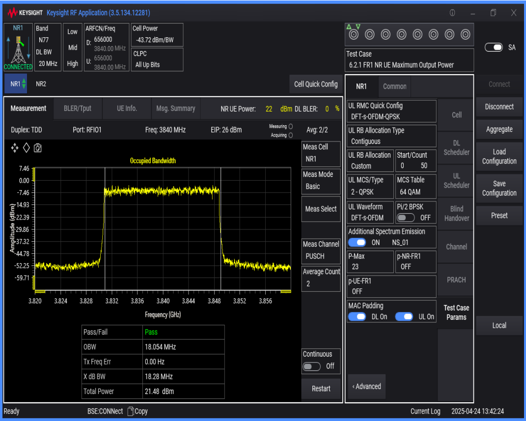
n77(3700-3980) SCS=30kHz DFT_QPSK BW=30MHz Channel=656000 RB=75@0
