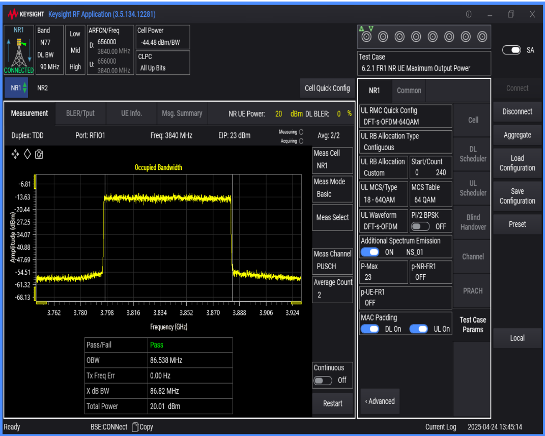
n77(3700-3980) SCS=30kHz DFT_QPSK BW=100MHz Channel=656000 RB=270@0
