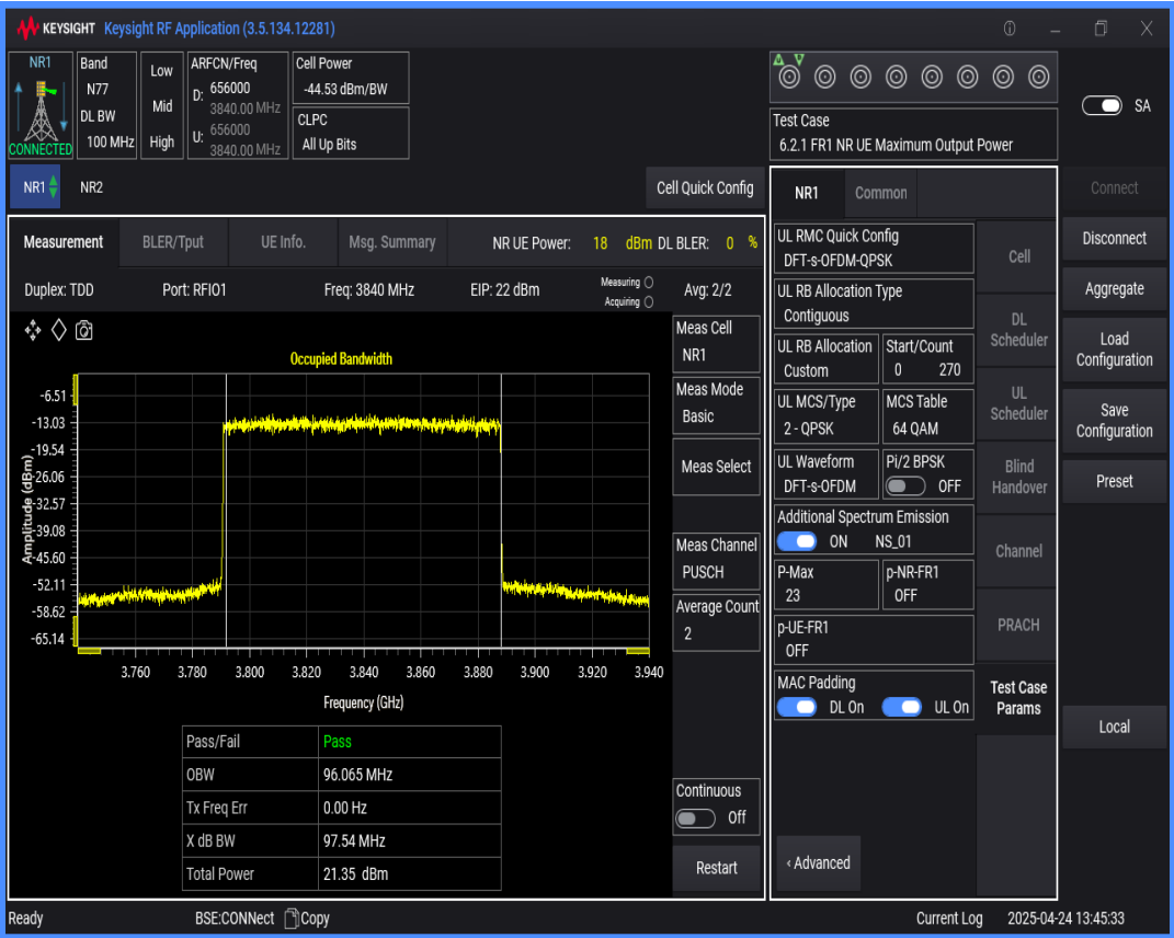
n77(3700-3980) SCS=30kHz DFT_QAM64 BW=80MHz Channel=656000 RB=216@0
