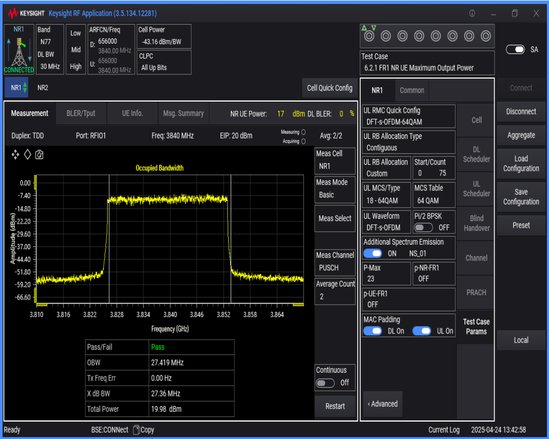
n77(3700-3980) SCS=30kHz DFT_QAM64 BW=15MHz Channel=656000 RB=36@0
