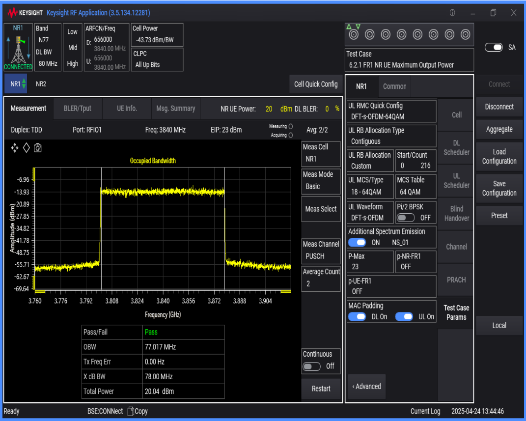
n77(3700-3980) SCS=30kHz DFT_QAM64 BW=50MHz Channel=656000 RB=128@0
