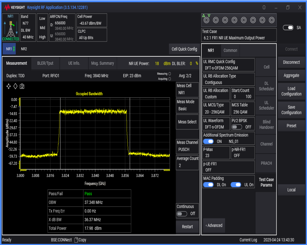
n77(3700-3980) SCS=30kHz DFT_QAM256 BW=50MHz Channel=656000 RB=128@0
