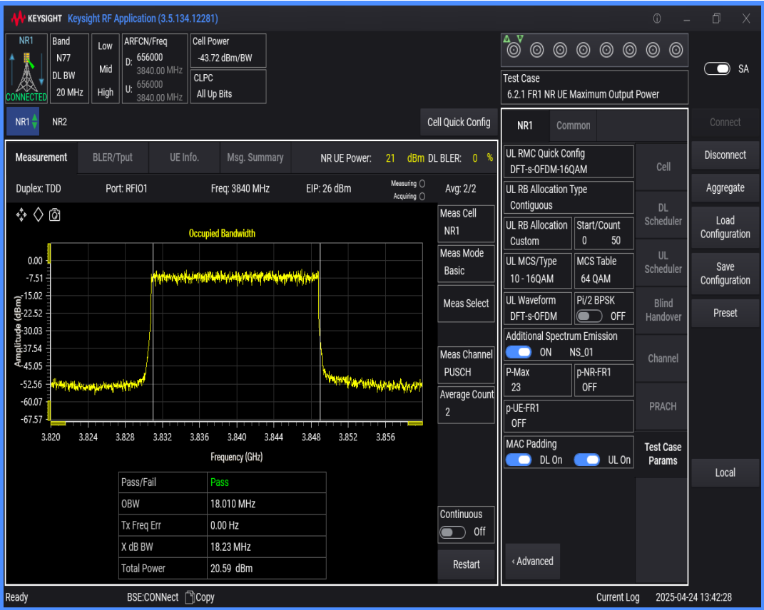
n77(3700-3980) SCS=30kHz DFT_QAM16 BW=30MHz Channel=656000 RB=75@0
