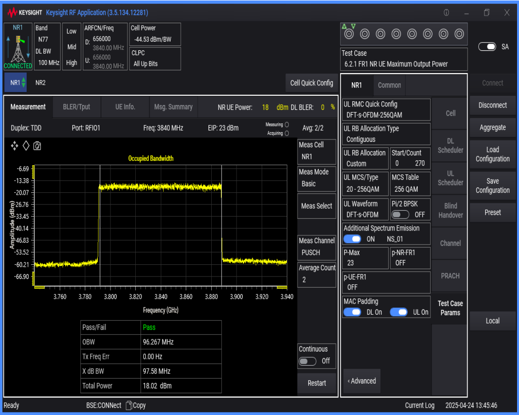
n77(3700-3980) SCS=30kHz DFT_QAM256 BW=40MHz Channel=656000 RB=100@0
