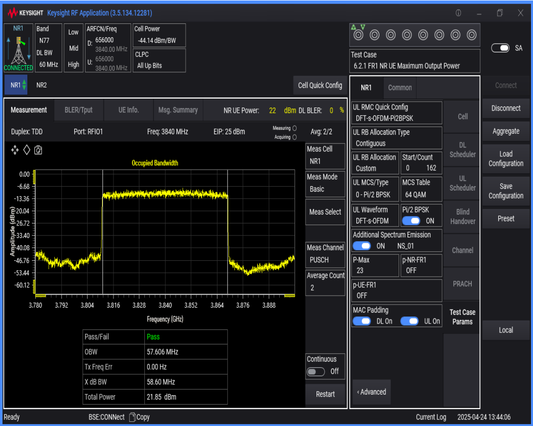
n77(3700-3980) SCS=30kHz DFT_BPSK BW=80MHz Channel=656000 RB=216@0
