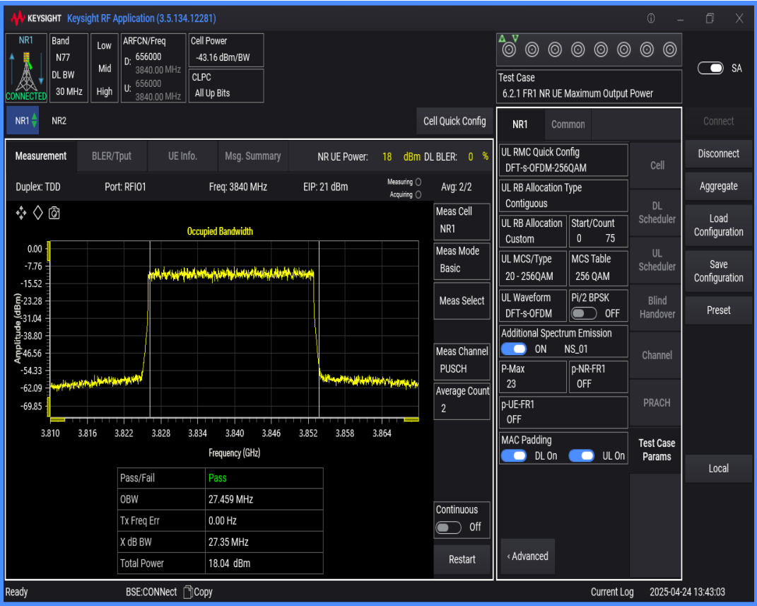
n77(3700-3980) SCS=30kHz DFT_QAM256 BW=80MHz Channel=656000 RB=216@0
