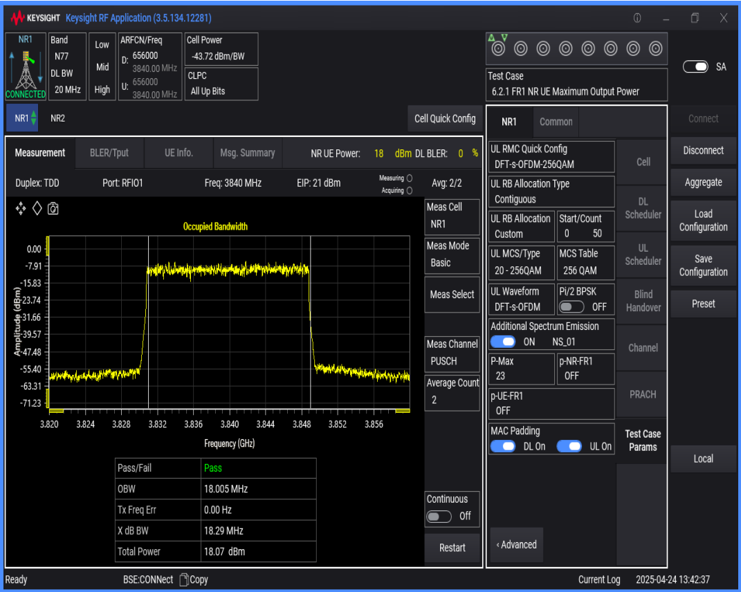
n77(3700-3980) SCS=30kHz DFT_QAM256 BW=30MHz Channel=656000 RB=75@0
