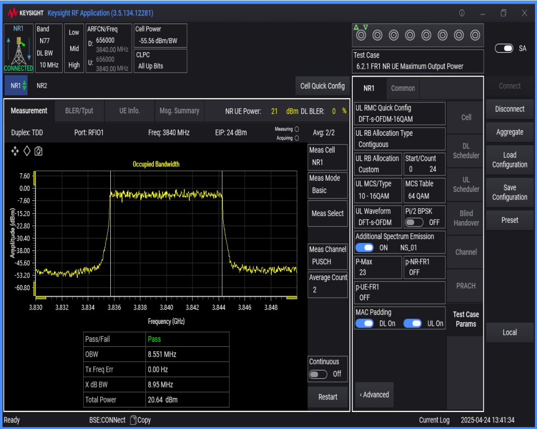
n77(3700-3980) SCS=30kHz DFT_QAM16 BW=15MHz Channel=656000 RB=36@0
