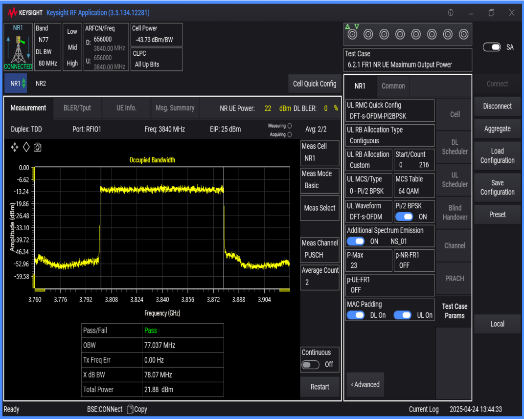
n77(3700-3980) SCS=30kHz DFT_BPSK BW=90MHz Channel=656000 RB=240@0
