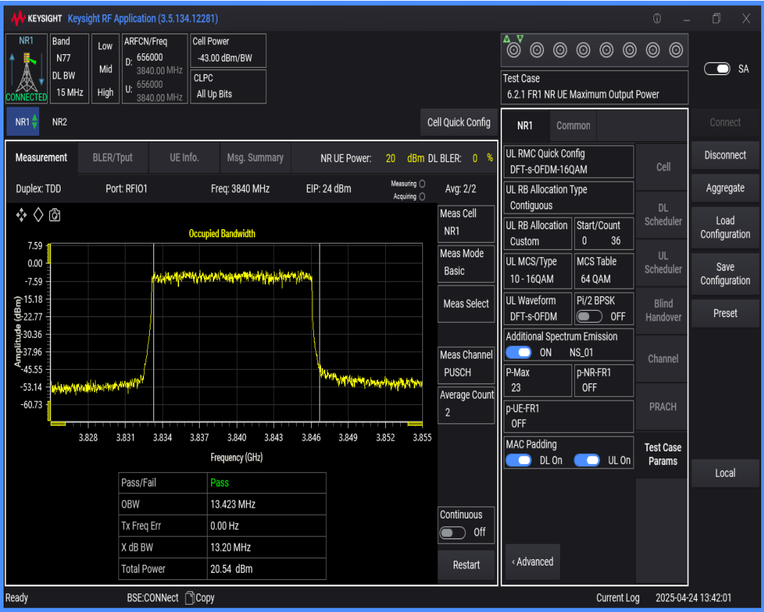
n77(3700-3980) SCS=30kHz DFT_QAM16 BW=40MHz Channel=656000 RB=100@0
