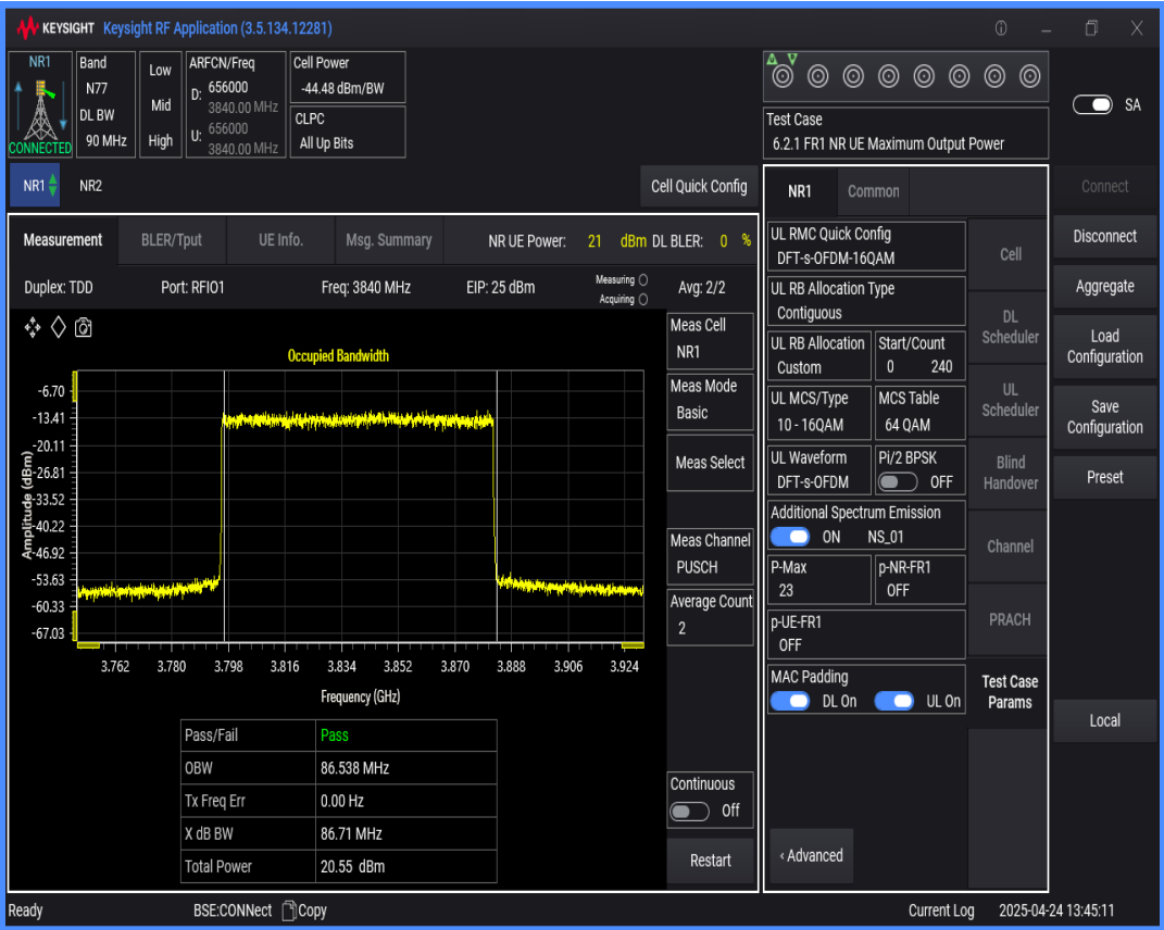
n77(3700-3980) SCS=30kHz DFT_QAM256 BW=100MHz Channel=656000 RB=270@0
