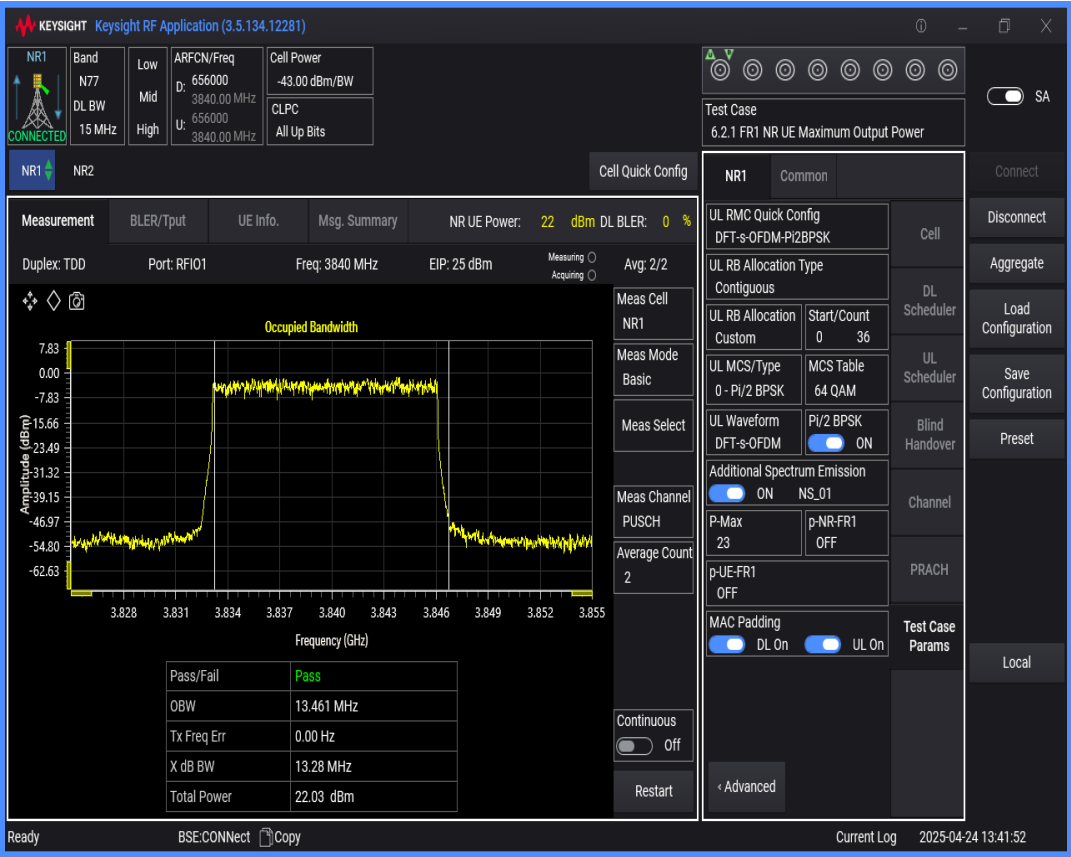
n77(3700-3980) SCS=30kHz DFT_BPSK BW=30MHz Channel=656000 RB=75@0
