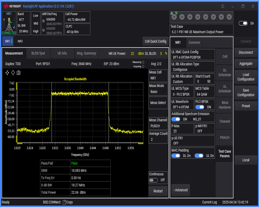
n77(3700-3980) SCS=30kHz DFT_BPSK BW=40MHz Channel=656000 RB=100@0
