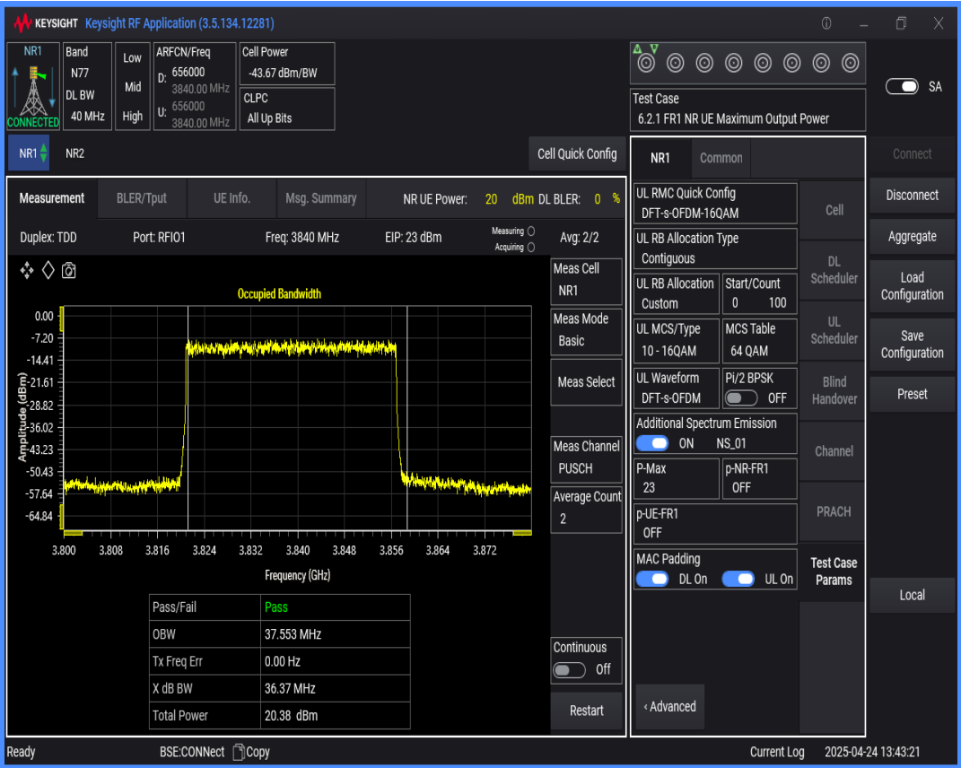
n77(3700-3980) SCS=30kHz DFT_QAM16 BW=50MHz Channel=656000 RB=128@0
