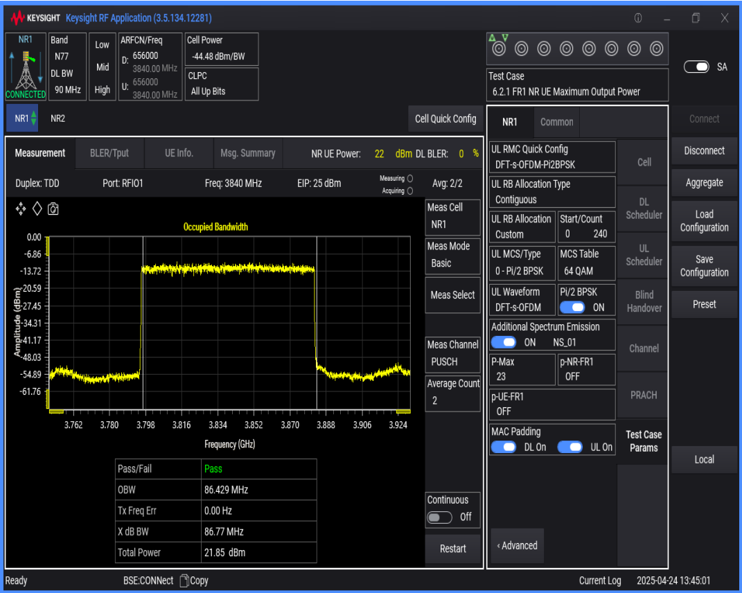
n77(3700-3980) SCS=30kHz DFT_QAM16 BW=100MHz Channel=656000 RB=270@0
