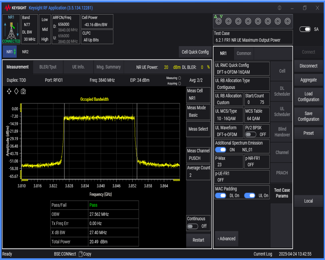
n77(3700-3980) SCS=30kHz DFT_QAM16 BW=60MHz Channel=656000 RB=162@0
