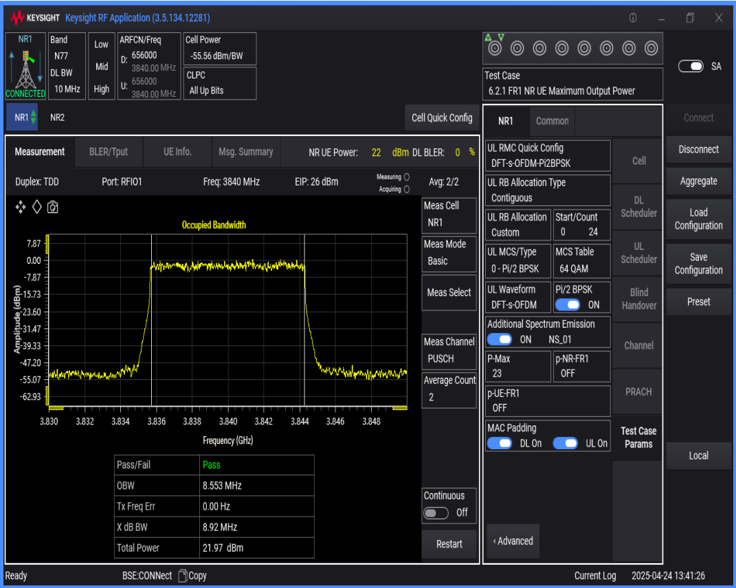
n77(3700-3980) SCS=30kHz DFT_BPSK BW=15MHz Channel=656000 RB=36@0
