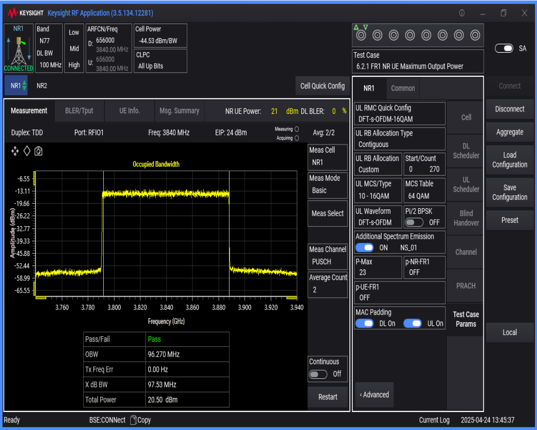
n77(3700-3980) SCS=30kHz DFT_QAM16 BW=10MHz Channel=656000 RB=24@0
