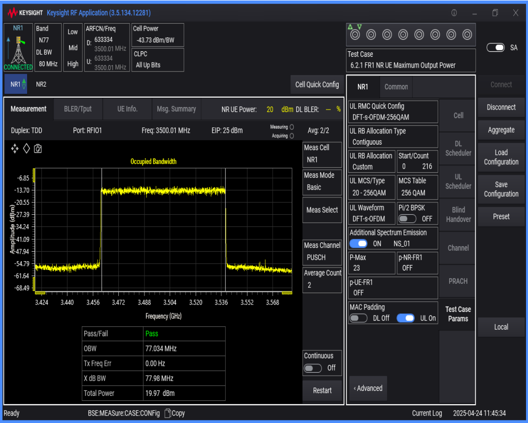
n77(3450-3550) SCS=30kHz DFT_QAM256 BW=50MHz Channel=633334 RB=128@0
