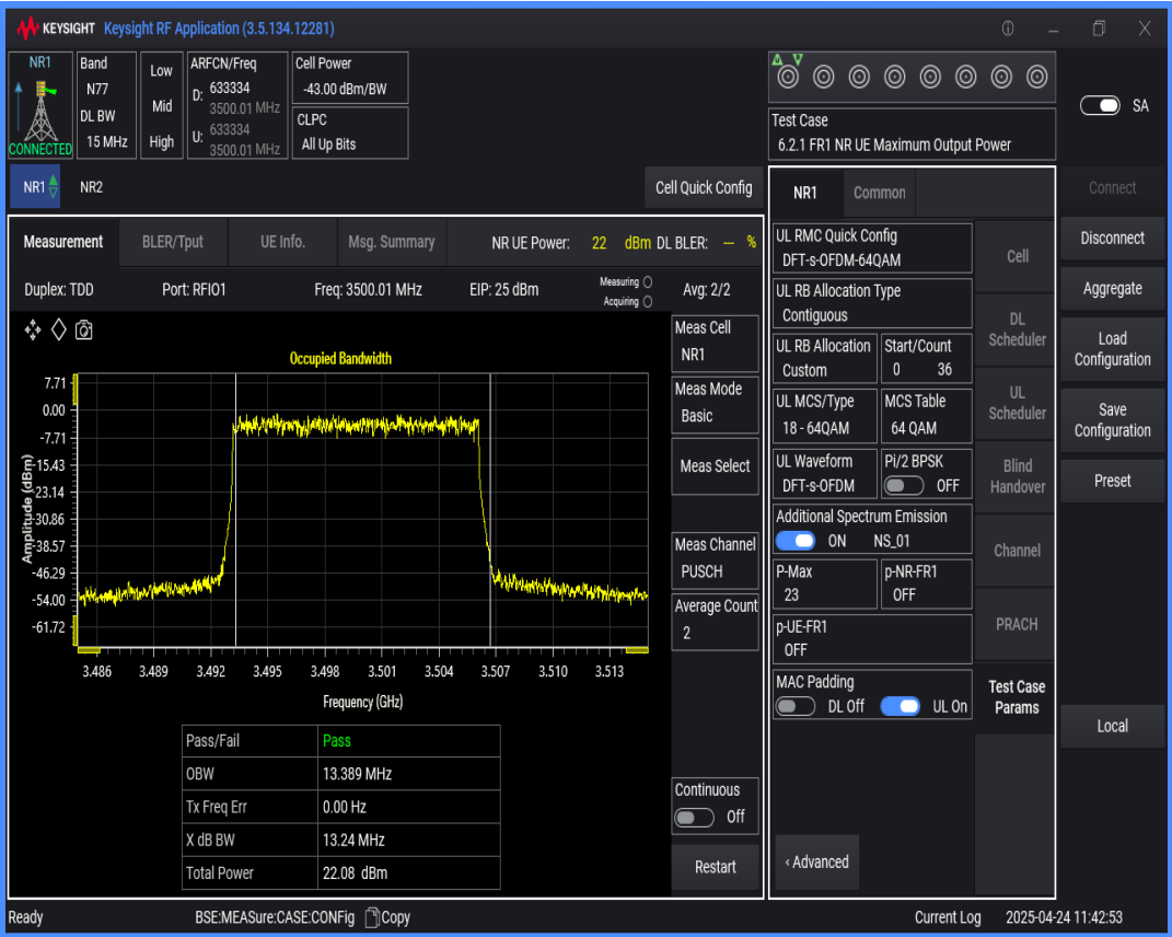
n77(3450-3550) SCS=30kHz DFT_QAM64 BW=10MHz Channel=633334 RB=24@0
