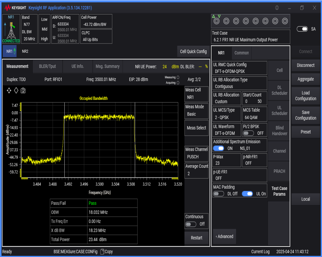
n77(3450-3550) SCS=30kHz DFT_QPSK BW=30MHz Channel=633334 RB=75@0
