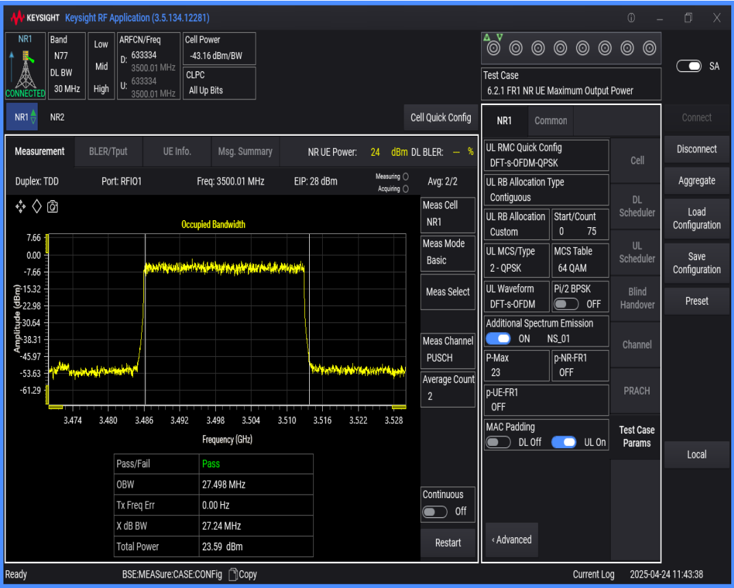
n77(3450-3550) SCS=30kHz DFT_QPSK BW=50MHz Channel=633334 RB=128@0
