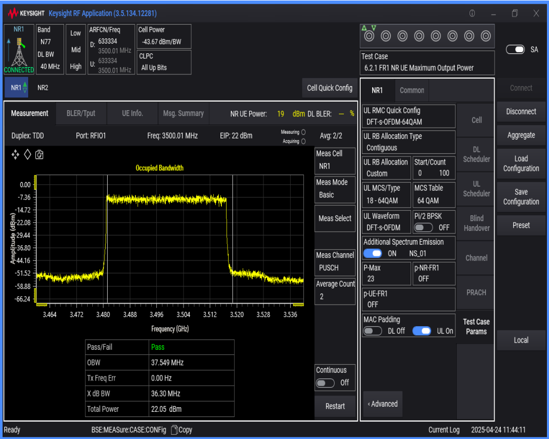
n77(3450-3550) SCS=30kHz DFT_QAM64 BW=50MHz Channel=633334 RB=128@0
