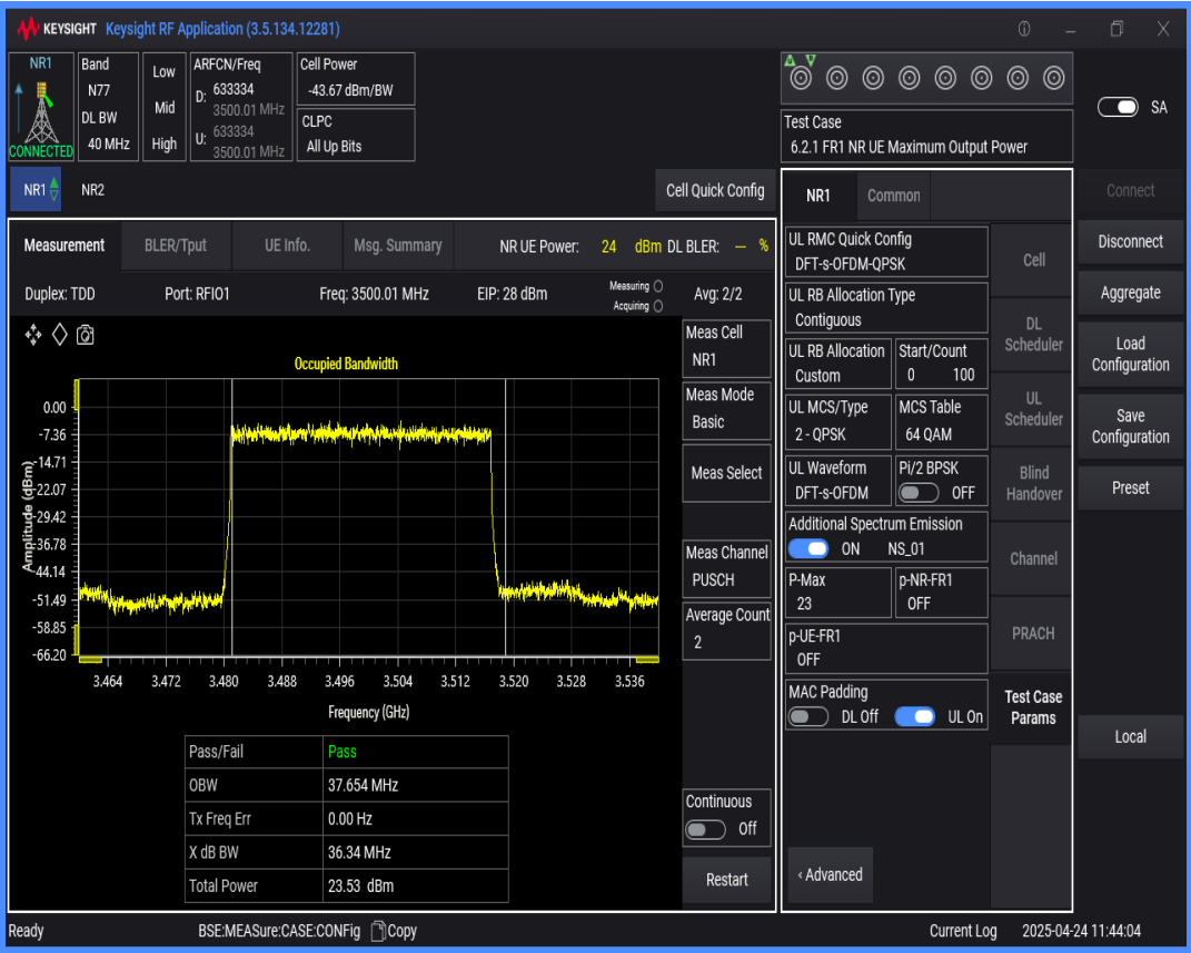
n77(3450-3550) SCS=30kHz DFT_QPSK BW=80MHz Channel=633334 RB=216@0
