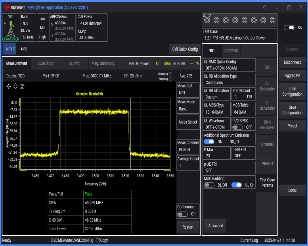
n77(3450-3550) SCS=30kHz DFT_QAM64 BW=80MHz Channel=633334 RB=216@0
