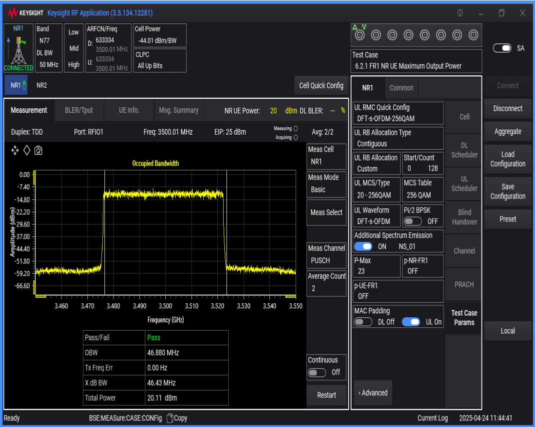
n77(3450-3550) SCS=30kHz DFT_QAM256 BW=60MHz Channel=633334 RB=162@0
