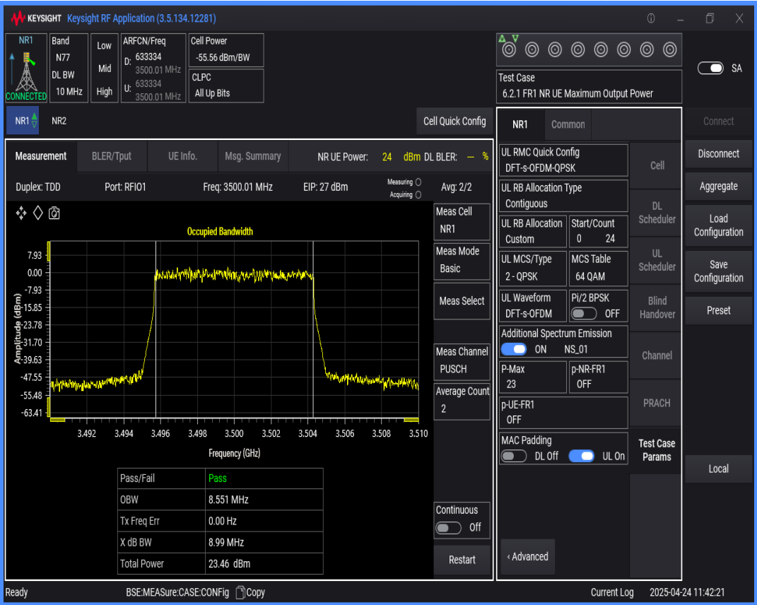
n77(3450-3550) SCS=30kHz DFT_QPSK BW=15MHz Channel=633334 RB=36@0
