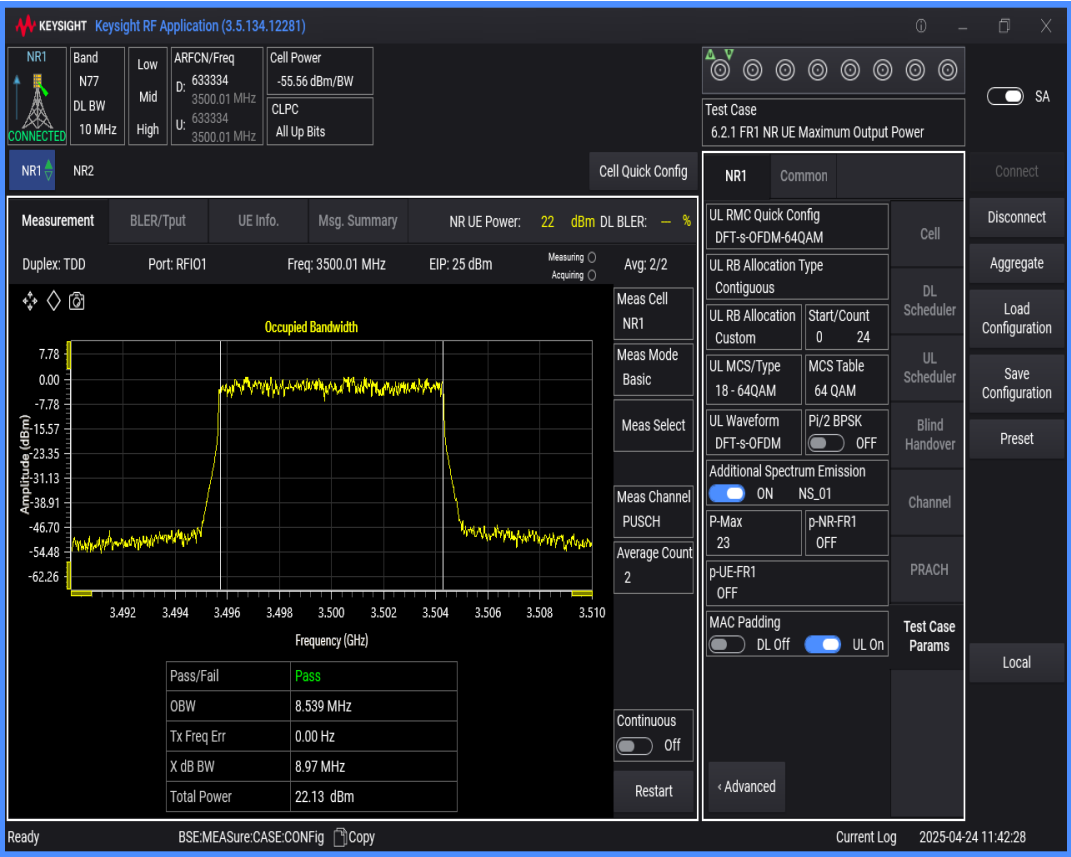
n77(3450-3550) SCS=30kHz DFT_QAM64 BW=30MHz Channel=633334 RB=75@0
