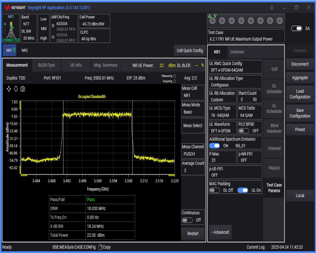
n77(3450-3550) SCS=30kHz DFT_QAM64 BW=40MHz Channel=633334 RB=100@0
