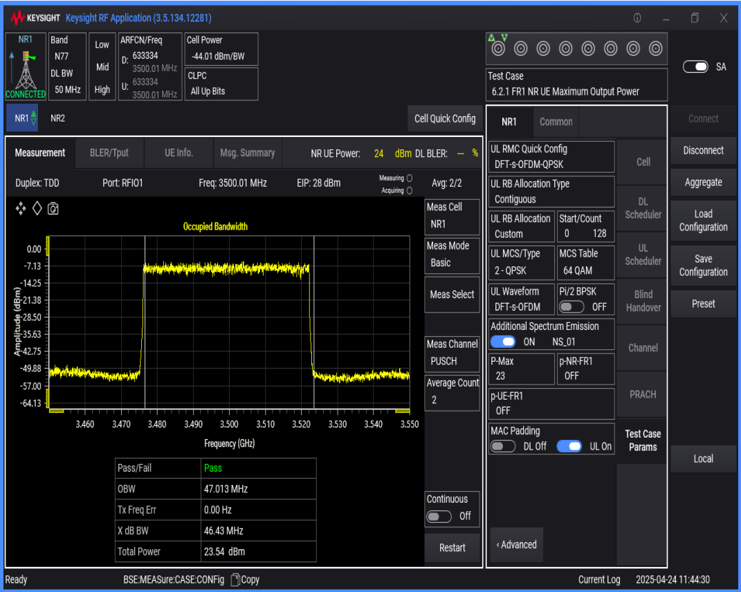
n77(3450-3550) SCS=30kHz DFT_QPSK BW=40MHz Channel=633334 RB=100@0
