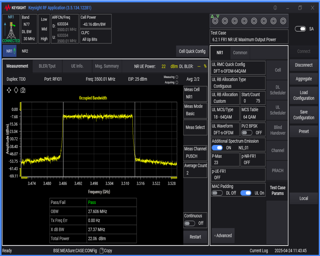
n77(3450-3550) SCS=30kHz DFT_QAM64 BW=20MHz Channel=633334 RB=50@0
