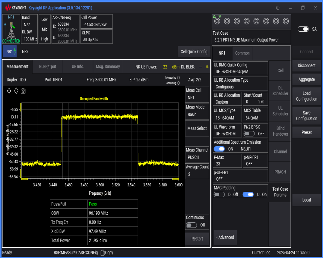
n77(3450-3550) SCS=30kHz DFT_QAM256 BW=80MHz Channel=633334 RB=216@0
