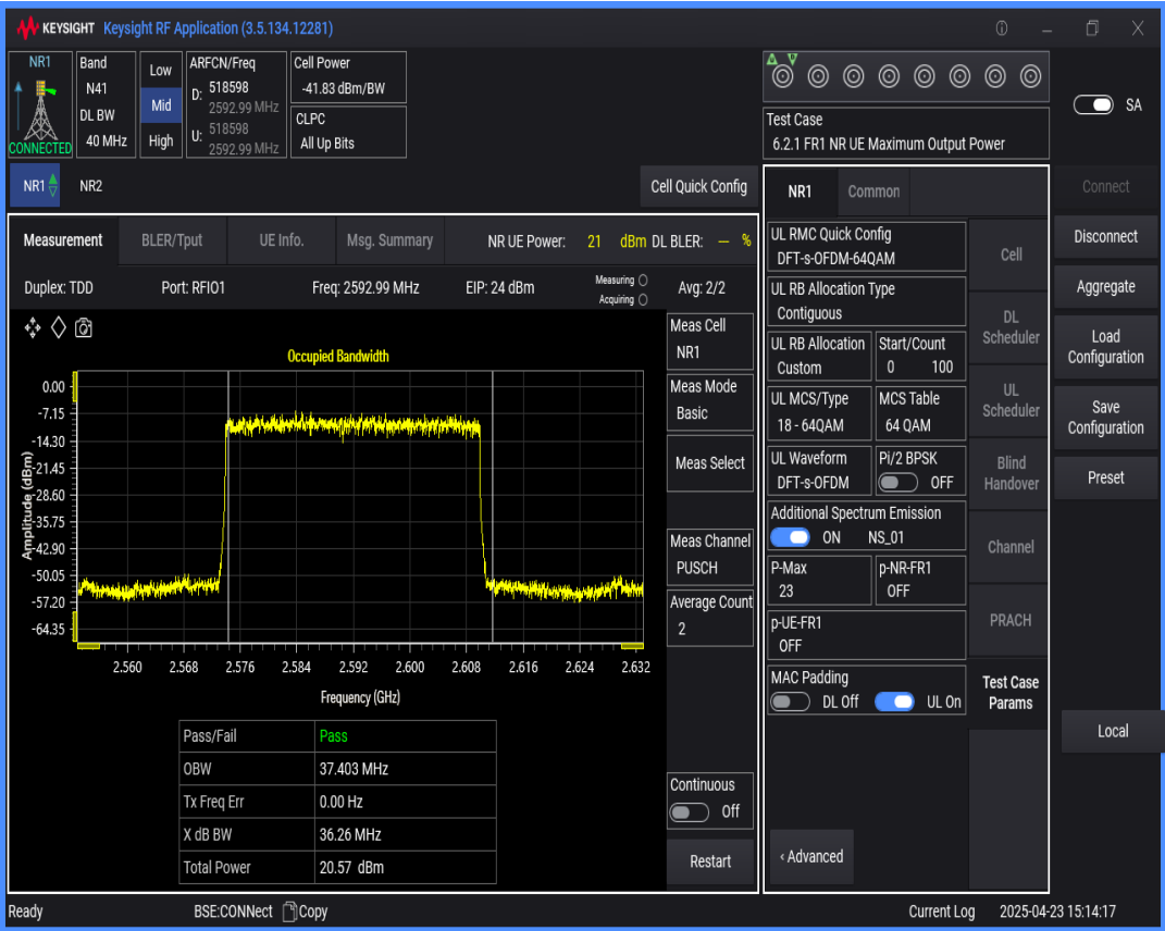
n41 SCS=30kHz DFT_QAM64 BW=50MHz Channel=518598 RB=128@0
