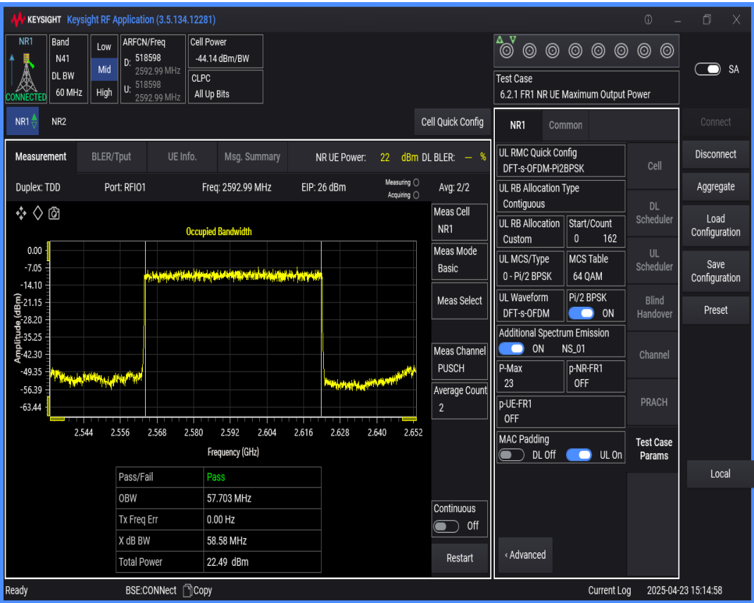
n41 SCS=30kHz DFT_BPSK BW=90MHz Channel=518598 RB=240@0
