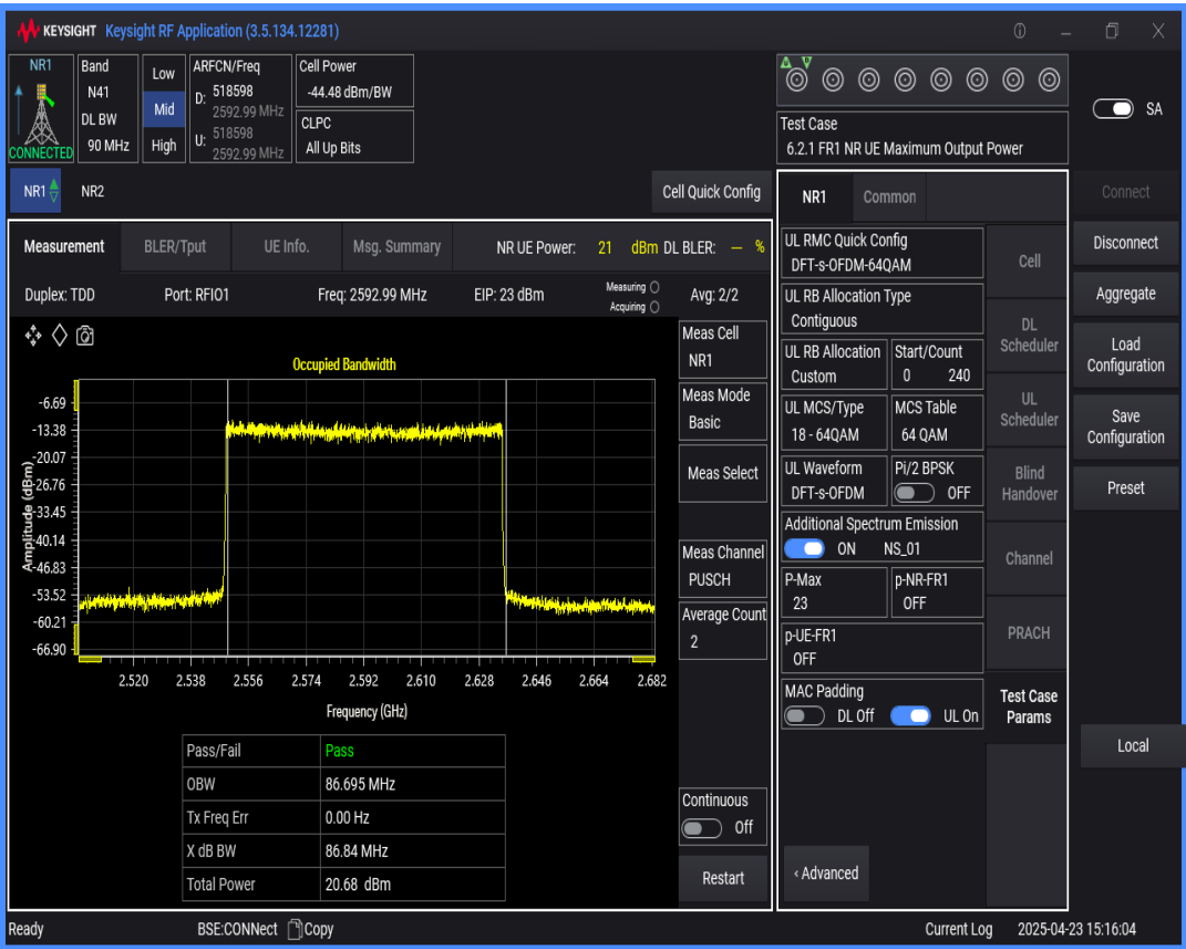
n41 SCS=30kHz DFT_QAM64 BW=80MHz Channel=518598 RB=216@0
