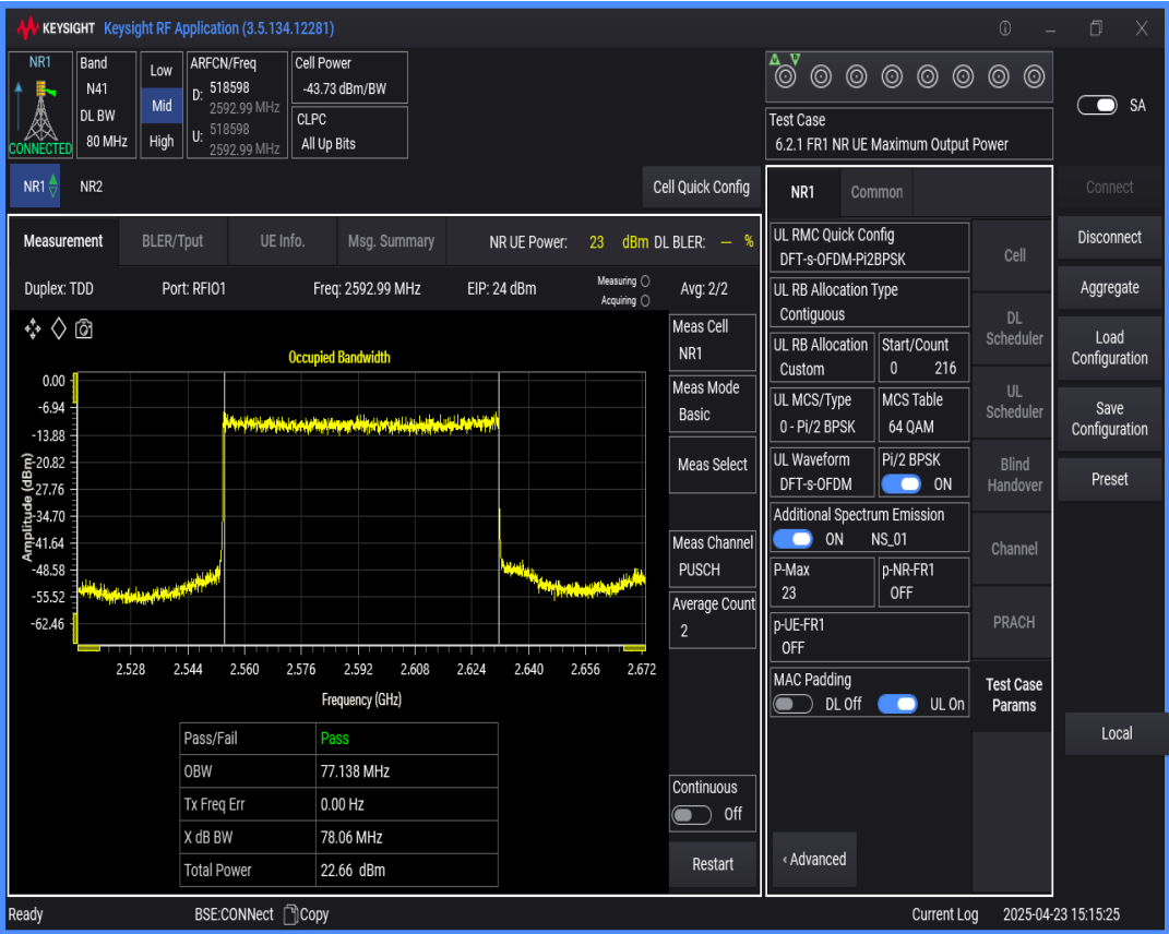
n41 SCS=30kHz DFT_BPSK BW=60MHz Channel=518598 RB=162@0
