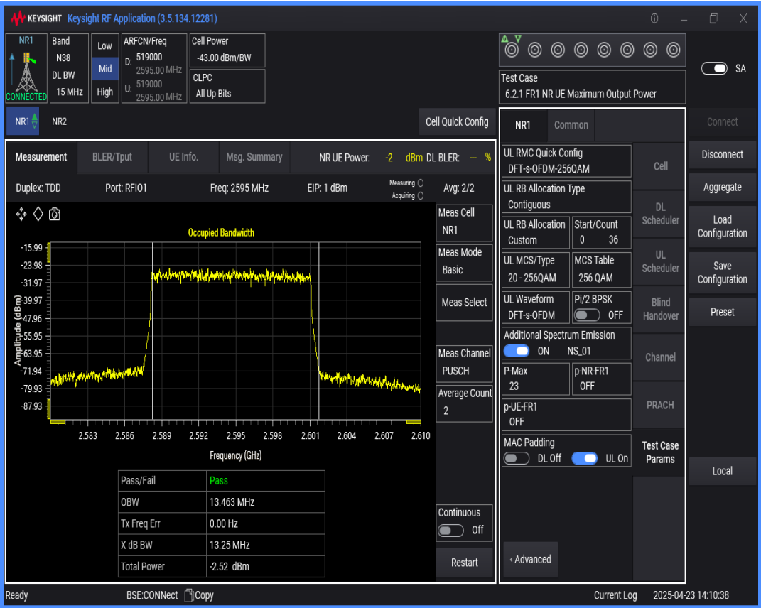
n38 SCS=30kHz DFT_QAM64 BW=15MHz Channel=519000 RB=36@0
