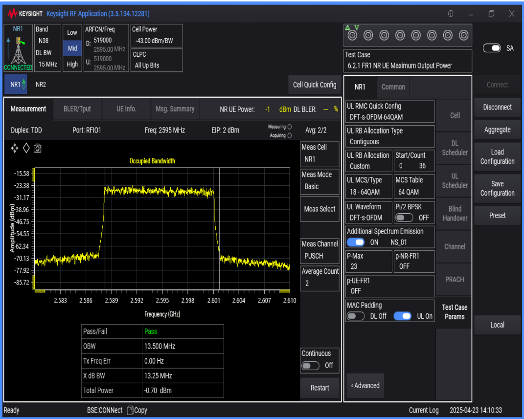
n38 SCS=30kHz DFT_QAM64 BW=10MHz Channel=519000 RB=24@0
