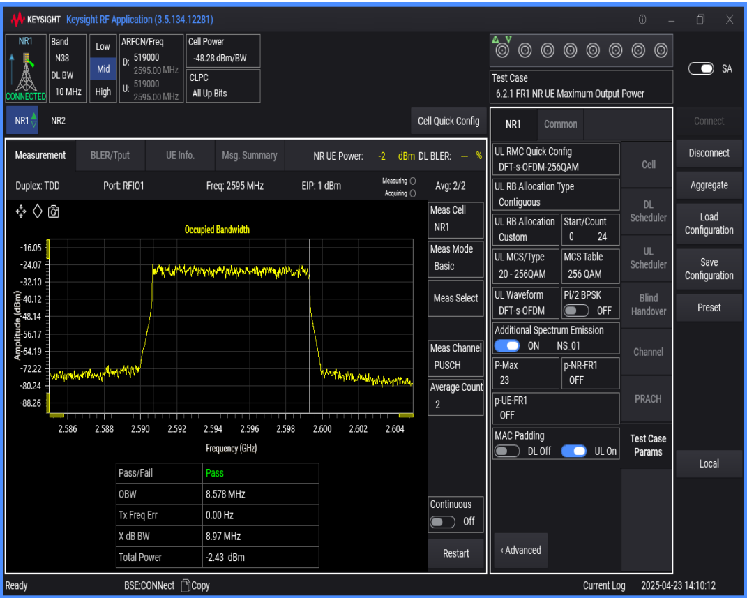
n38 SCS=30kHz DFT_QAM256 BW=15MHz Channel=519000 RB=36@0
