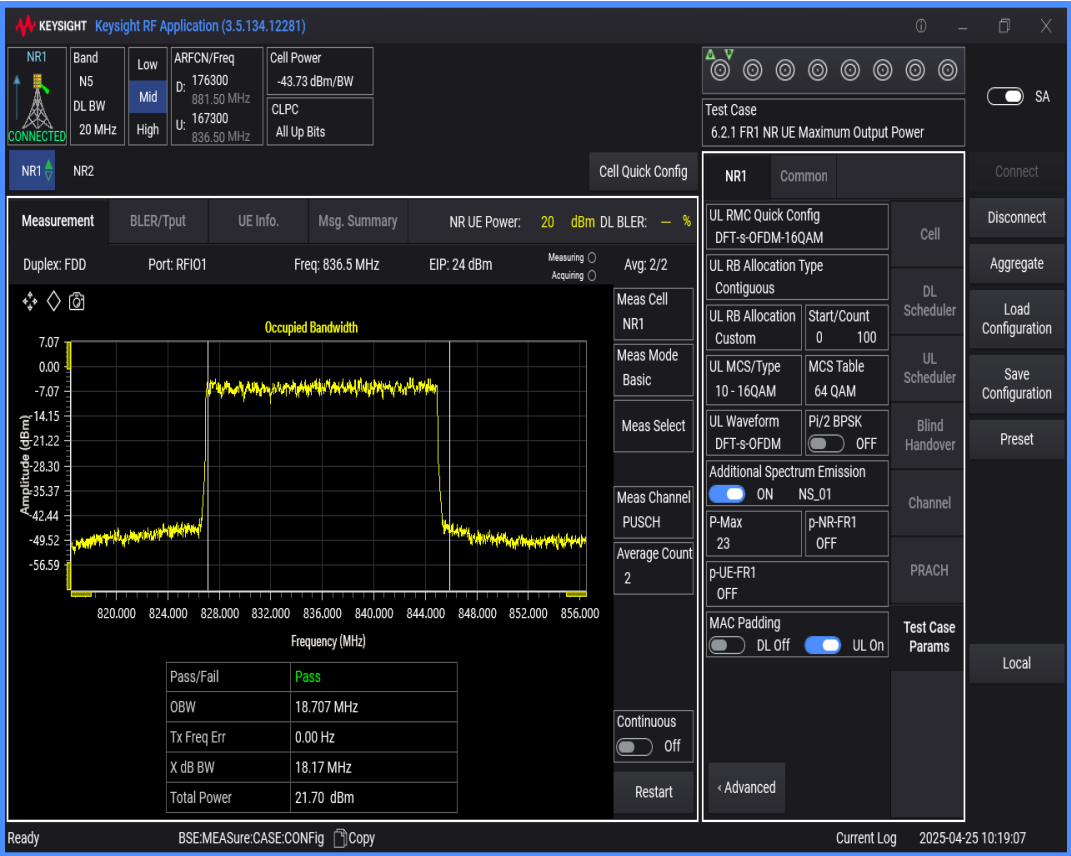
n5 SCS=15kHz DFT_QAM16 BW=5MHz Channel=167300 RB=25@0
