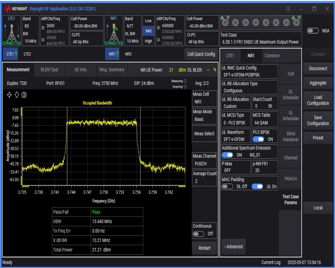
n77 SCS=30kHz DFT_QAM16 BW=15MHz Channel=650000 RB=36@0
