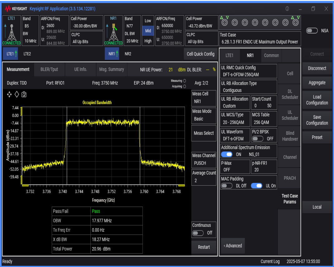
n77 SCS=30kHz DFT_QAM16 BW=80MHz Channel=650000 RB=216@0
