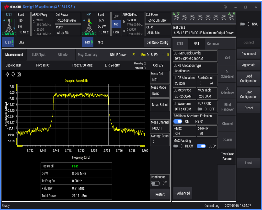
n77 SCS=30kHz DFT_QAM256 BW=40MHz Channel=650000 RB=100@0
