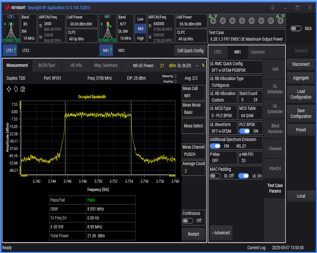
n77 SCS=30kHz DFT_BPSK BW=15MHz Channel=650000 RB=36@0
