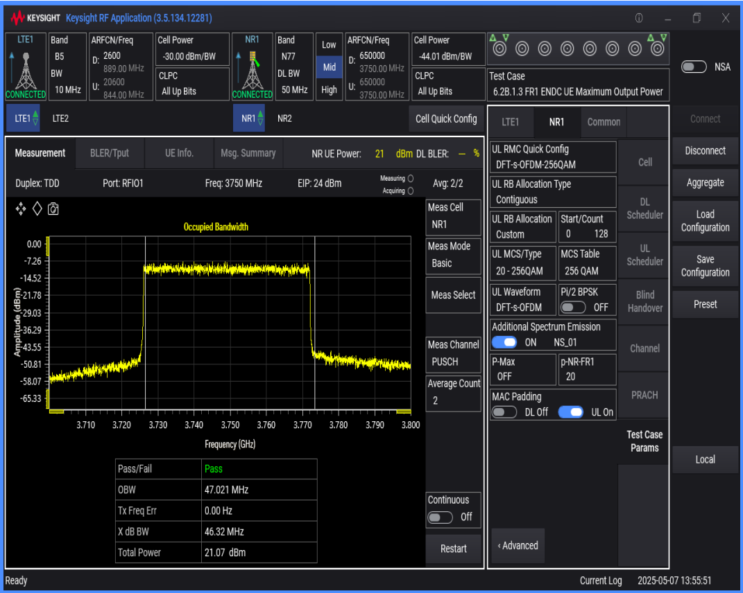
n77 SCS=30kHz DFT_QAM256 BW=90MHz Channel=650000 RB=240@0
