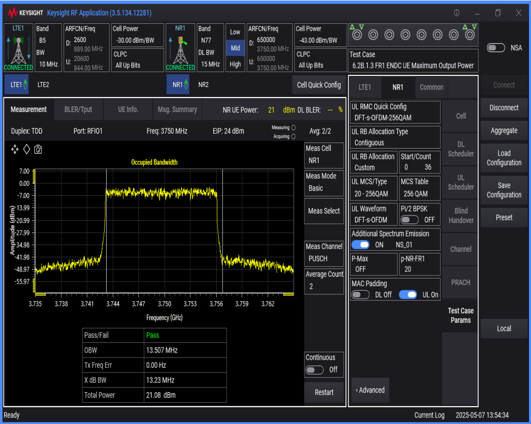
n77 SCS=30kHz DFT_QAM256 BW=10MHz Channel=650000 RB=24@0
