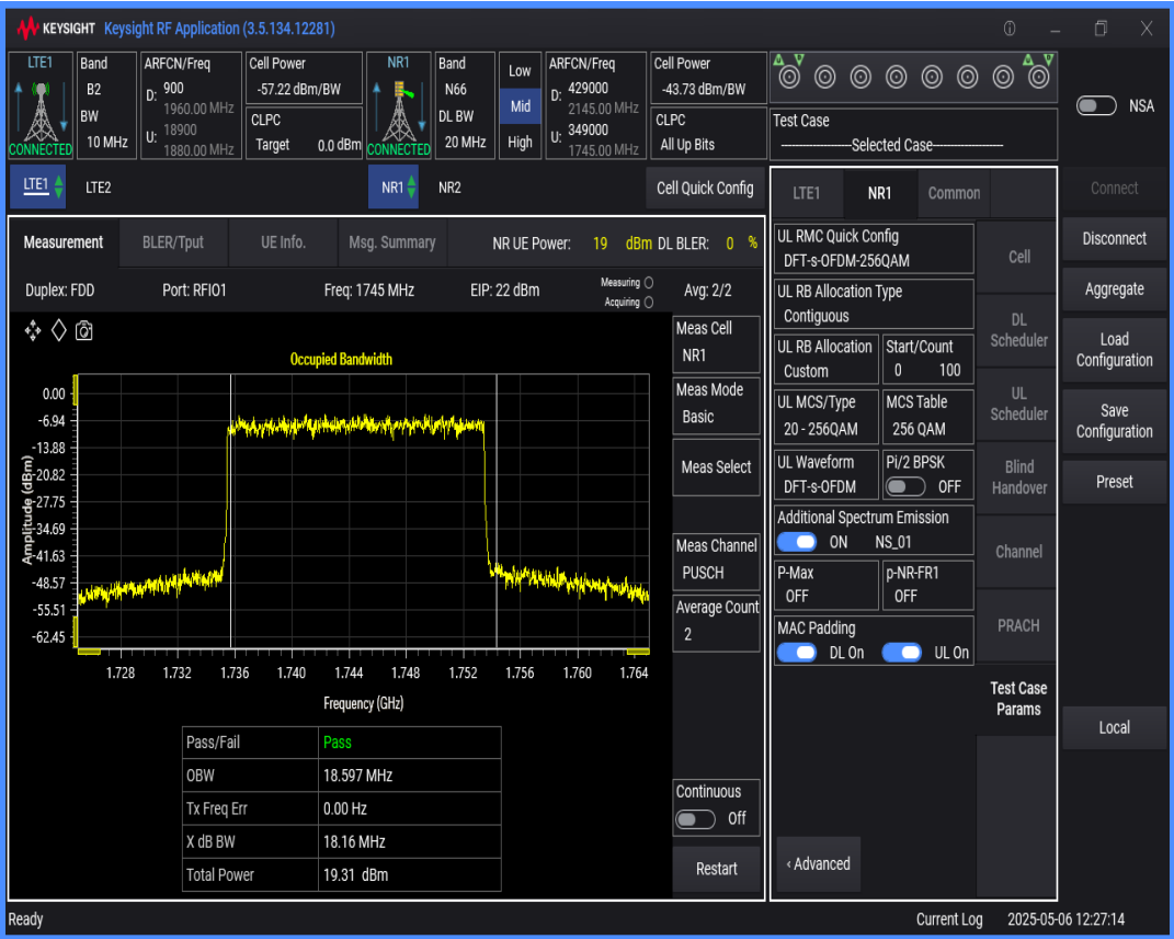
n66 SCS=15kHz DFT_QAM256 BW=15MHz Channel=349000 RB=75@0
