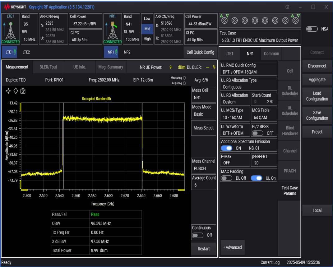
n41 SCS=30kHz DFT_BPSK BW=60MHz Channel=518598 RB=162@0
