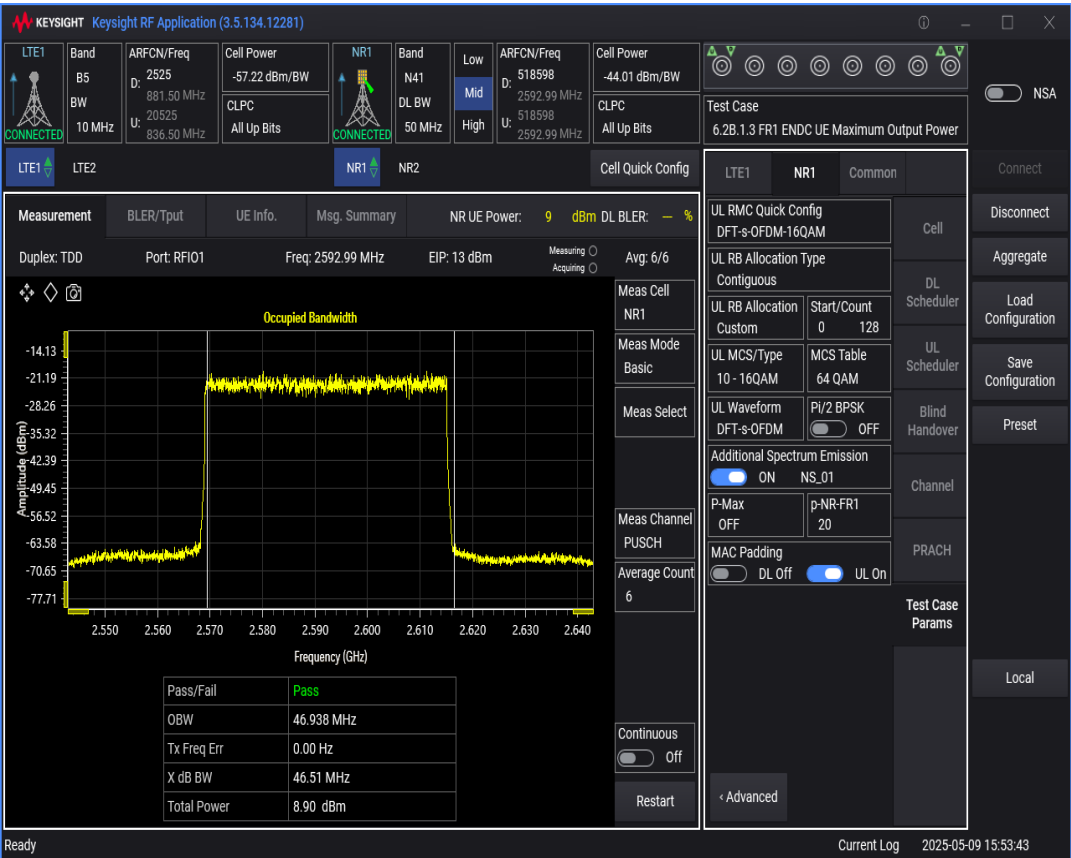
n41 SCS=30kHz DFT_QAM16 BW=40MHz Channel=518598 RB=100@0
