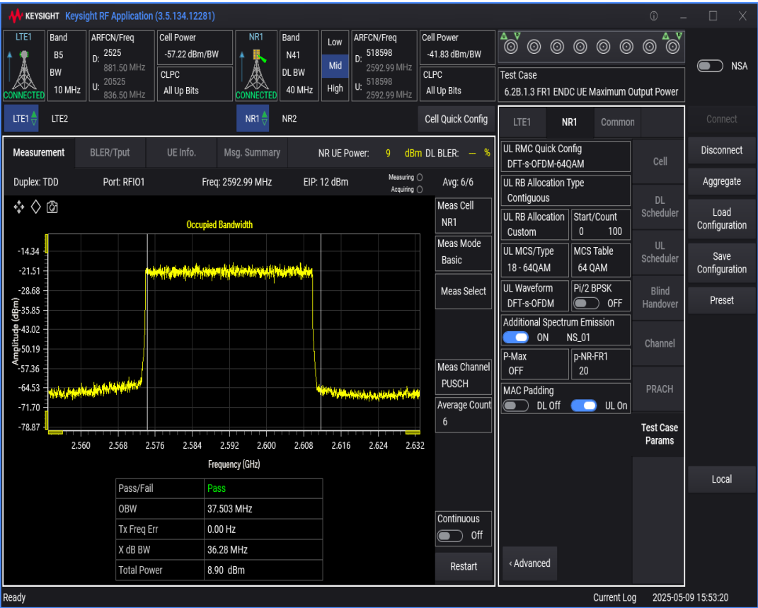
n41 SCS=30kHz DFT_QAM256 BW=90MHz Channel=518598 RB=240@0
