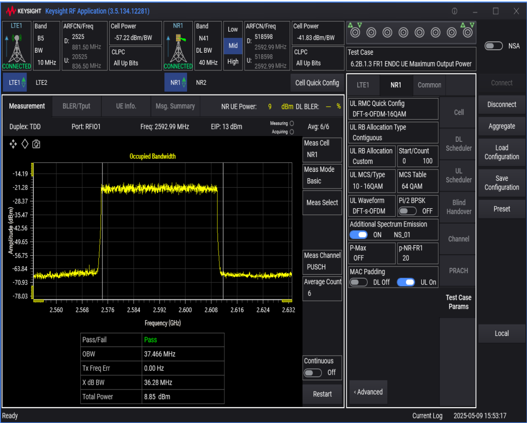
n41 SCS=30kHz DFT_QAM16 BW=60MHz Channel=518598 RB=162@0
