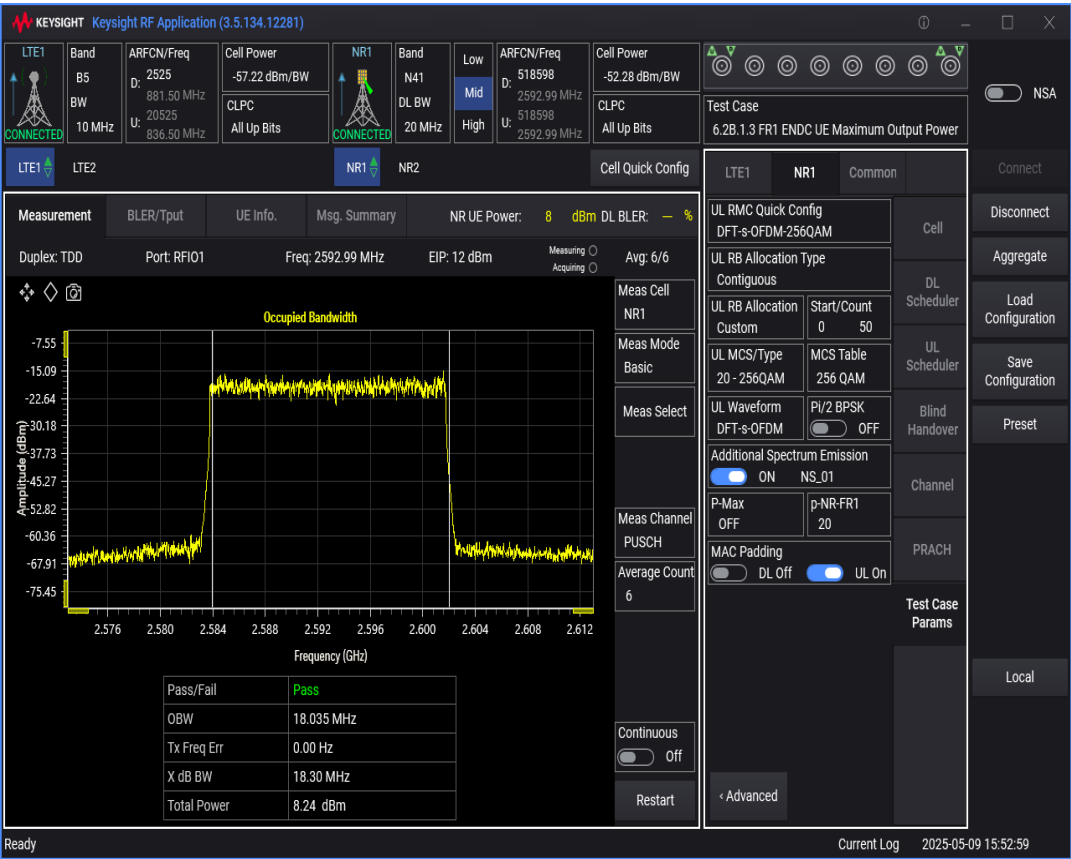
n41 SCS=30kHz DFT_QAM256 BW=100MHz Channel=518598 RB=270@0
