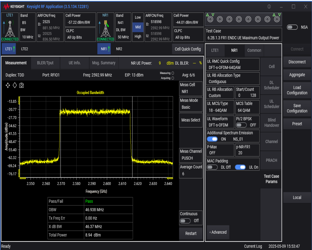
n41 SCS=30kHz DFT_QAM64 BW=90MHz Channel=518598 RB=240@0
