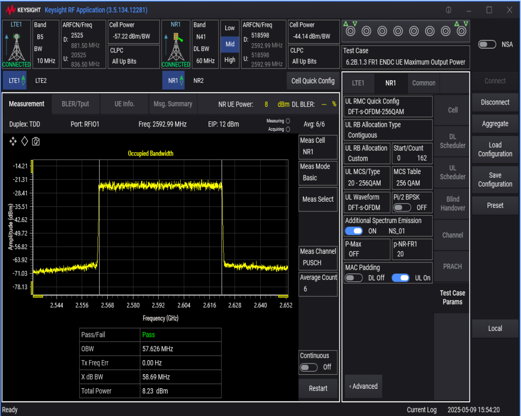
n41 SCS=30kHz DFT_QAM256 BW=50MHz Channel=518598 RB=128@0
