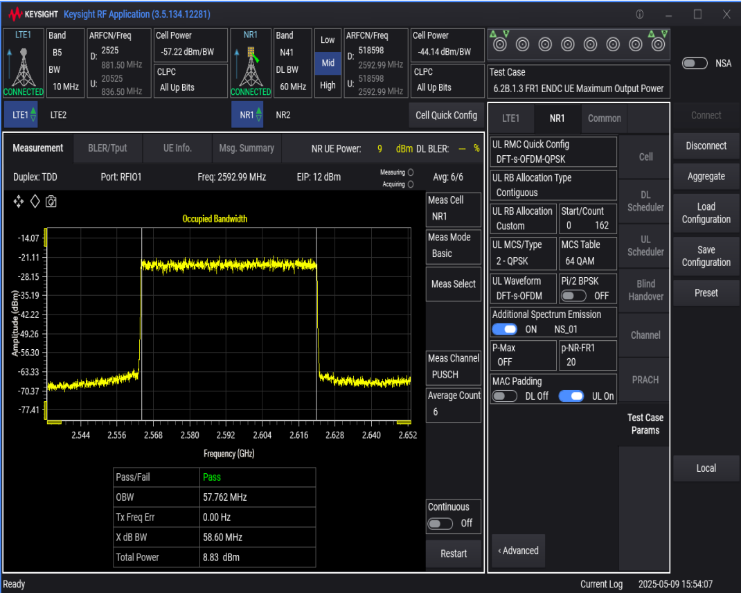
n41 SCS=30kHz DFT_QPSK BW=80MHz Channel=518598 RB=216@0
