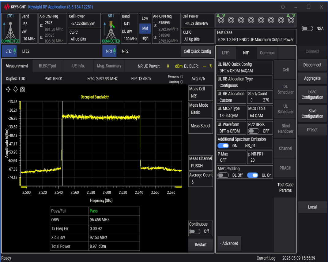
n41 SCS=30kHz DFT_QPSK BW=60MHz Channel=518598 RB=162@0
