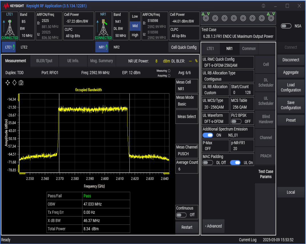
n41 SCS=30kHz DFT_QAM16 BW=50MHz Channel=518598 RB=128@0
