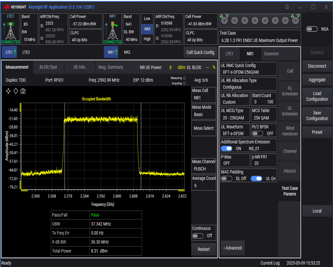
n41 SCS=30kHz DFT_QAM256 BW=60MHz Channel=518598 RB=162@0
