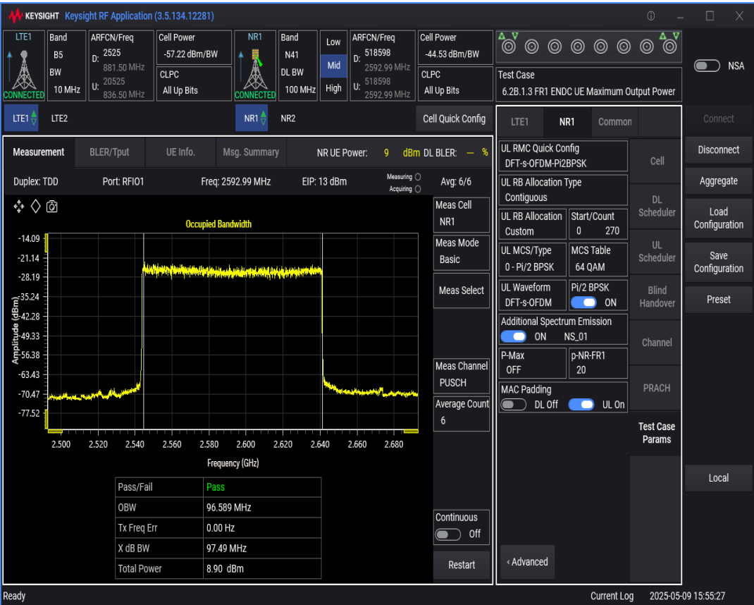
n41 SCS=30kHz DFT_BPSK BW=50MHz Channel=518598 RB=128@0
