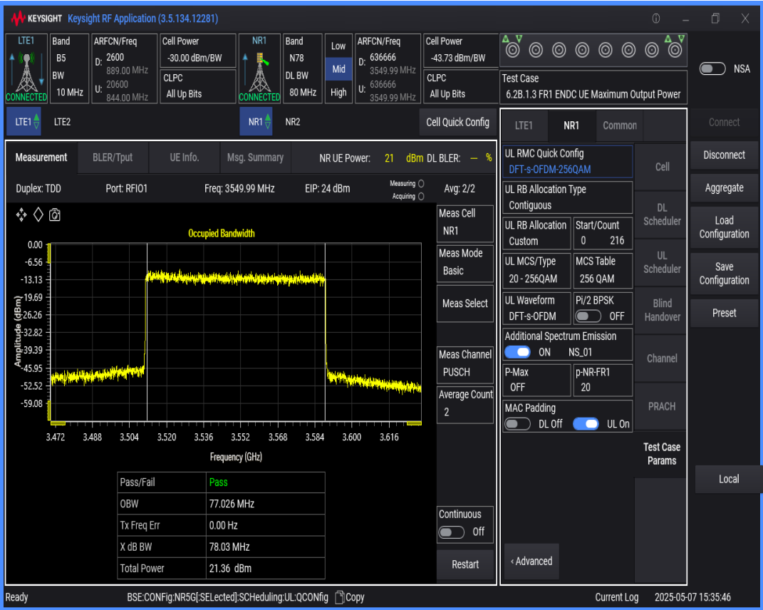
n78 SCS=30kHz DFT_QAM64 BW=100MHz Channel=636666 RB=270@0
