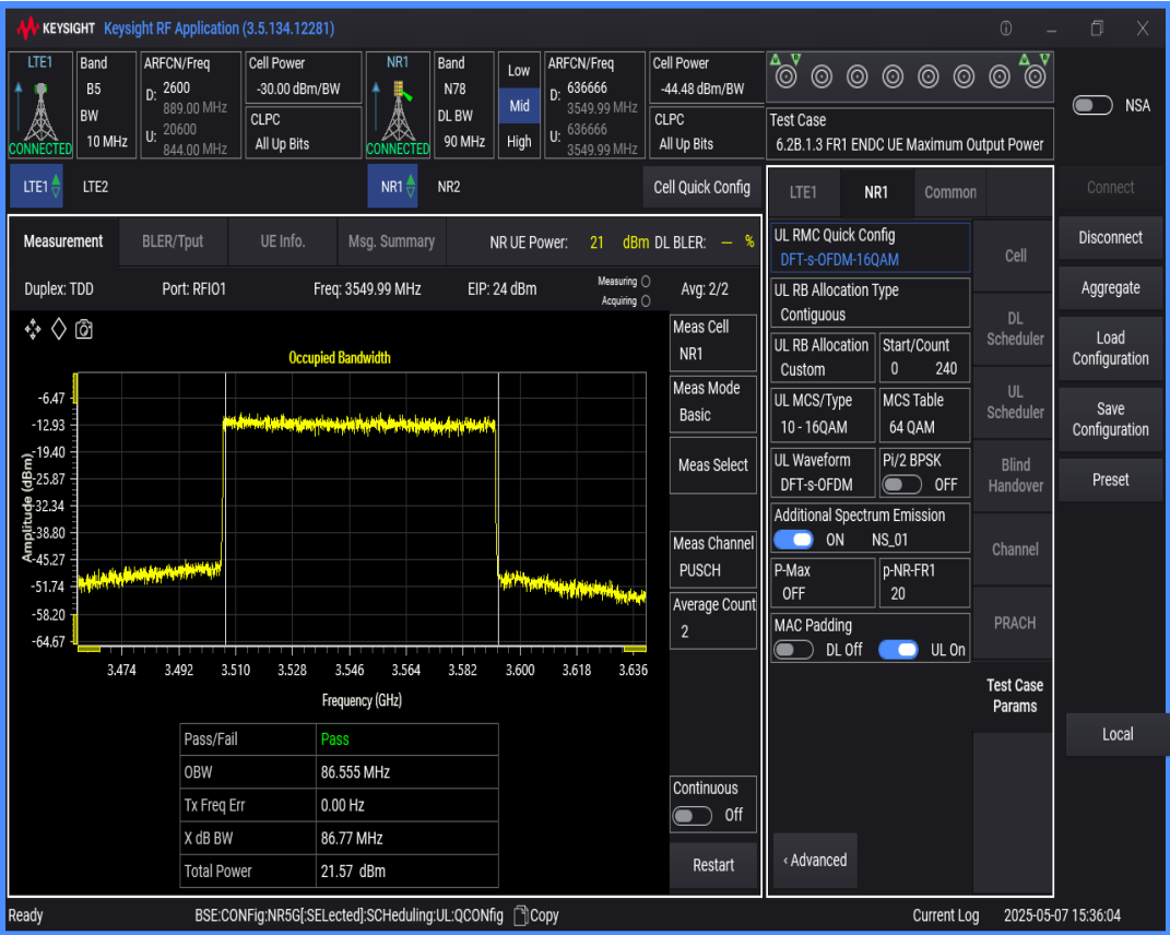
n78 SCS=30kHz DFT_QAM16 BW=80MHz Channel=636666 RB=216@0
