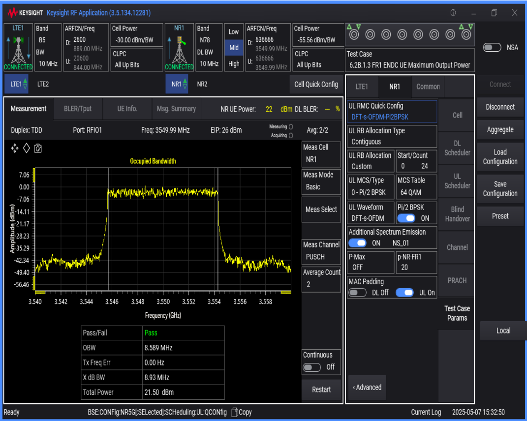
n78 SCS=30kHz DFT_BPSK BW=100MHz Channel=636666 RB=270@0
