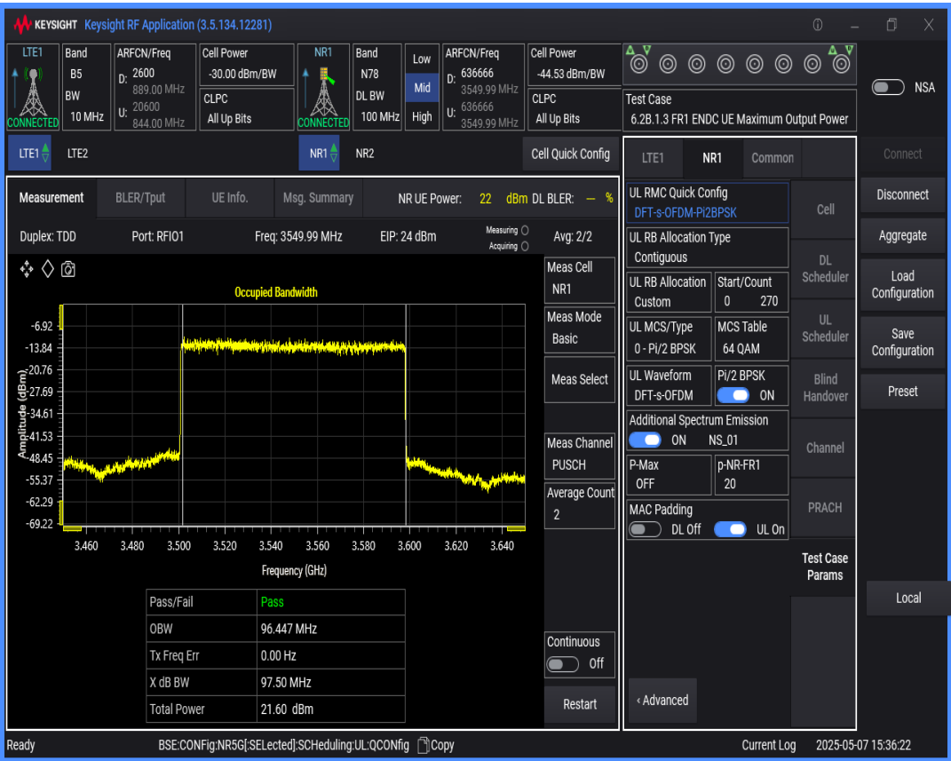
n78 SCS=30kHz DFT_BPSK BW=90MHz Channel=636666 RB=240@0
