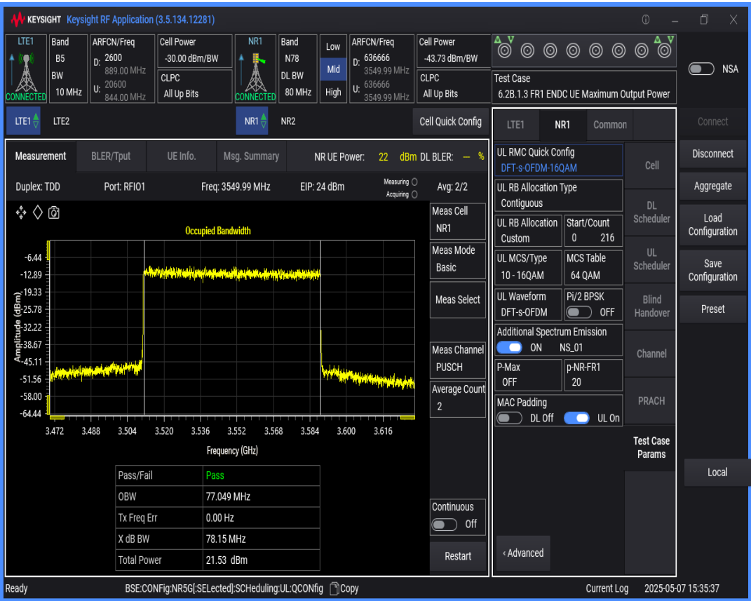
n78 SCS=30kHz DFT_QAM256 BW=10MHz Channel=636666 RB=24@0
