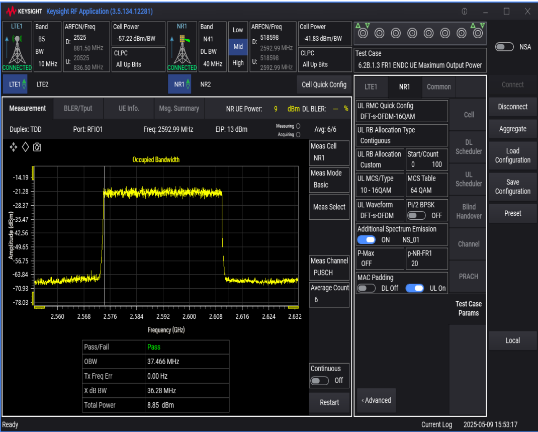
n41 SCS=30kHz DFT_QAM16 BW=50MHz Channel=518598 RB=128@0
