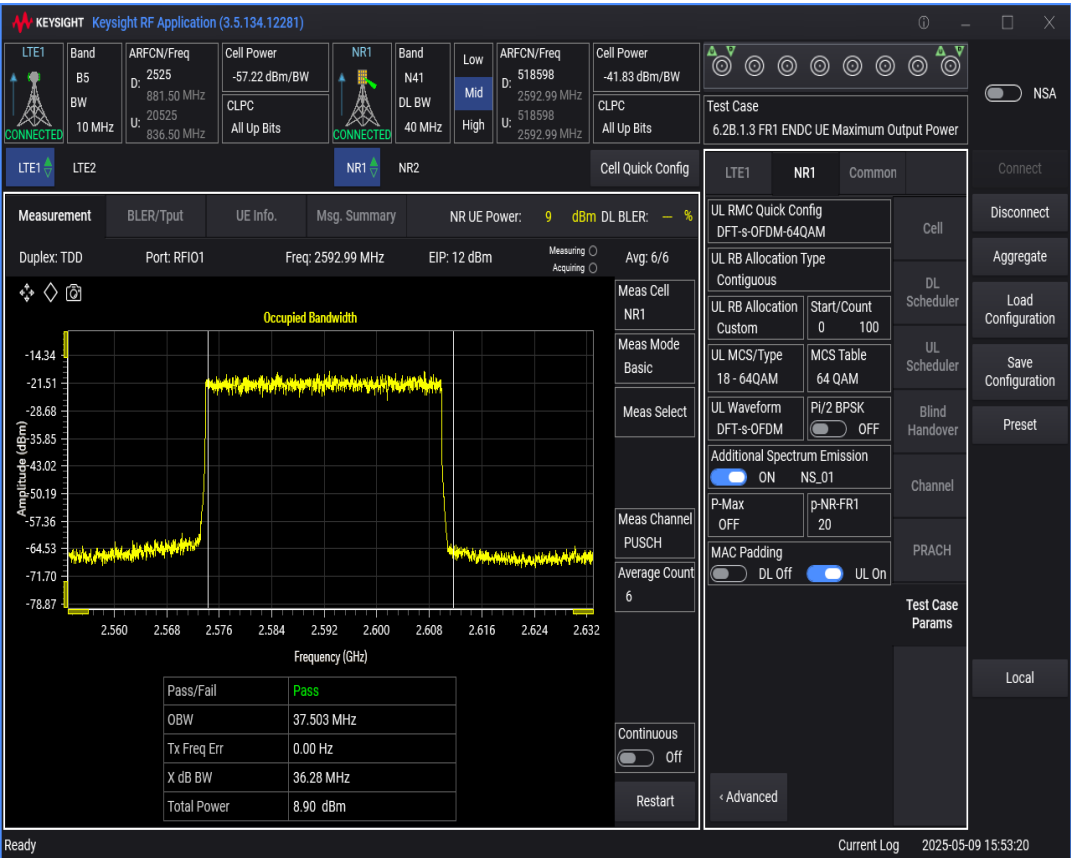
n41 SCS=30kHz DFT_QAM64 BW=50MHz Channel=518598 RB=128@0
