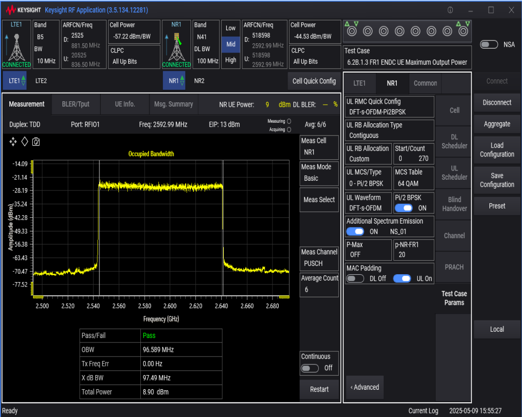
n41 SCS=30kHz DFT_BPSK BW=50MHz Channel=518598 RB=128@0
