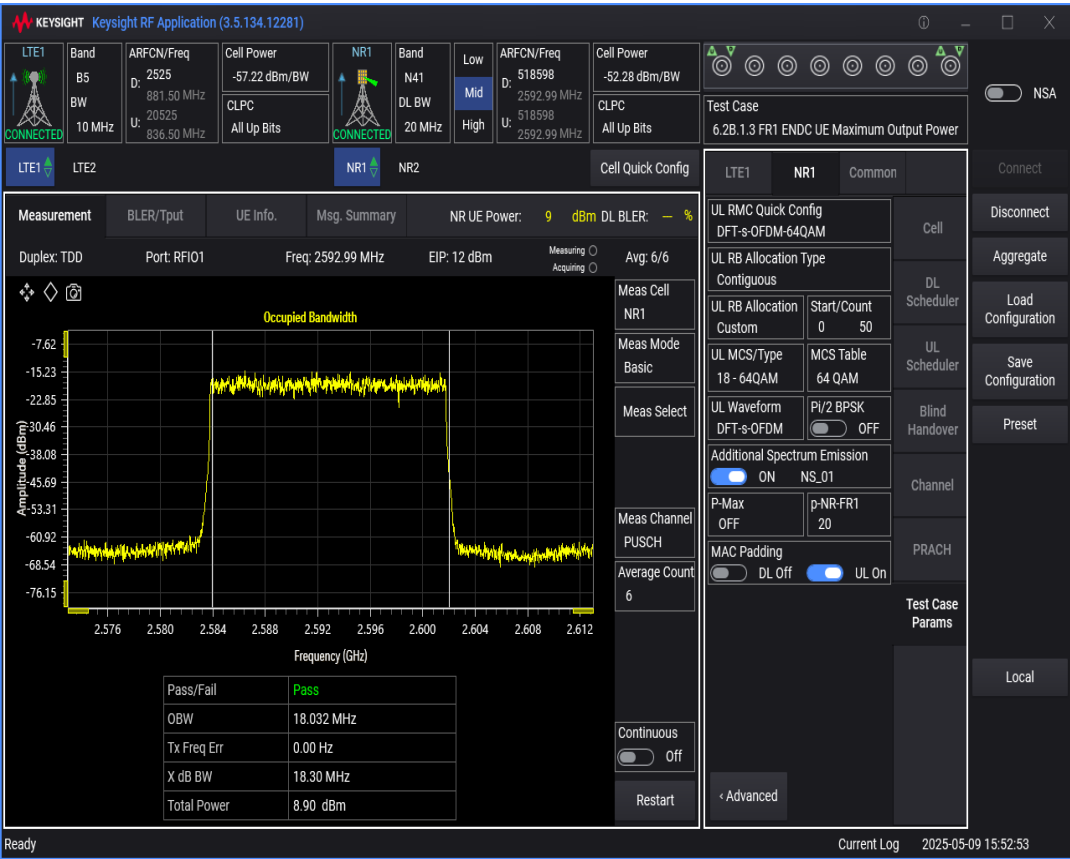
n41 SCS=30kHz DFT_QAM64 BW=40MHz Channel=518598 RB=100@0
