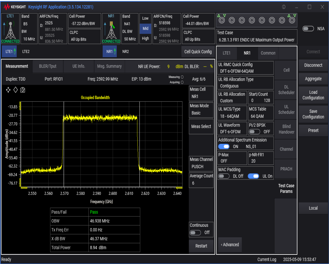
n41 SCS=30kHz DFT_QAM256 BW=80MHz Channel=518598 RB=216@0
