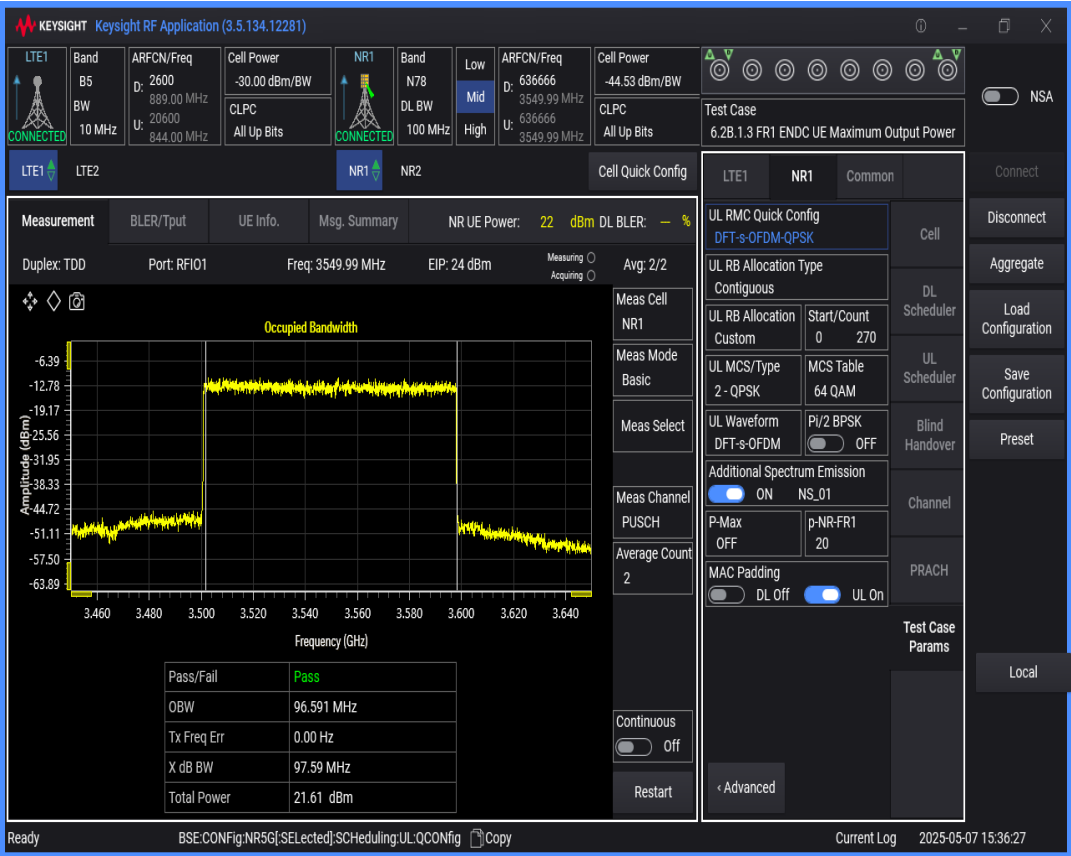
n78 SCS=30kHz DFT_QAM64 BW=90MHz Channel=636666 RB=240@0
