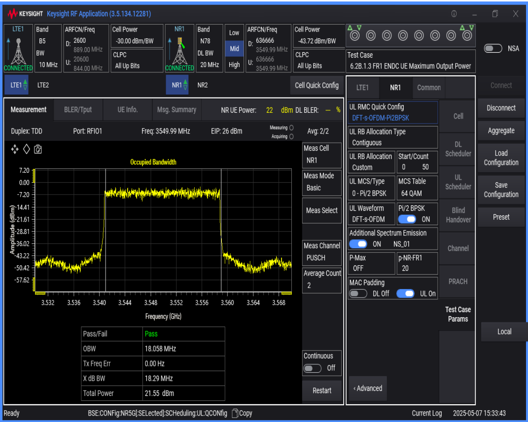
n78 SCS=30kHz DFT_BPSK BW=15MHz Channel=636666 RB=36@0
