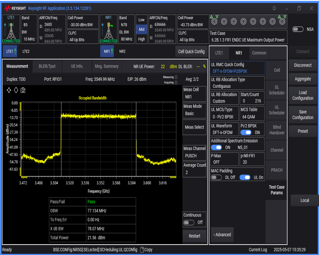
n78 SCS=30kHz DFT_BPSK BW=60MHz Channel=636666 RB=162@0
