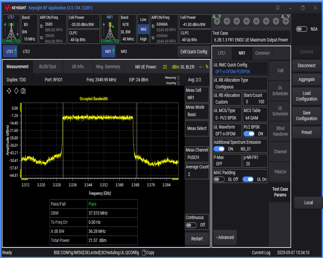
n78 SCS=30kHz DFT_BPSK BW=80MHz Channel=636666 RB=216@0
