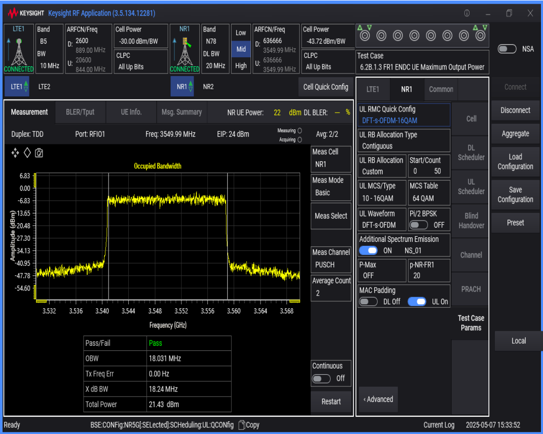
n78 SCS=30kHz DFT_QAM16 BW=60MHz Channel=636666 RB=162@0
