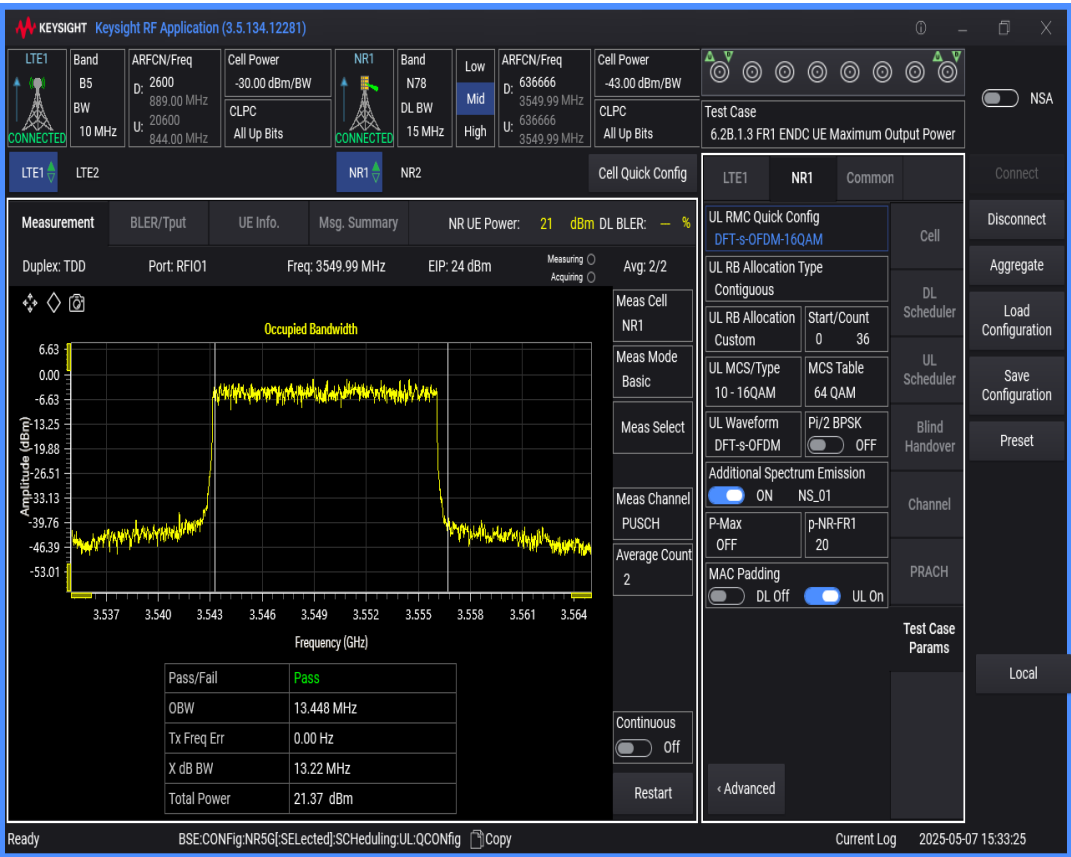
n78 SCS=30kHz DFT_QAM16 BW=10MHz Channel=636666 RB=24@0
