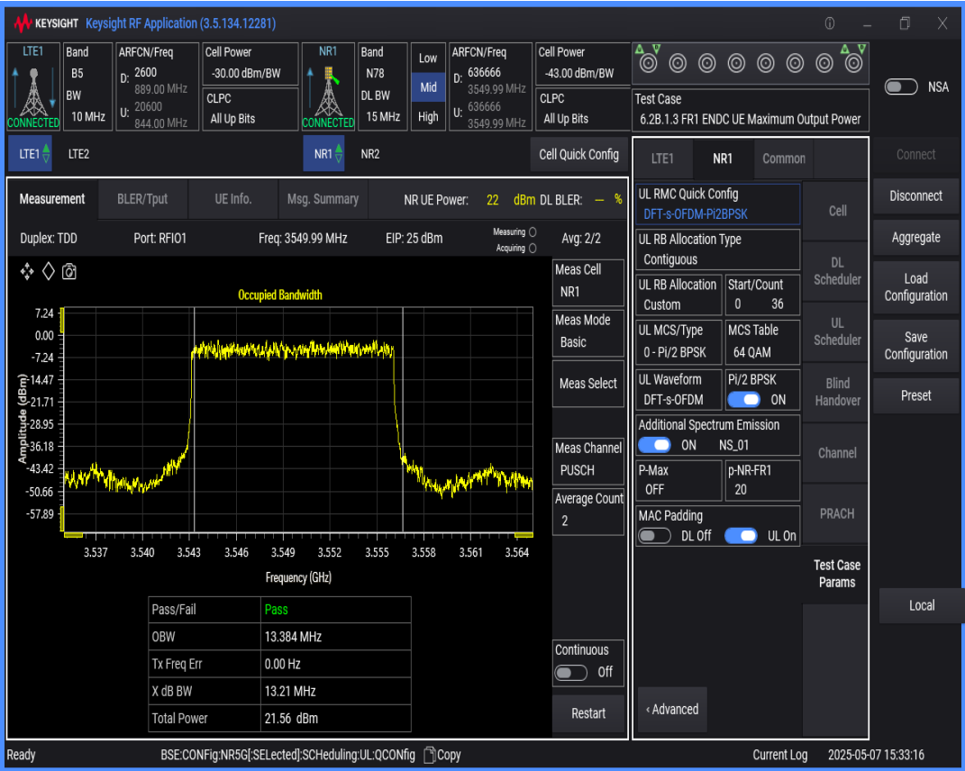
n78 SCS=30kHz DFT_QAM16 BW=40MHz Channel=636666 RB=100@0
