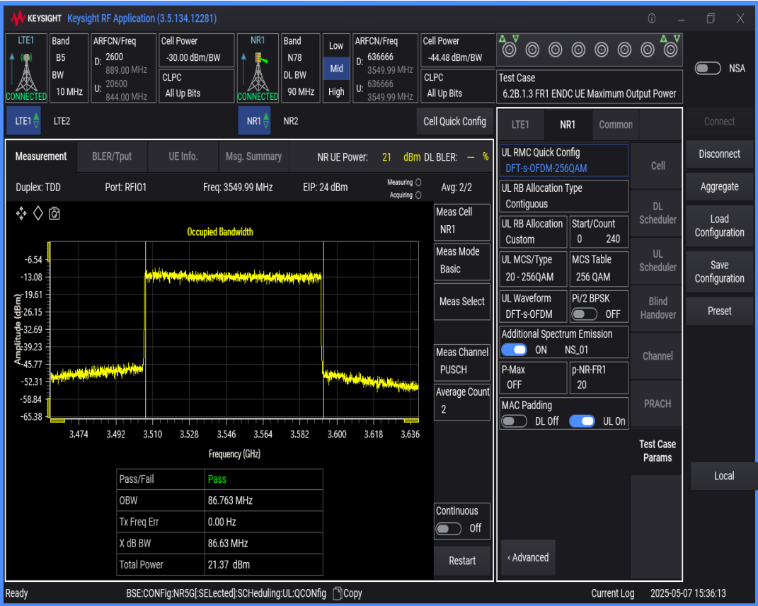
n78 SCS=30kHz DFT_QAM256 BW=80MHz Channel=636666 RB=216@0
