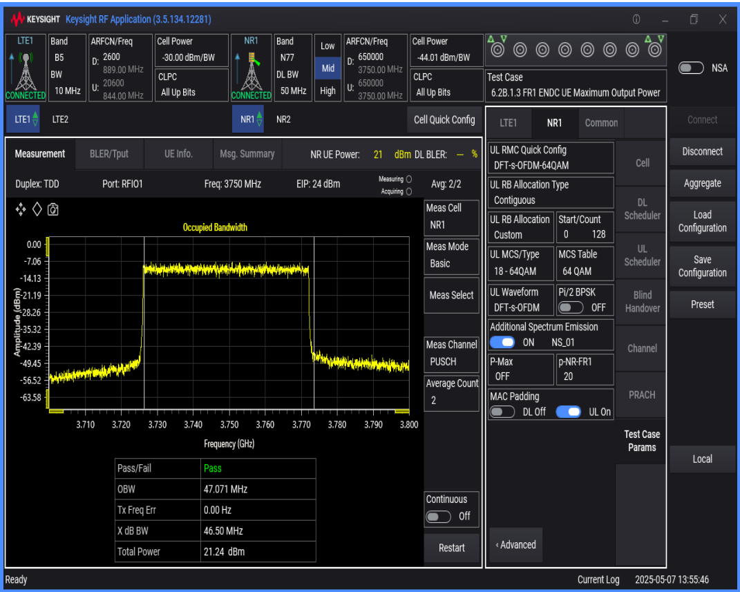
n77 SCS=30kHz DFT_QAM64 BW=60MHz Channel=650000 RB=162@0
