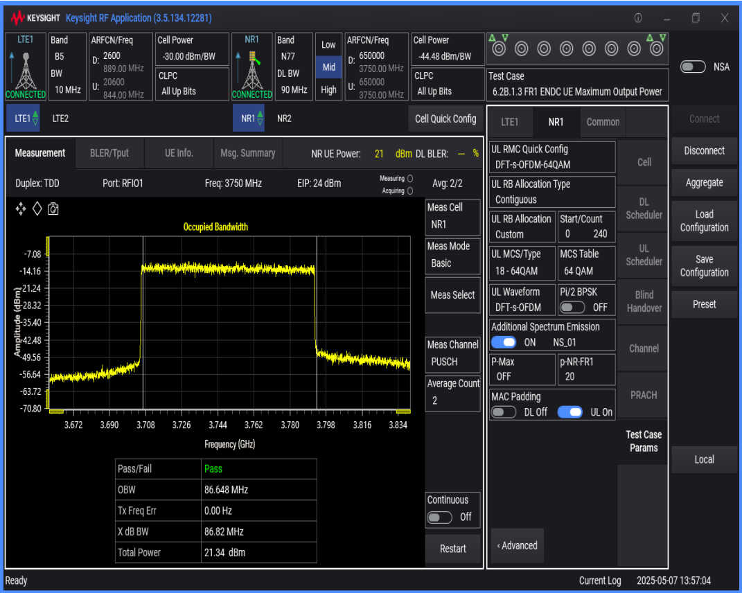
n77 SCS=30kHz DFT_QAM64 BW=50MHz Channel=650000 RB=128@0
