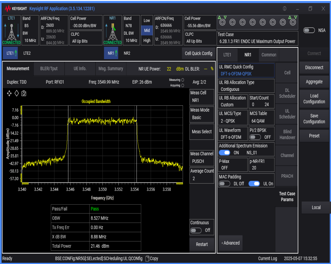
n78 SCS=30kHz DFT_QPSK BW=40MHz Channel=636666 RB=100@0
