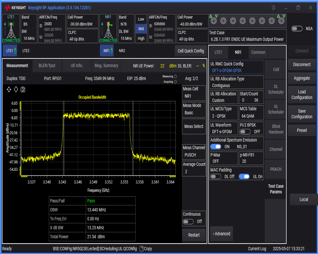
n78 SCS=30kHz DFT_QPSK BW=10MHz Channel=636666 RB=24@0
