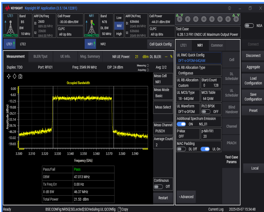
n78 SCS=30kHz DFT_QAM64 BW=60MHz Channel=636666 RB=162 @0
