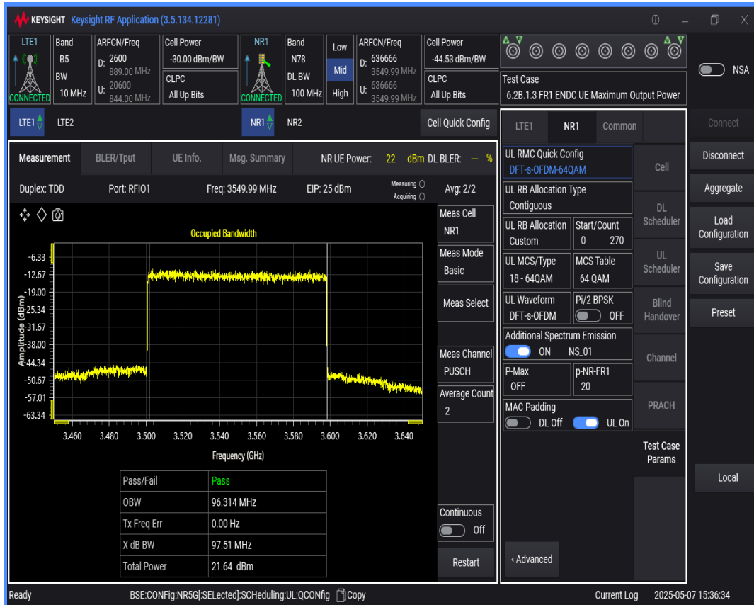
n78 SCS=30kHz DFT_QAM256 BW=90MHz Channel=636666 RB=240@0
