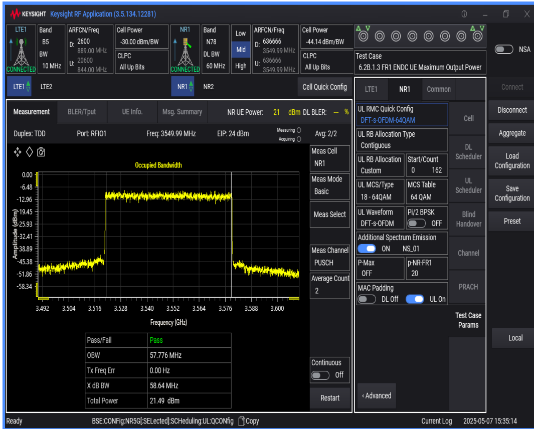
n78 SCS=30kHz DFT_QAM64 BW=90MHz Channel=636666 RB=240@0
