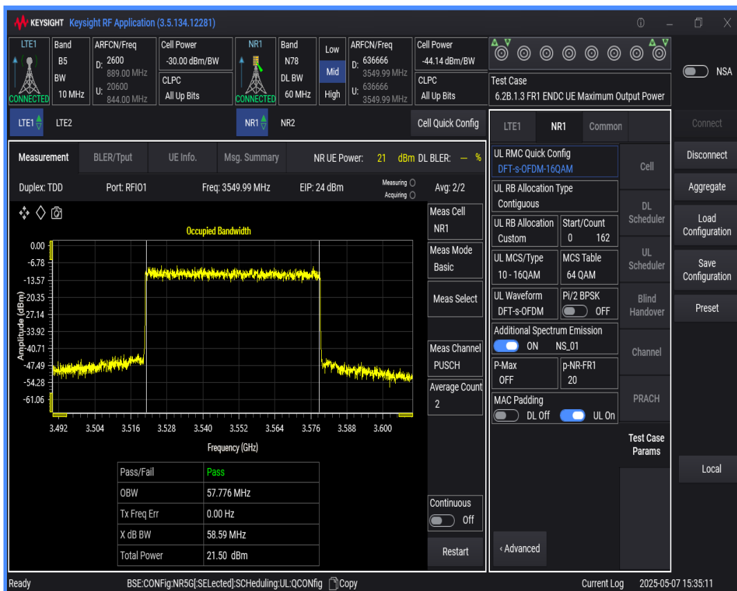
n78 SCS=30kHz DFT_QAM16 BW=90MHz Channel=636666 RB=240 @0
