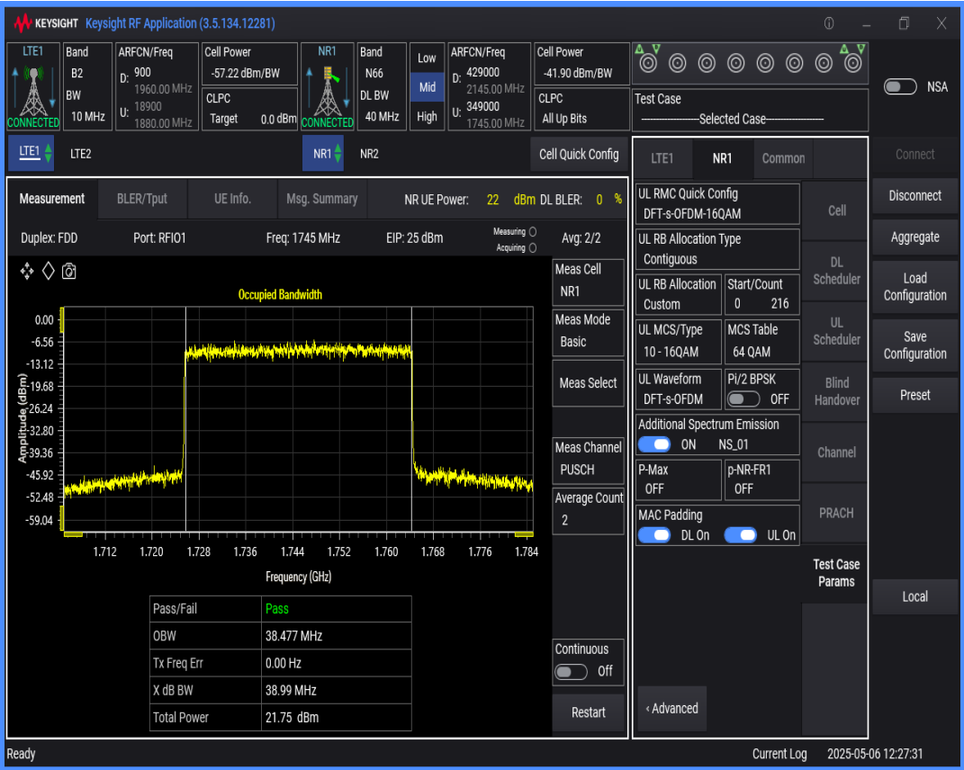
n66 SCS=15kHz DFT_QAM16 BW=20MHz Channel=349000 RB=100@0
