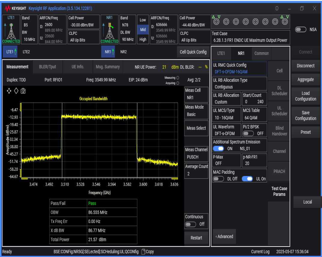
n78 SCS=30kHz DFT_QAM16 BW=80MHz Channel=636666 RB=216@0
