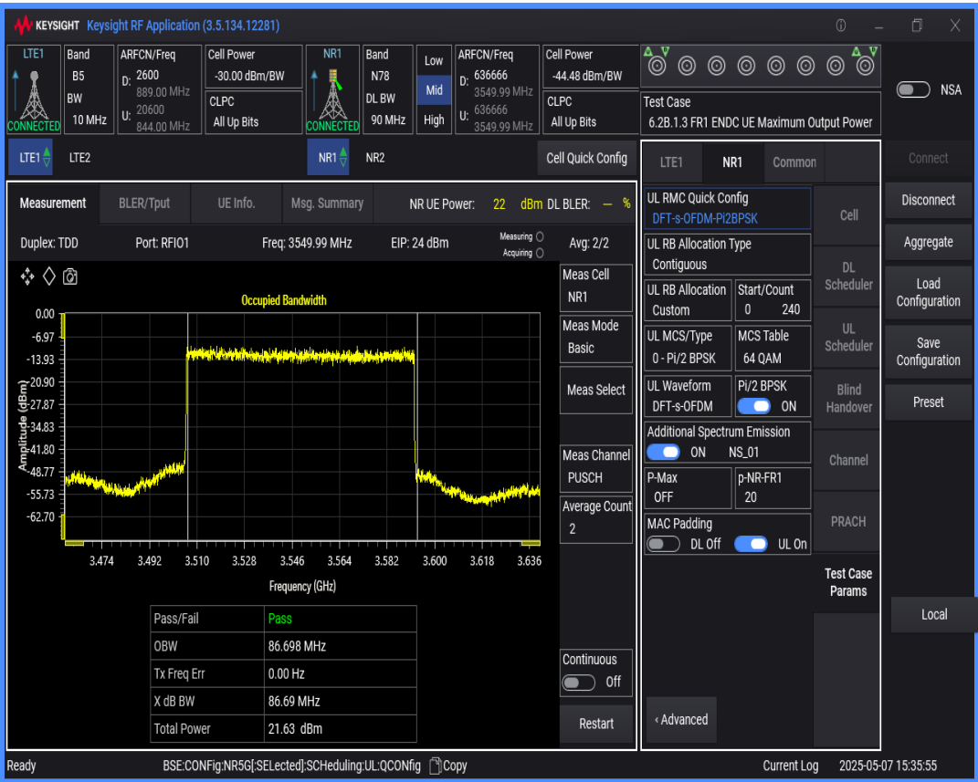
n78 SCS=30kHz DFT_BPSK BW=80MHz Channel=636666 RB=216@0
