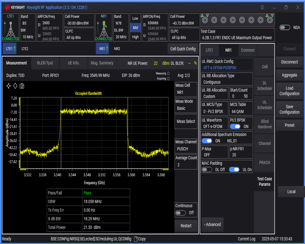
n78 SCS=30kHz DFT_BPSK BW=15MHz Channel=636666 RB=36@0
