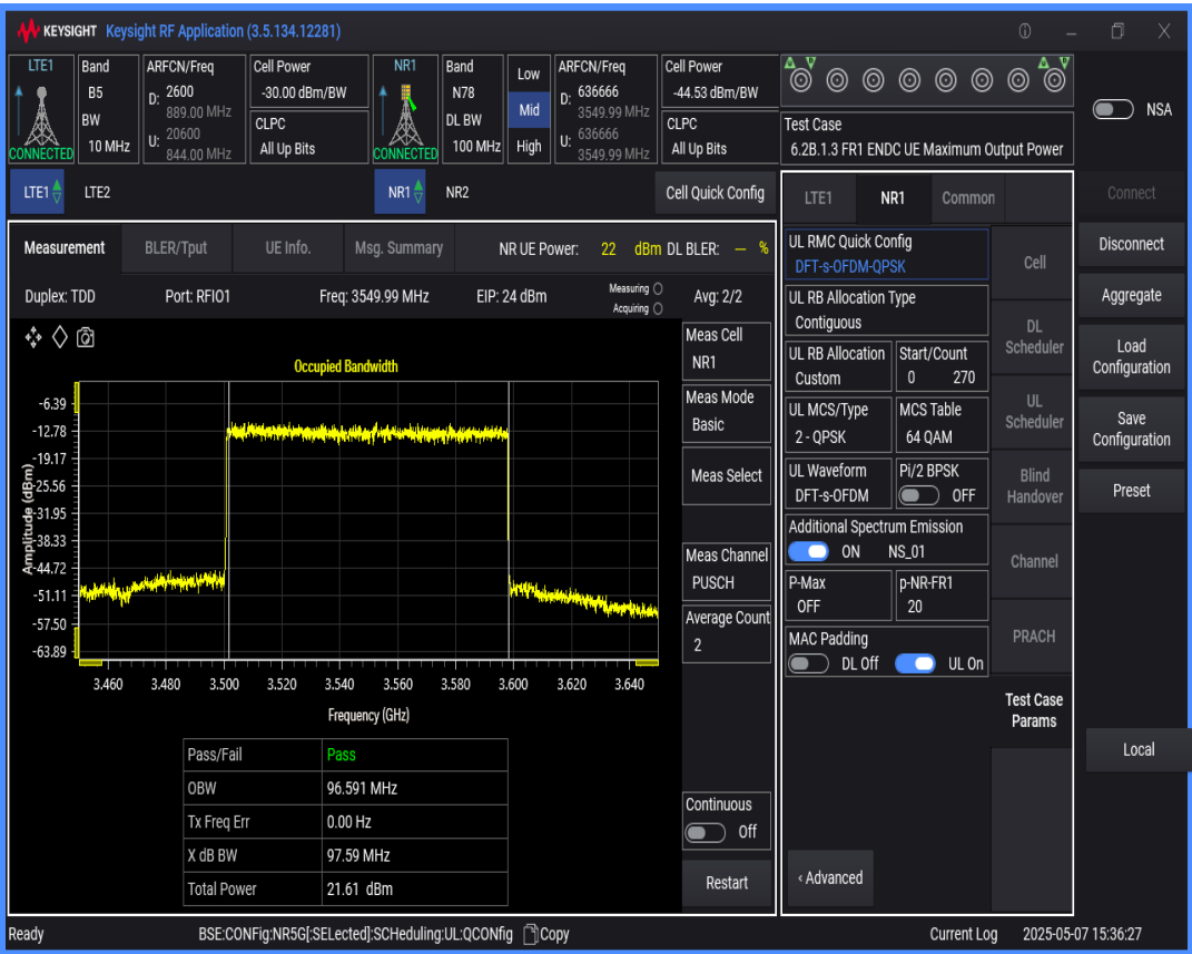
n78 SCS=30kHz DFT_QAM64 BW=60MHz Channel=636666 RB=162@0
