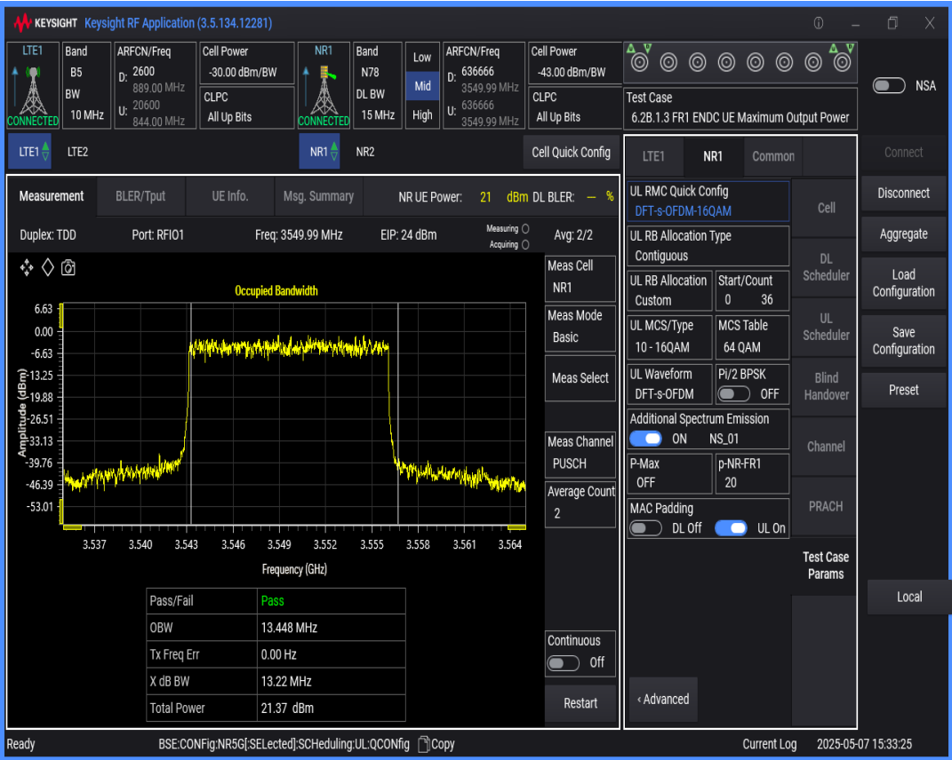
n78 SCS=30kHz DFT_QAM16 BW=10MHz Channel=636666 RB=24@0
