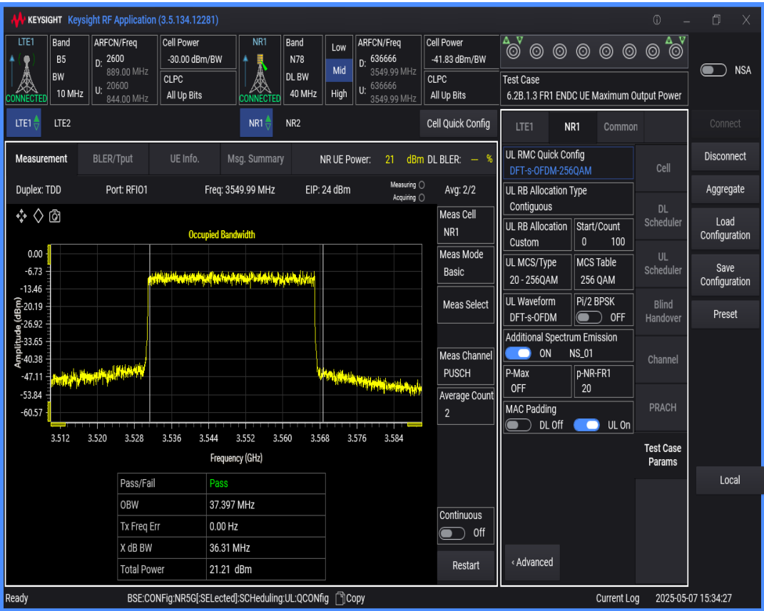
n78 SCS=30kHz DFT_QAM64 BW=90MHz Channel=636666 RB=240@0
