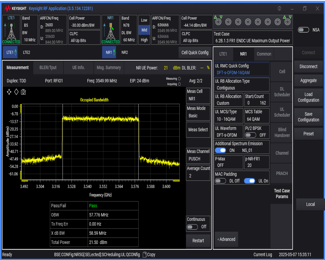
n78 SCS=30kHz DFT_QAM16 BW=50MHz Channel=636666 RB=128@0
