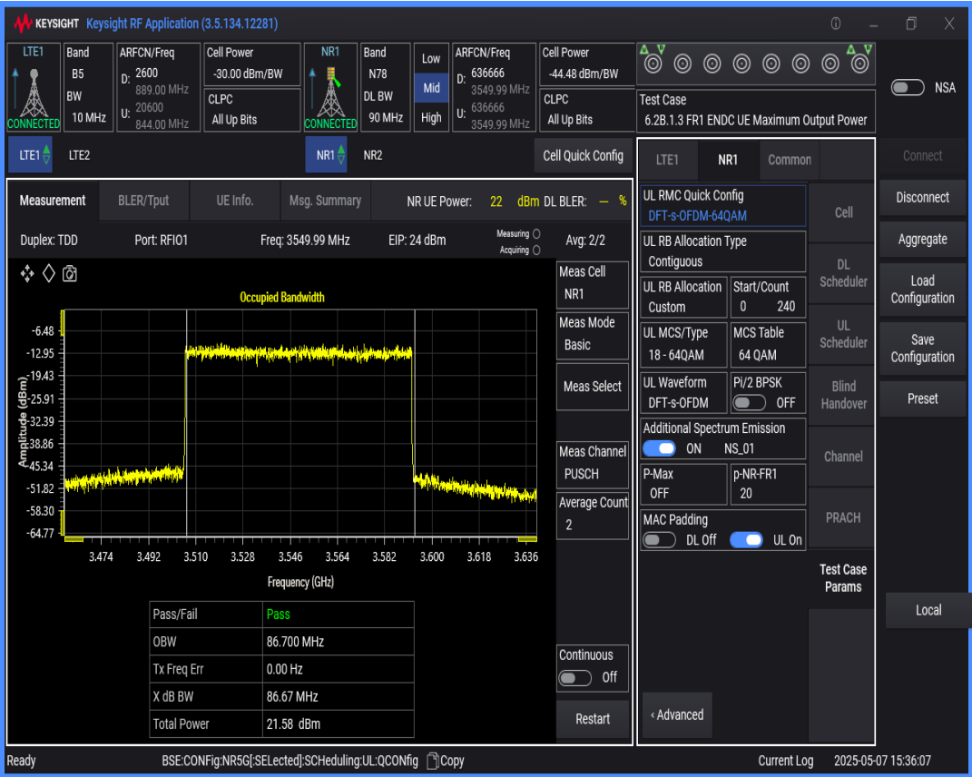
n78 SCS=30kHz DFT_QAM64 BW=80MHz Channel=636666 RB=216@0
