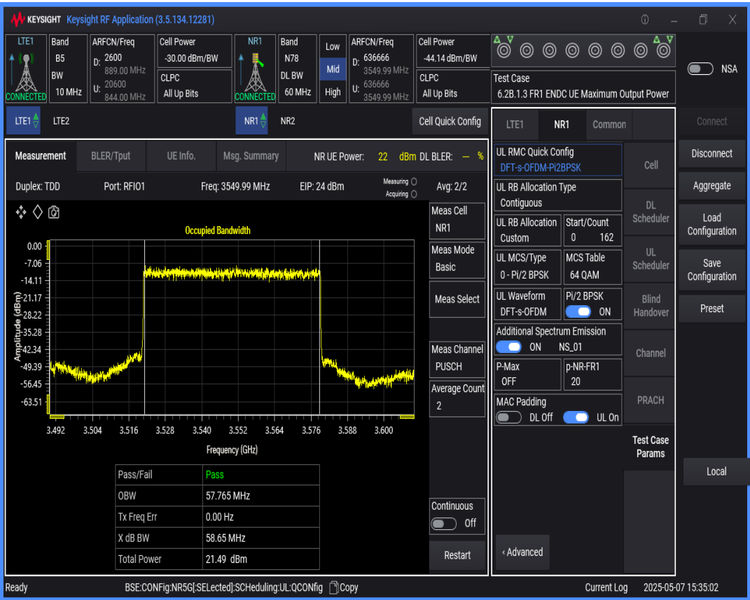
n78 SCS=30kHz DFT_BPSK BW=50MHz Channel=636666 RB=128@0
