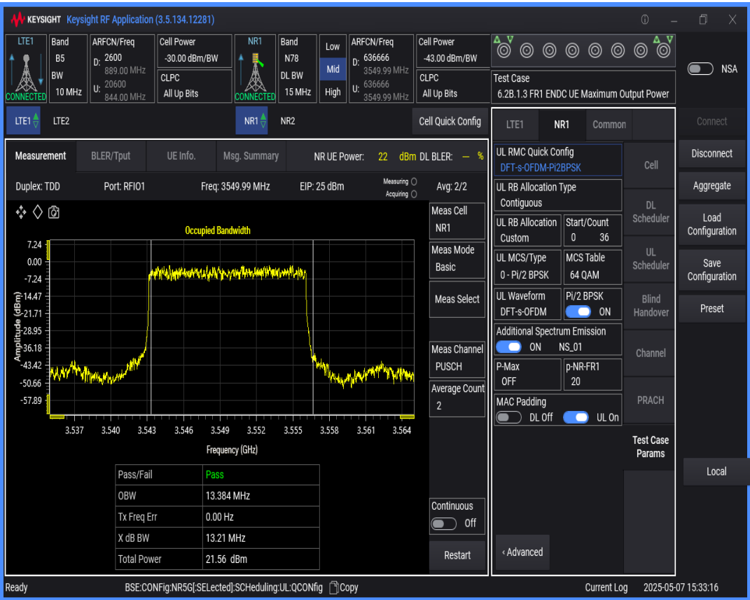
n78 SCS=30kHz DFT_BPSK BW=40MHz Channel=636666 RB=100@0
