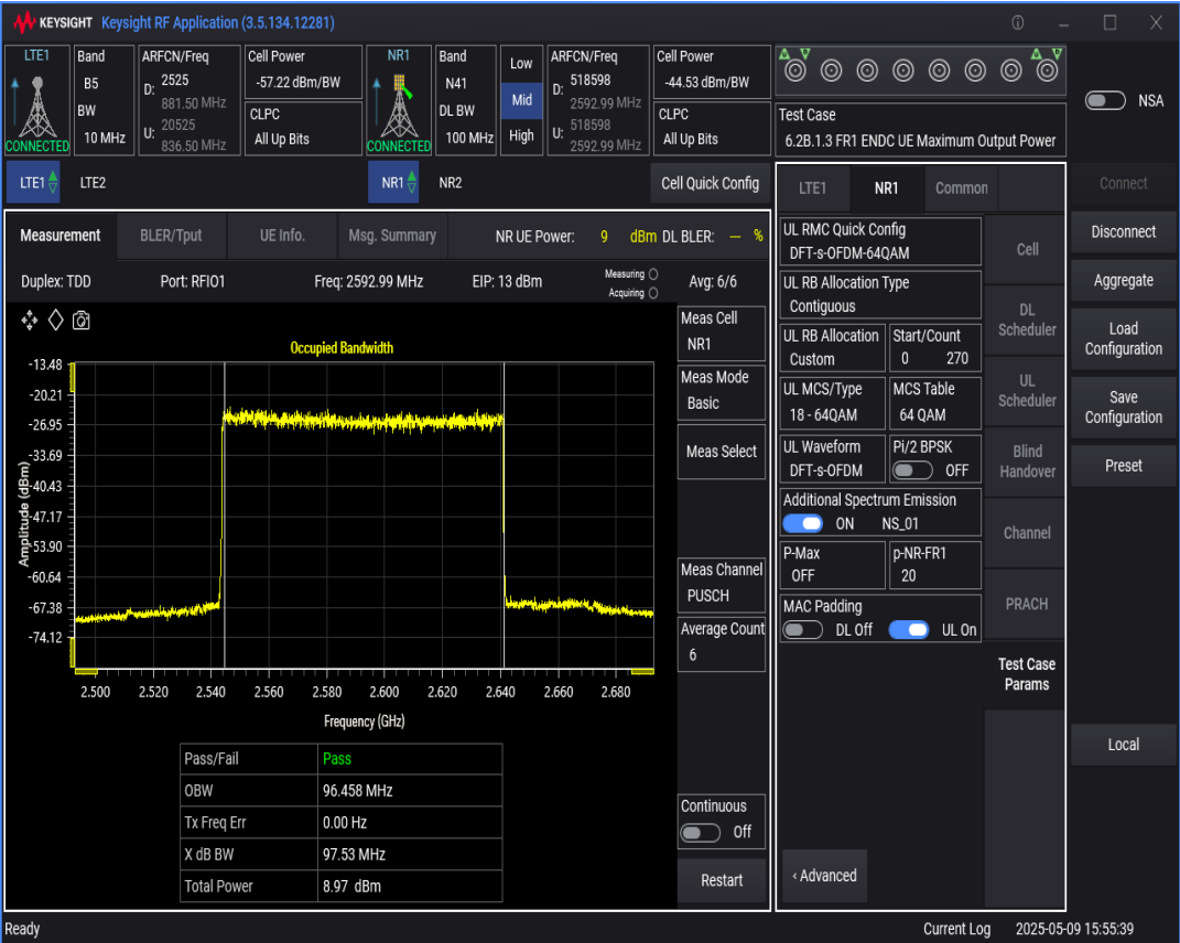
n41 SCS=30kHz DFT_QAM256 BW=90MHz Channel=518598 RB=240@0
