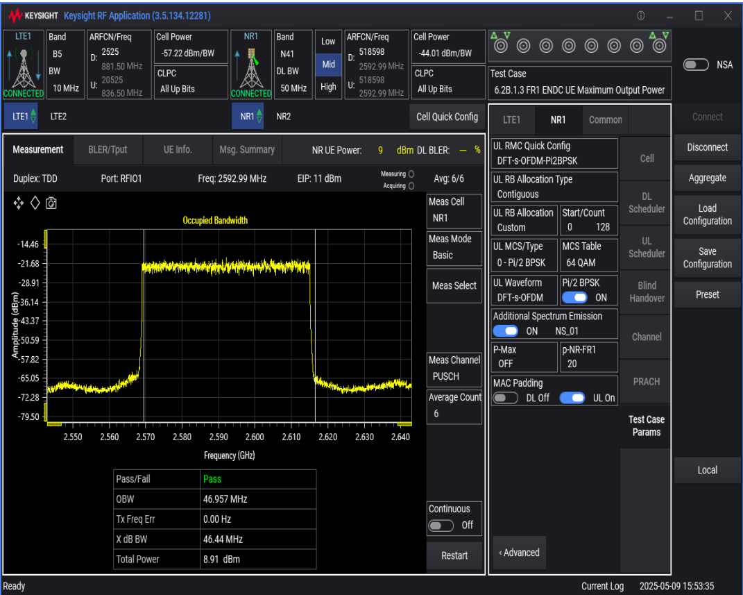
n41 SCS=30kHz DFT_BPSK BW=60MHz Channel=518598 RB=162@0
