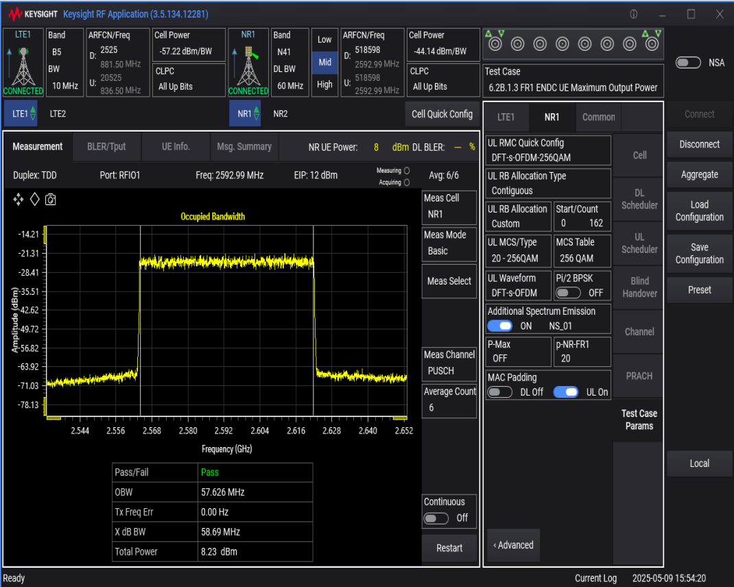
n41 SCS=30kHz DFT_QAM256 BW=80MHz Channel=518598 RB=216@0
