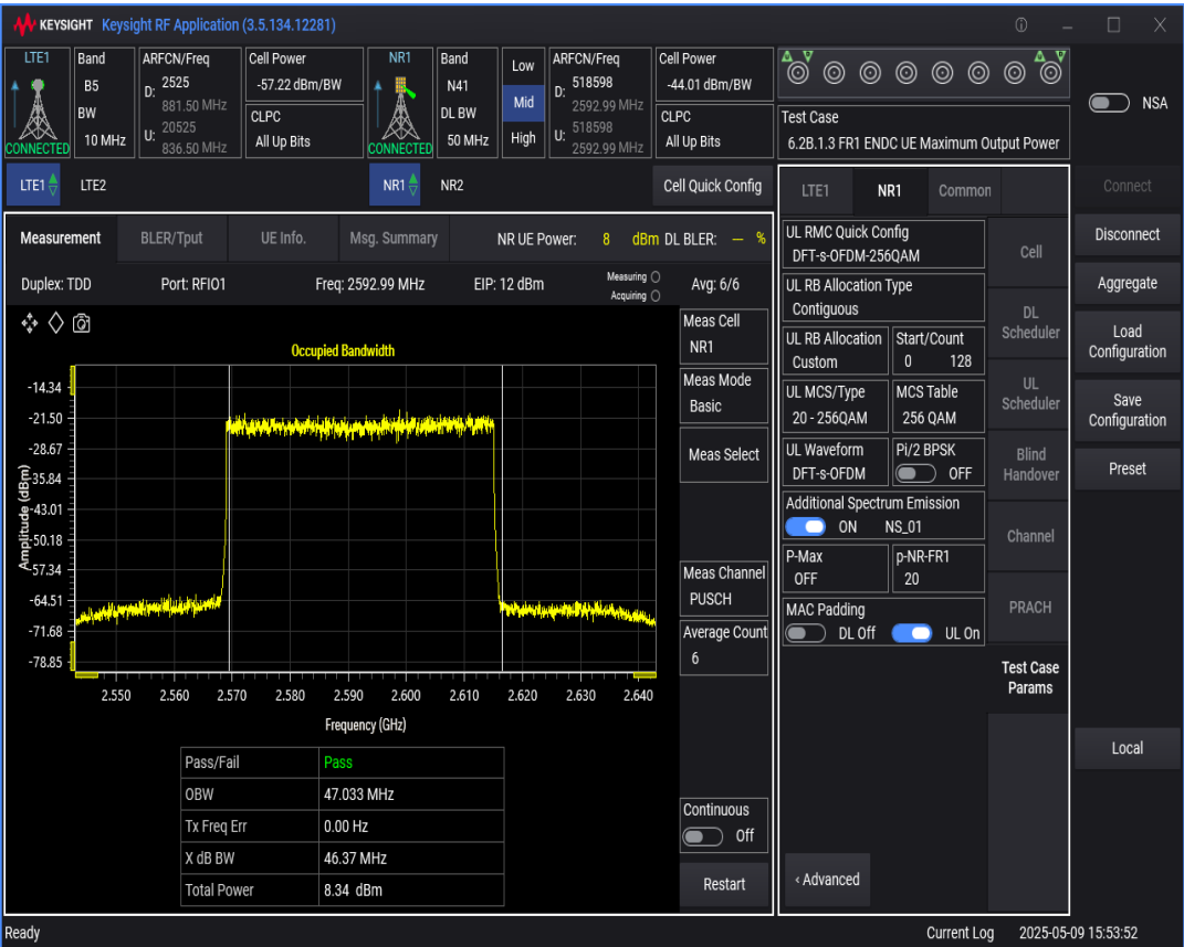
n41 SCS=30kHz DFT_QAM256 BW=60MHz Channel=518598 RB=162@0
