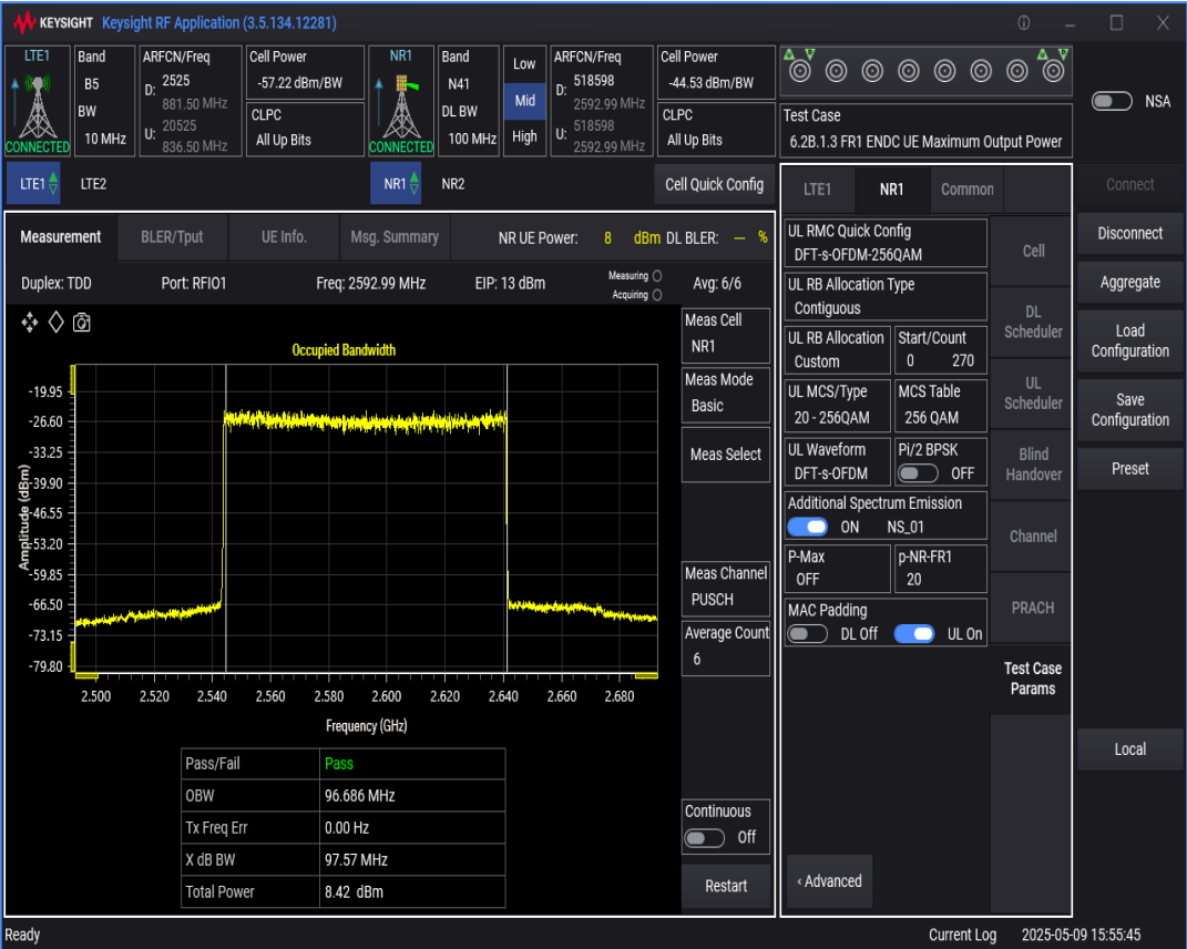
n41 SCS=30kHz DFT_QAM256 BW=50MHz Channel=518598 RB=128@0
