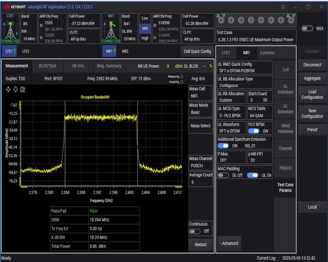
n41 SCS=30kHz DFT_BPSK BW=50MHz Channel=518598 RB=128@0
