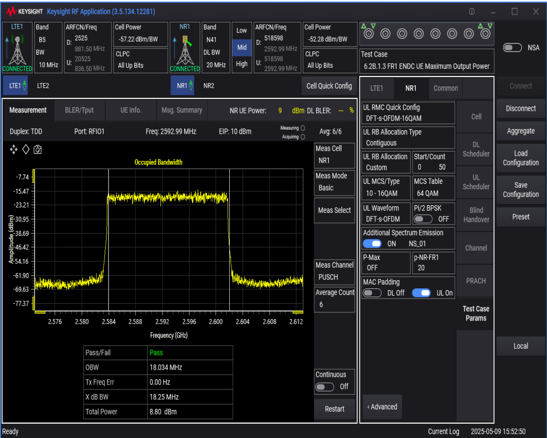
n41 SCS=30kHz DFT_QAM16 BW=40MHz Channel=518598 RB=100@0
