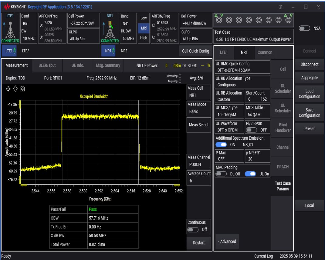
n41 SCS=30kHz DFT_QAM16 BW=50MHz Channel=518598 RB=128@0
