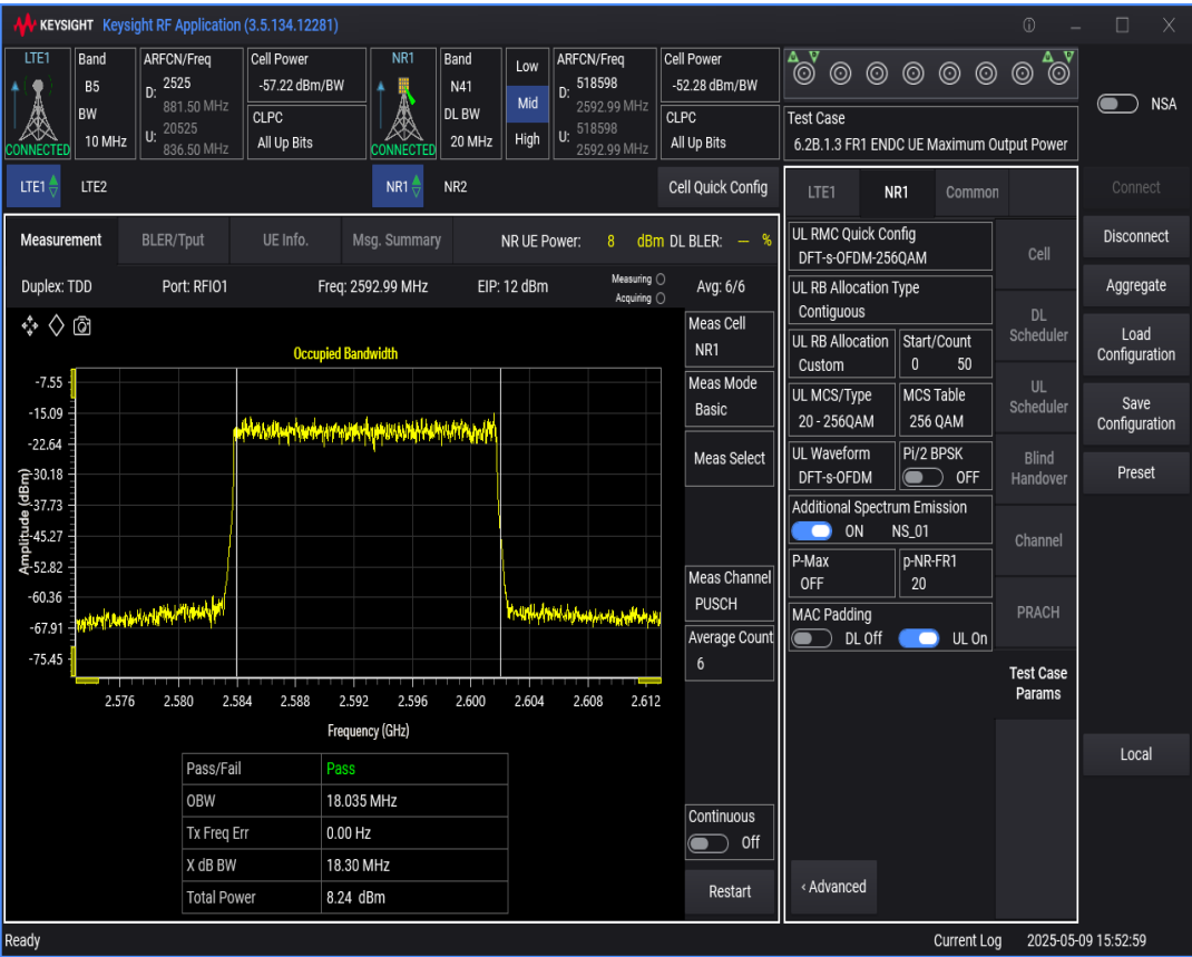
n41 SCS=30kHz DFT_QAM256 BW=100MHz Channel=518598 RB=270@0
