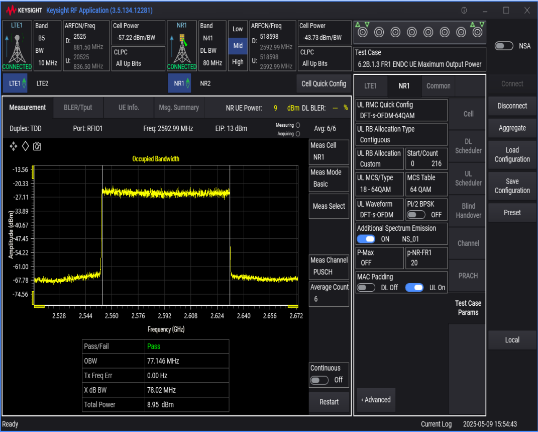
n41 SCS=30kHz DFT_QAM64 BW=90MHz Channel=518598 RB=240@0
