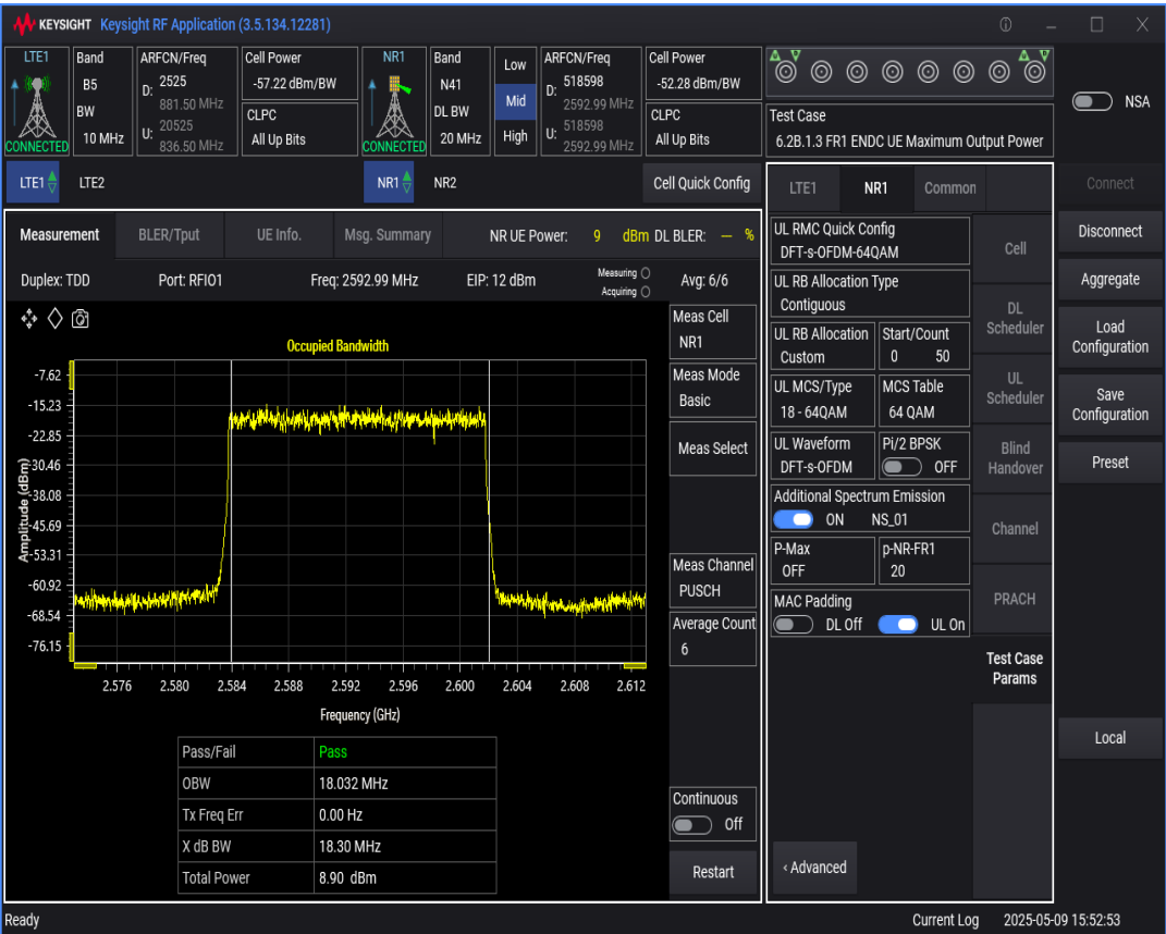
n41 SCS=30kHz DFT_QAM64 BW=40MHz Channel=518598 RB=100@0
