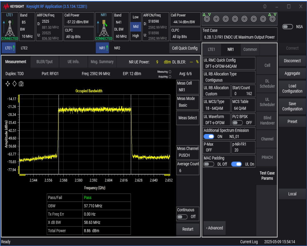
n41 SCS=30kHz DFT_QAM64 BW=80MHz Channel=518598 RB=216@0
