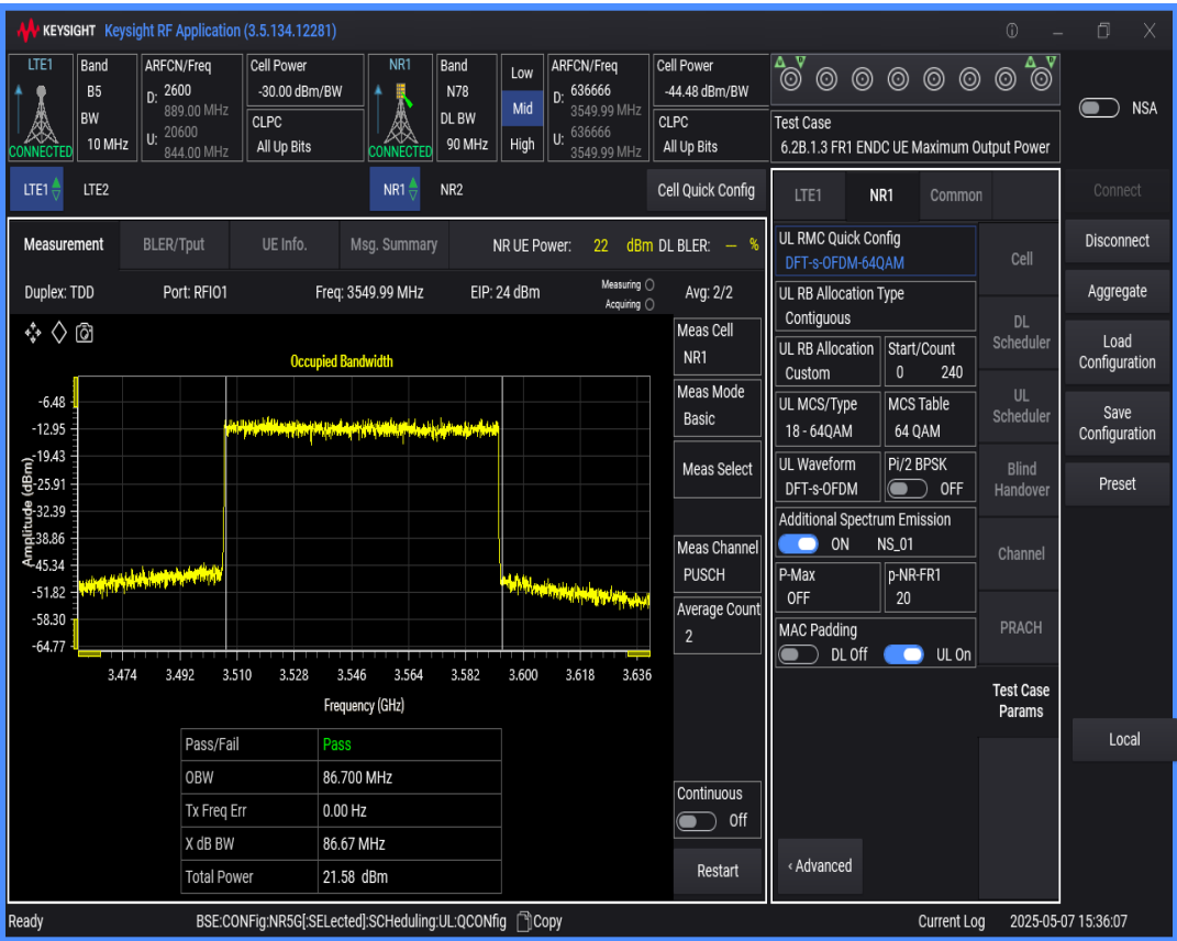
n78 SCS=30kHz DFT_QPSK BW=10MHz Channel=636666 RB=24@0
