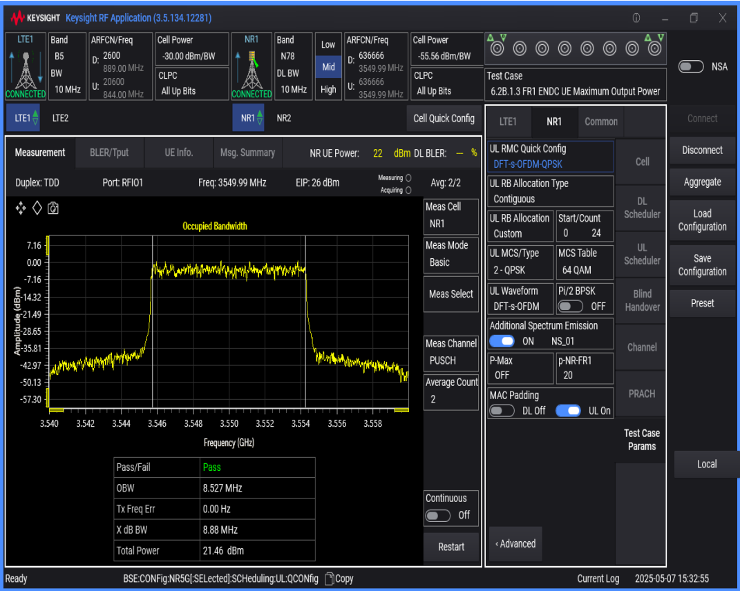
n78 SCS=30kHz DFT_QPSK BW=40MHz Channel=636666 RB=100@0
