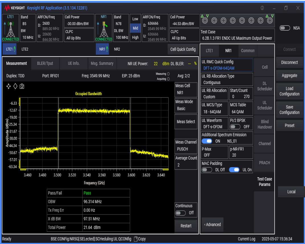
n78 SCS=30kHz DFT_QAM256 BW=90MHz Channel=636666 RB=240@0
