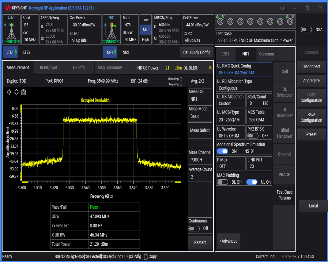
n78 SCS=30kHz DFT_QAM256 BW=40MHz Channel=636666 RB=100@0
