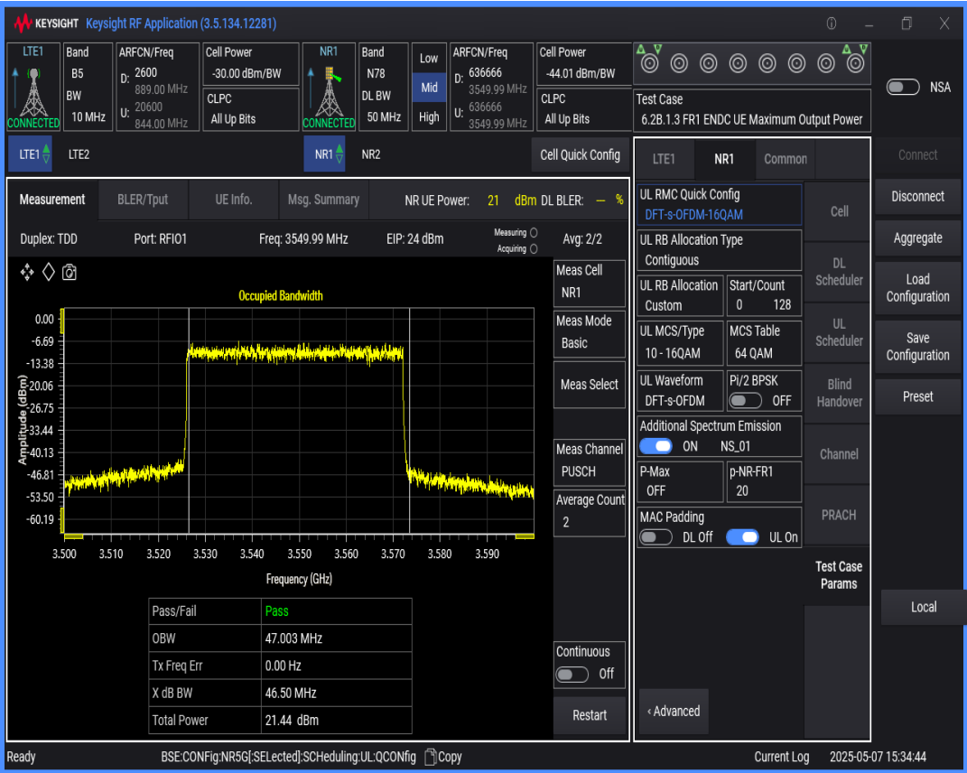
n78 SCS=30kHz DFT_QAM16 BW=80MHz Channel=636666 RB=216@0
