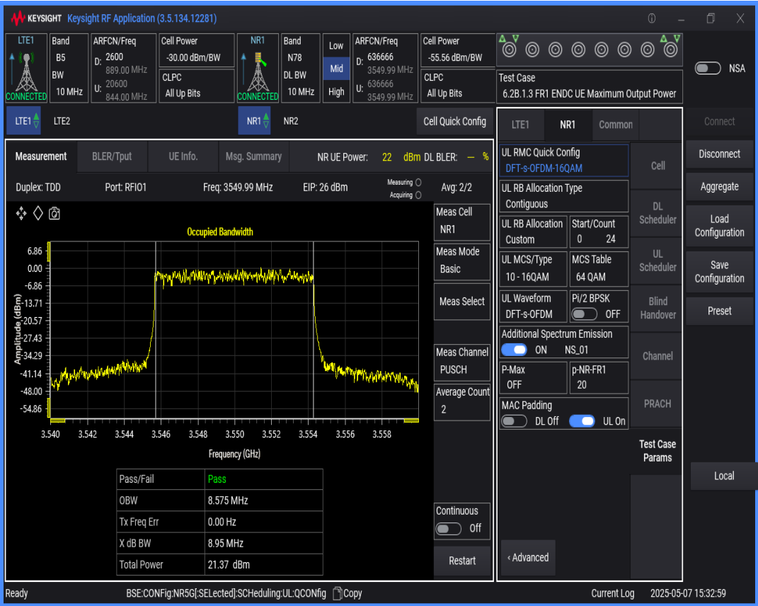
n78 SCS=30kHz DFT_QAM16 BW=100MHz Channel=636666 RB=270@0
