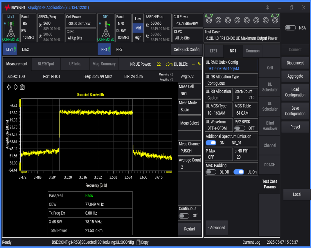
n78 SCS=30kHz DFT_QAM256 BW=100MHz Channel=636666 RB=270@0
