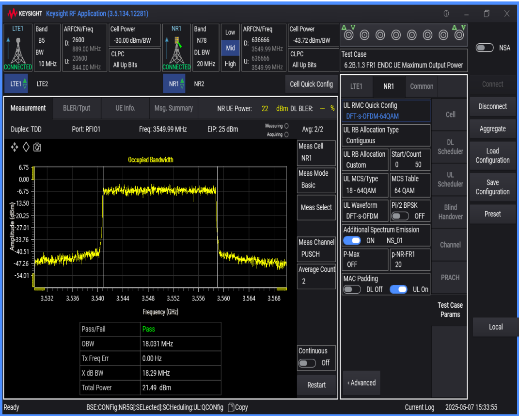
n78 SCS=30kHz DFT_QAM64 BW=15MHz Channel=636666 RB=36@0
