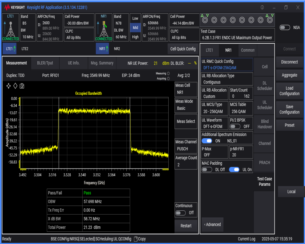
n78 SCS=30kHz DFT_QAM64 BW=100MHz Channel=636666 RB=270@0
