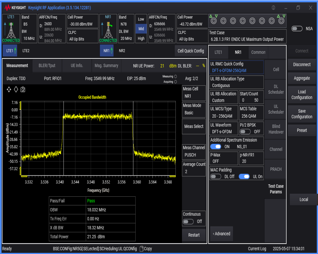
n78 SCS=30kHz DFT_QAM256 BW=80MHz Channel=636666 RB=216@0
