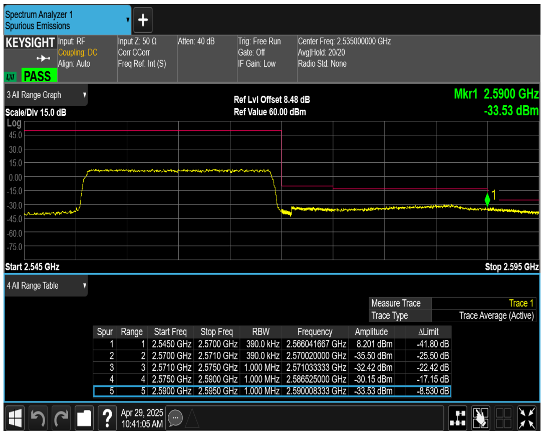
Band7 QPSK BW=20MHz Channel=20850 RB Size=100 Position=#0
