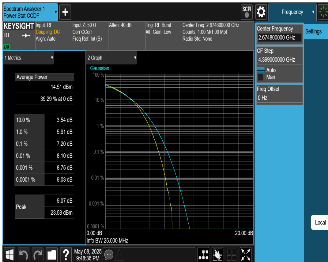
41C 16QAM PCC BW=20MHz Ch=41341 RB=100@0,SCC BW=15MHz Ch=41512 RB=75@0
