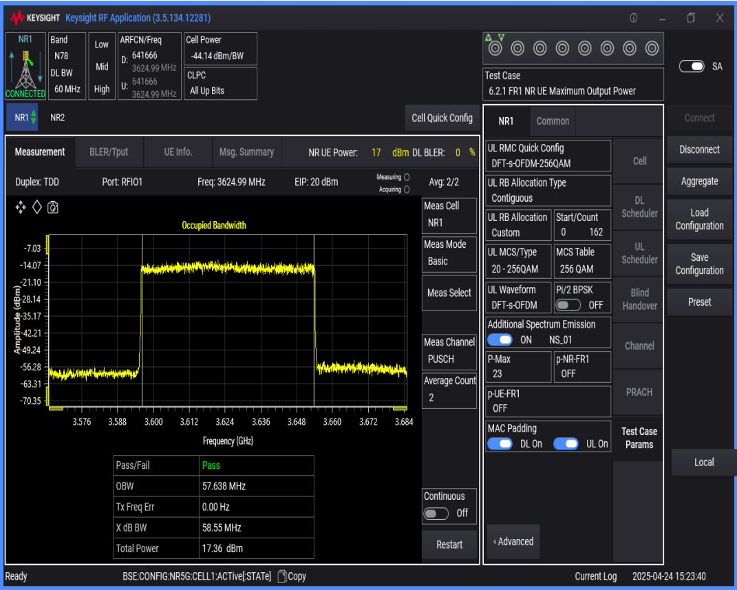
n78(3550-3700) SCS=30kHz DFT_QAM256 BW=70MHz Channel=641666 RB=180@0
