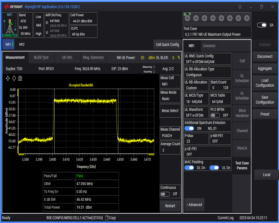
n78(3550-3700) SCS=30kHz DFT_QAM64 BW=100MHz Channel=641666 RB=270@0
