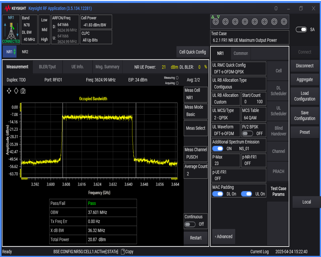
n78(3550-3700) SCS=30kHz DFT_QPSK BW=15MHz Channel=641666 RB=36@0
