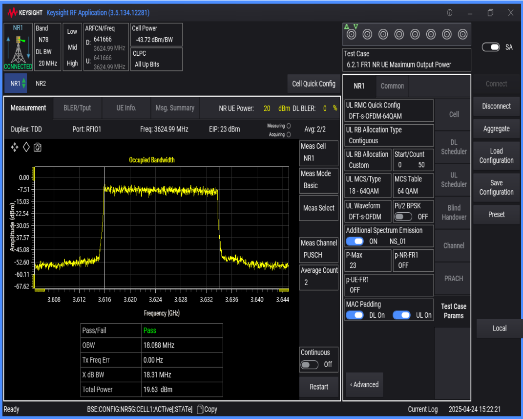
n78(3550-3700) SCS=30kHz DFT_QAM64 BW=40MHz Channel=641666 RB=100@0
