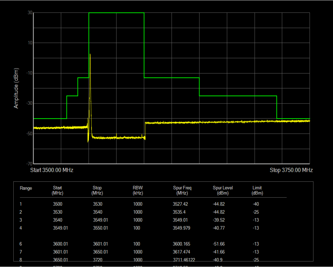
n78(3550-3700) SCS=30kHz CP_QPSK BW=50MHz Channel=645000 RB=133@0
