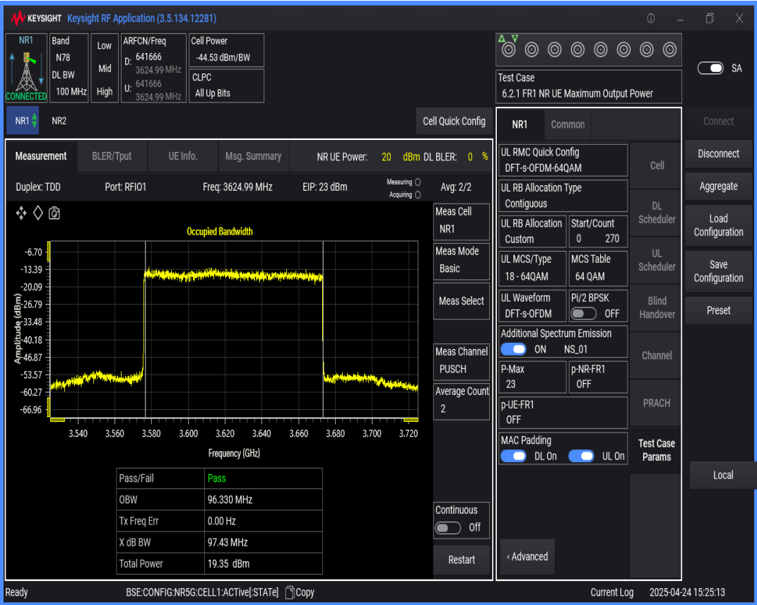
n78(3550-3700) SCS=30kHz DFT_QAM64 BW=10MHz Channel=641666 RB=24@0
