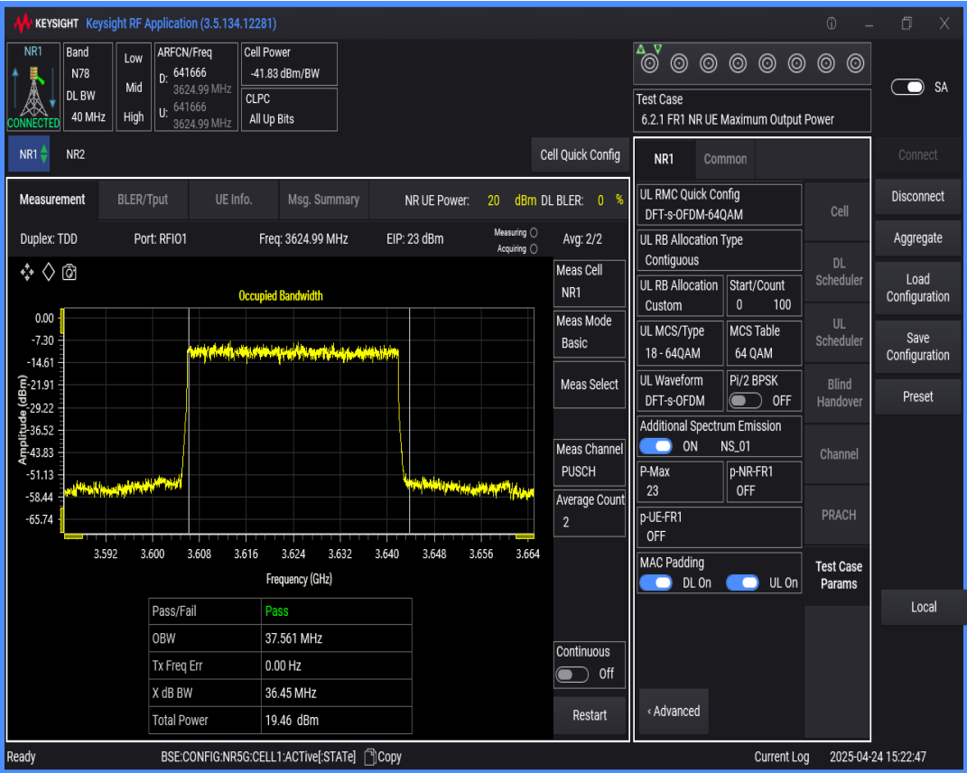
n78(3550-3700) SCS=30kHz DFT_QAM64 BW=50MHz Channel=641666 RB=128@0
