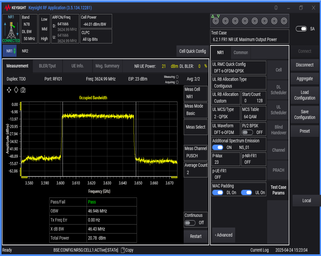
n78(3550-3700) SCS=30kHz DFT_QPSK BW=60MHz Channel=641666 RB=162@0
