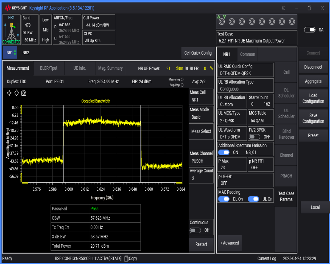
n78(3550-3700) SCS=30kHz DFT_QPSK BW=40MHz Channel=641666 RB=100@0
