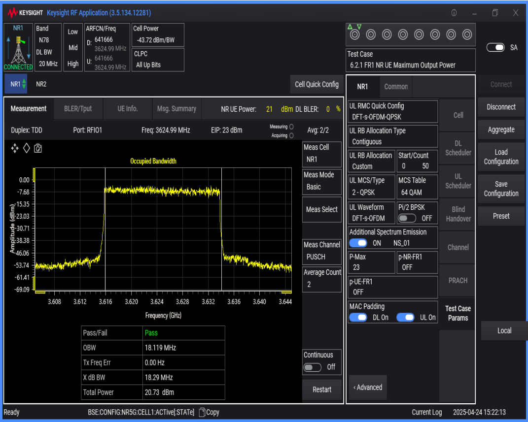
n78(3550-3700) SCS=30kHz DFT_QPSK BW=80MHz Channel=641666 RB=216@0
