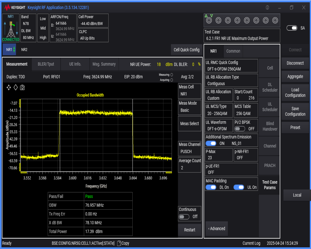
n78(3550-3700) SCS=30kHz DFT_QAM256 BW=90MHz Channel=641666 RB=240@0
