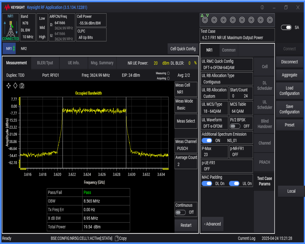
n78(3550-3700) SCS=30kHz DFT_QAM64 BW=15MHz Channel=641666 RB=36@0
