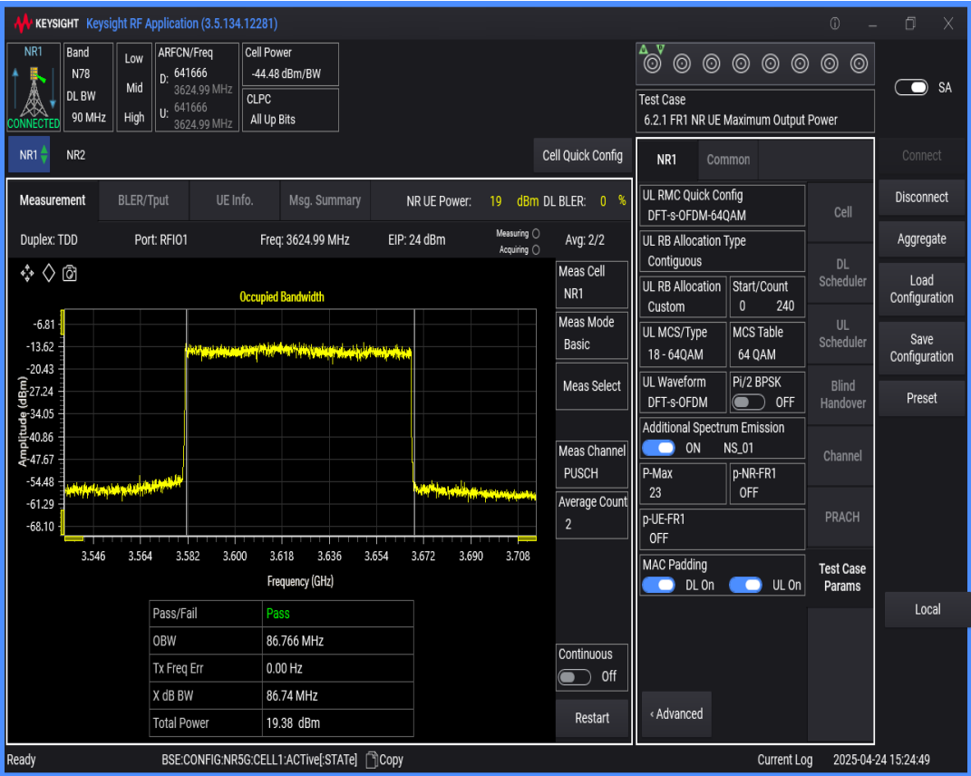
n78(3550-3700) SCS=30kHz DFT_QPSK BW=10MHz Channel=641666 RB=24@0
