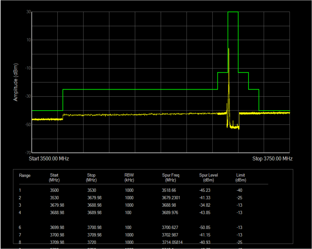
n78(3550-3700) SCS=30kHz CP_QPSK BW=10MHz Channel=646332 RB=1@23
