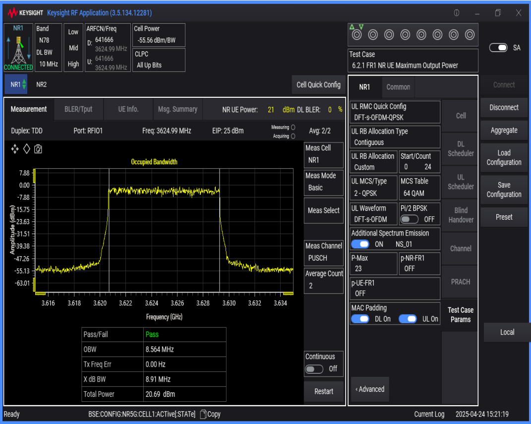
n78(3550-3700) SCS=30kHz DFT_QPSK BW=100MHz Channel=641666 RB=270@0
