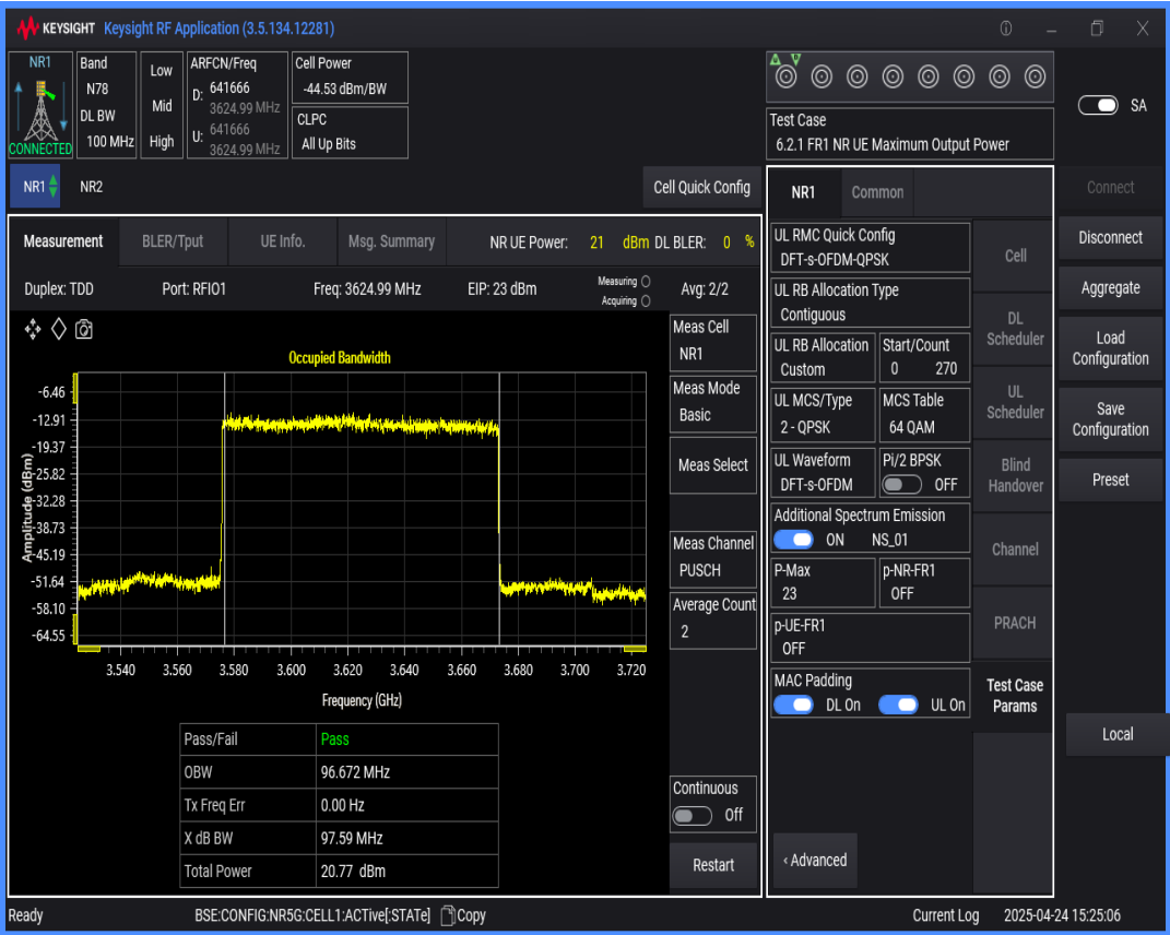
n78(3550-3700) SCS=30kHz DFT_QPSK BW=50MHz Channel=641666 RB=128@0
