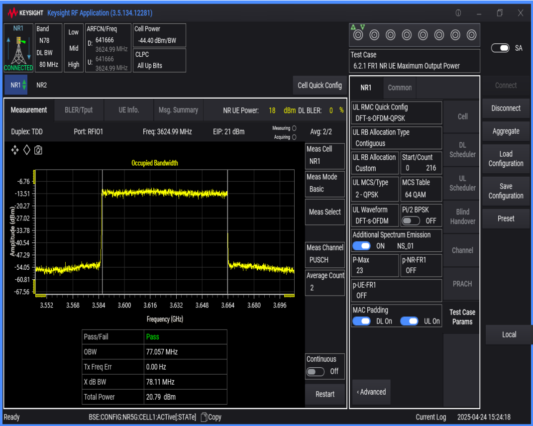
n78(3550-3700) SCS=30kHz DFT_QPSK BW=70MHz Channel=641666 RB=180@0
