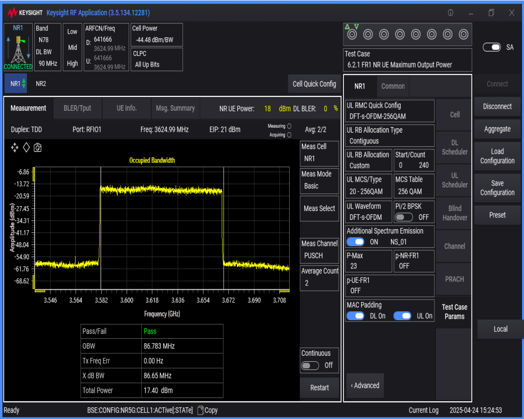
n78(3550-3700) SCS=30kHz DFT_QAM256 BW=60MHz Channel=641666 RB=162@0
