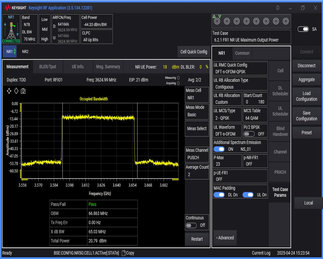
n78(3550-3700) SCS=30kHz DFT_QPSK BW=90MHz Channel=641666 RB=240@0
