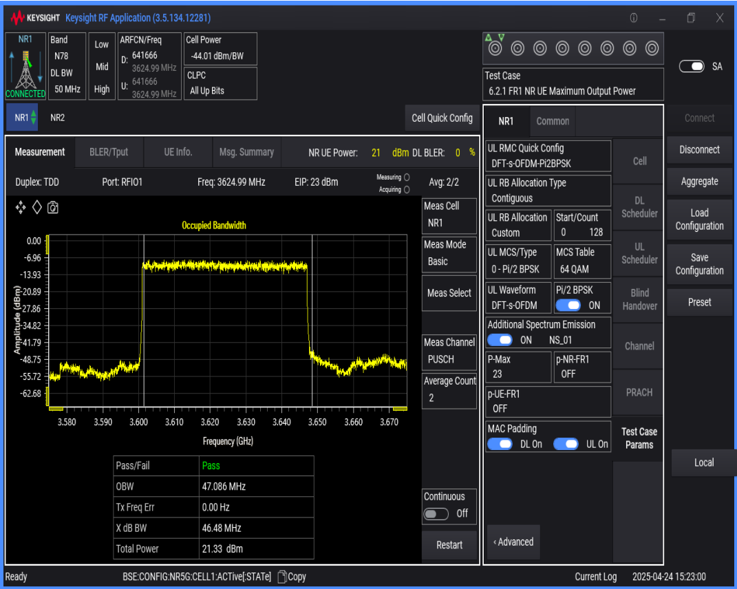
n78(3550-3700) SCS=30kHz DFT_BPSK BW=60MHz Channel=641666 RB=162@0
