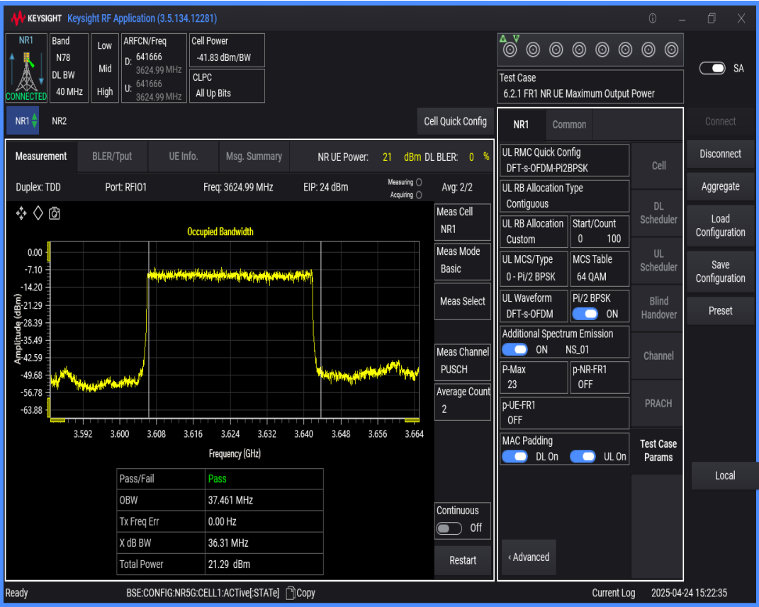
n78(3550-3700) SCS=30kHz DFT_BPSK BW=50MHz Channel=641666 RB=128@0
