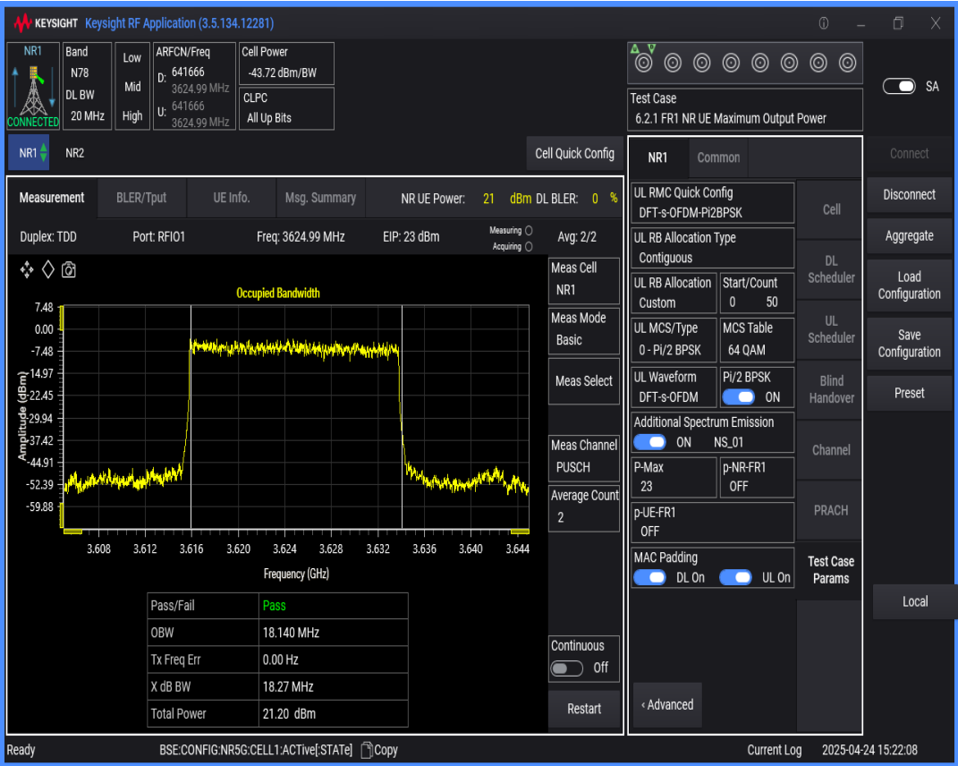
n78(3550-3700) SCS=30kHz DFT_BPSK BW=40MHz Channel=641666 RB=100@0
