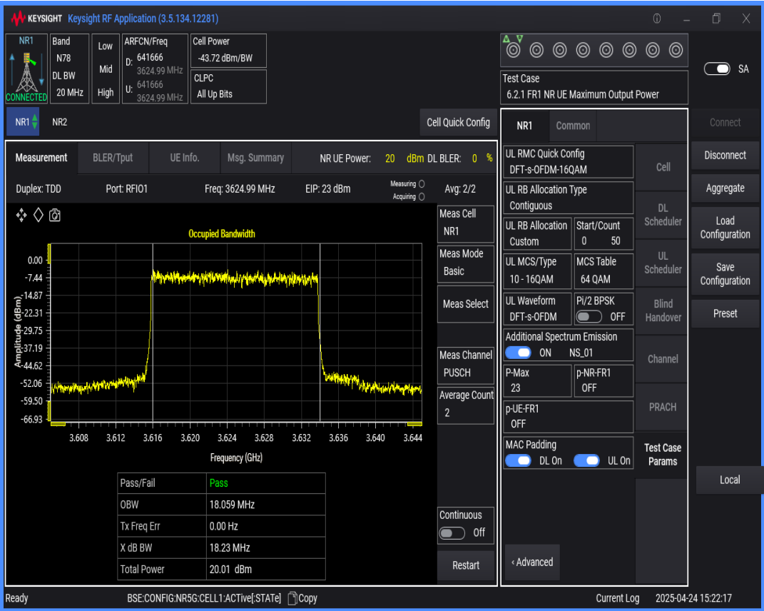
n78(3550-3700) SCS=30kHz DFT_QAM16 BW=50MHz Channel=641666 RB=128@0
