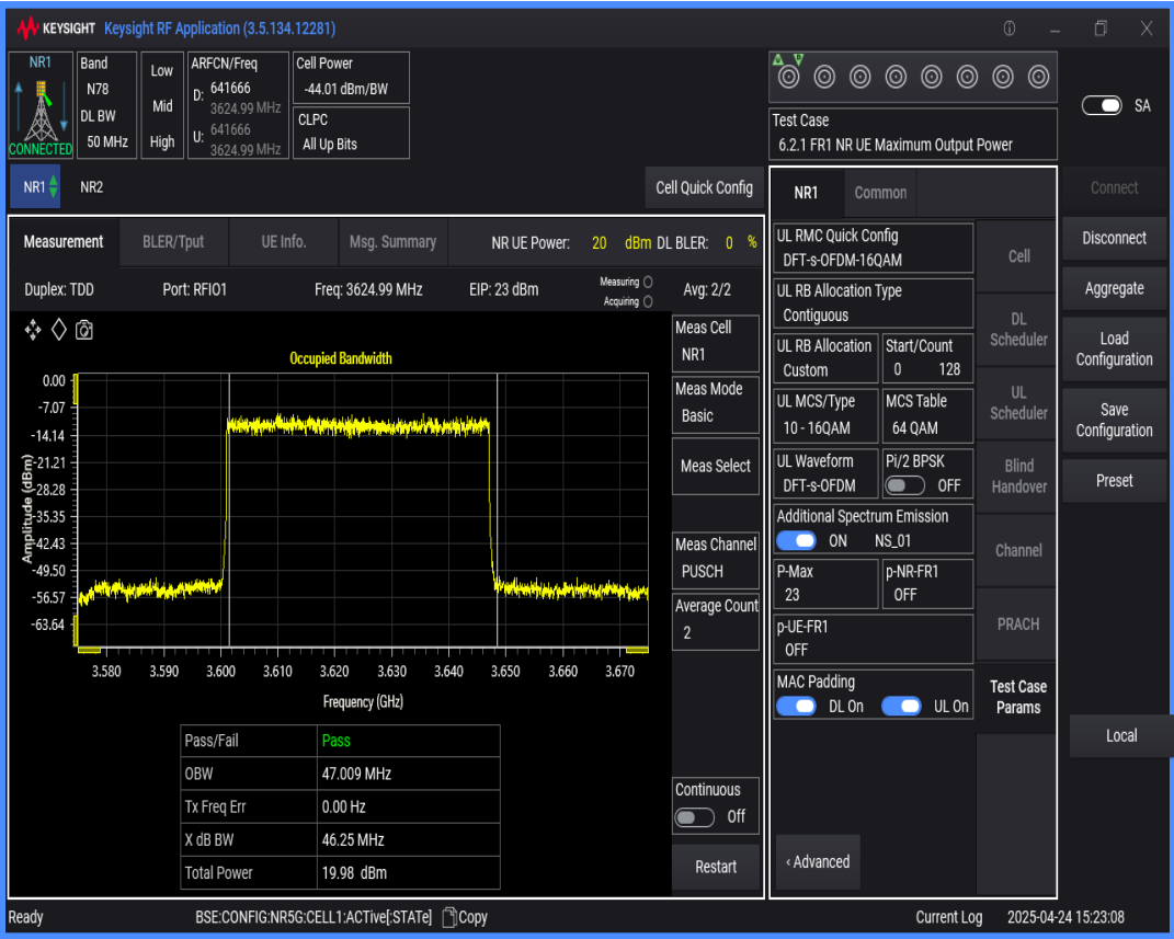
n78(3550-3700) SCS=30kHz DFT_QAM16 BW=40MHz Channel=641666 RB=100@0
