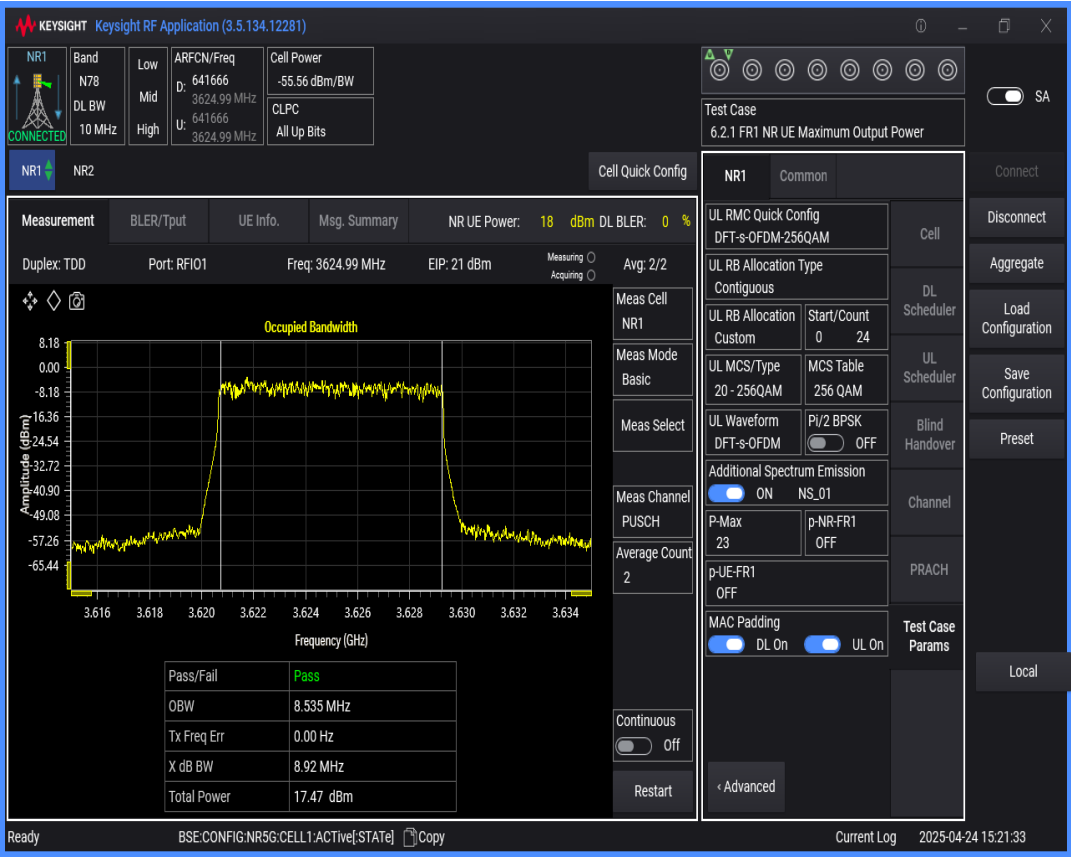
n78(3550-3700) SCS=30kHz DFT_QAM256 BW=15MHz Channel=641666 RB=36@0
