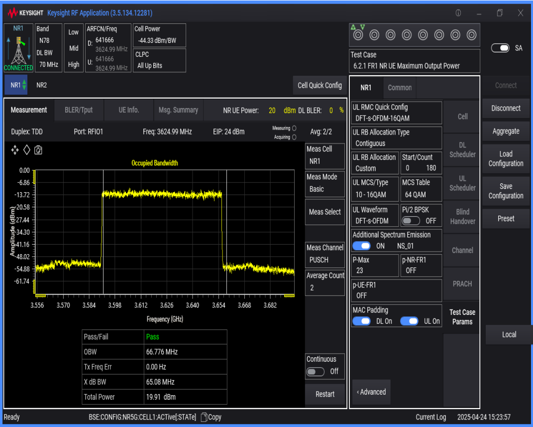
n78(3550-3700) SCS=30kHz DFT_QAM256 BW=40MHz Channel=641666 RB=100@0
