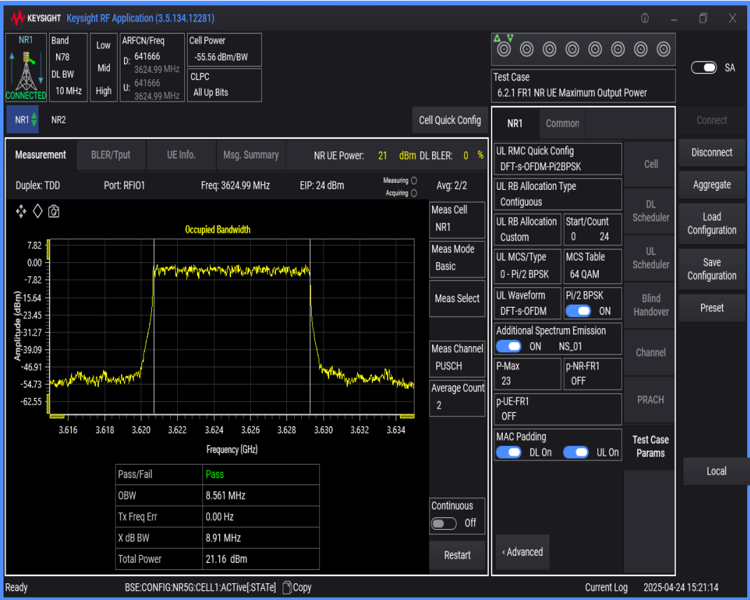
n78(3550-3700) SCS=30kHz DFT_BPSK BW=15MHz Channel=641666 RB=36@0
