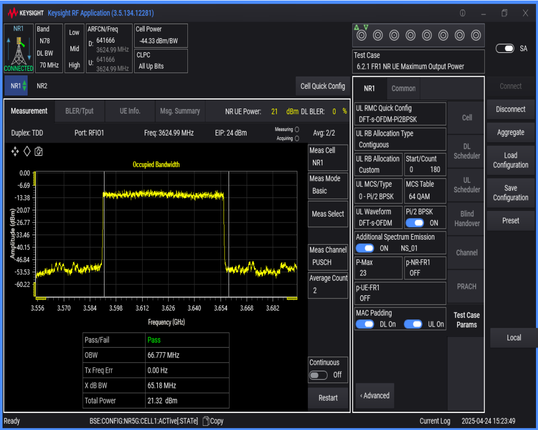
n78(3550-3700) SCS=30kHz DFT_BPSK BW=80MHz Channel=641666 RB=216@0
