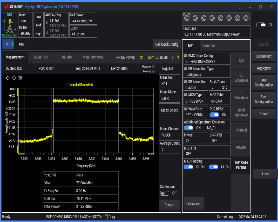
n78(3550-3700) SCS=30kHz DFT_BPSK BW=90MHz Channel=641666 RB=240@0
