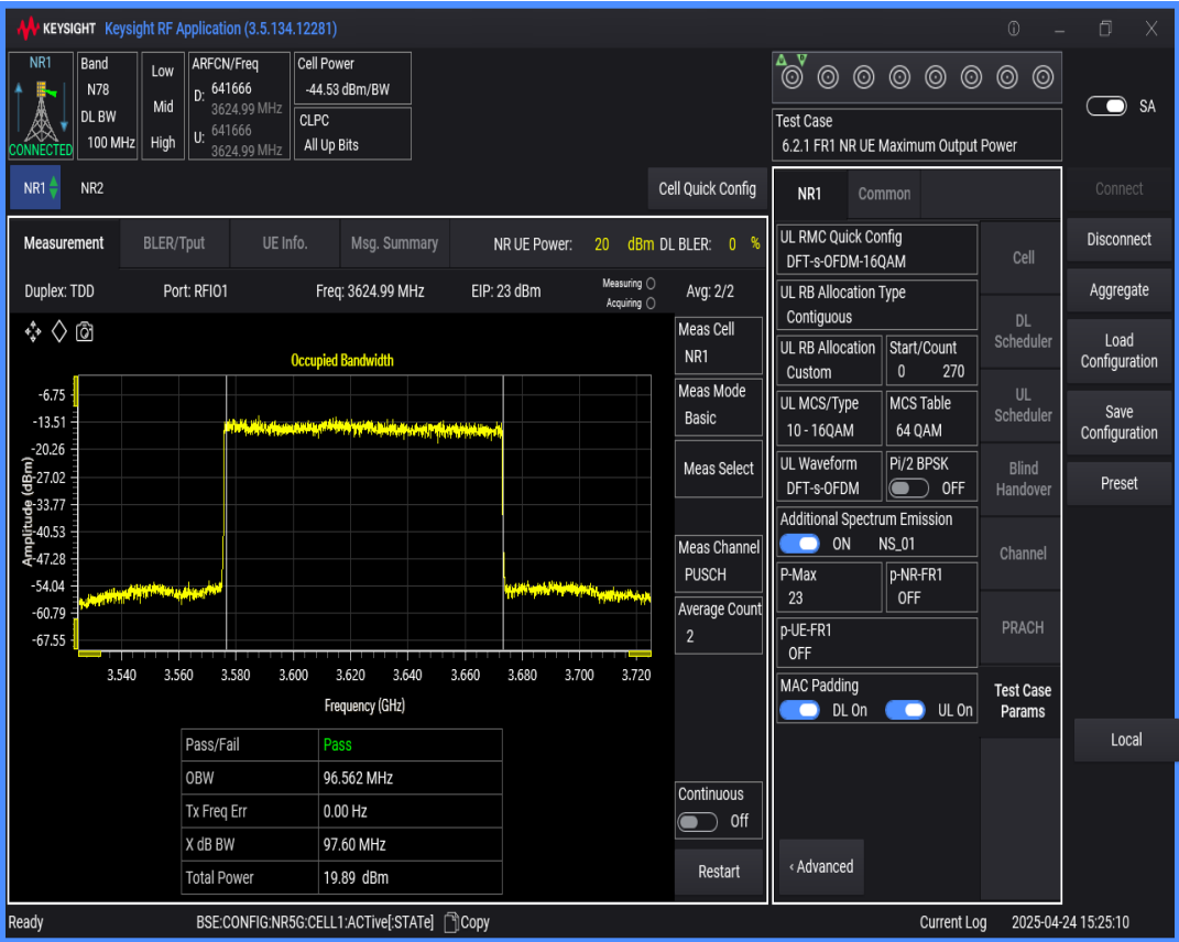
n78(3550-3700) SCS=30kHz DFT_QAM16 BW=15MHz Channel=641666 RB=36@0
