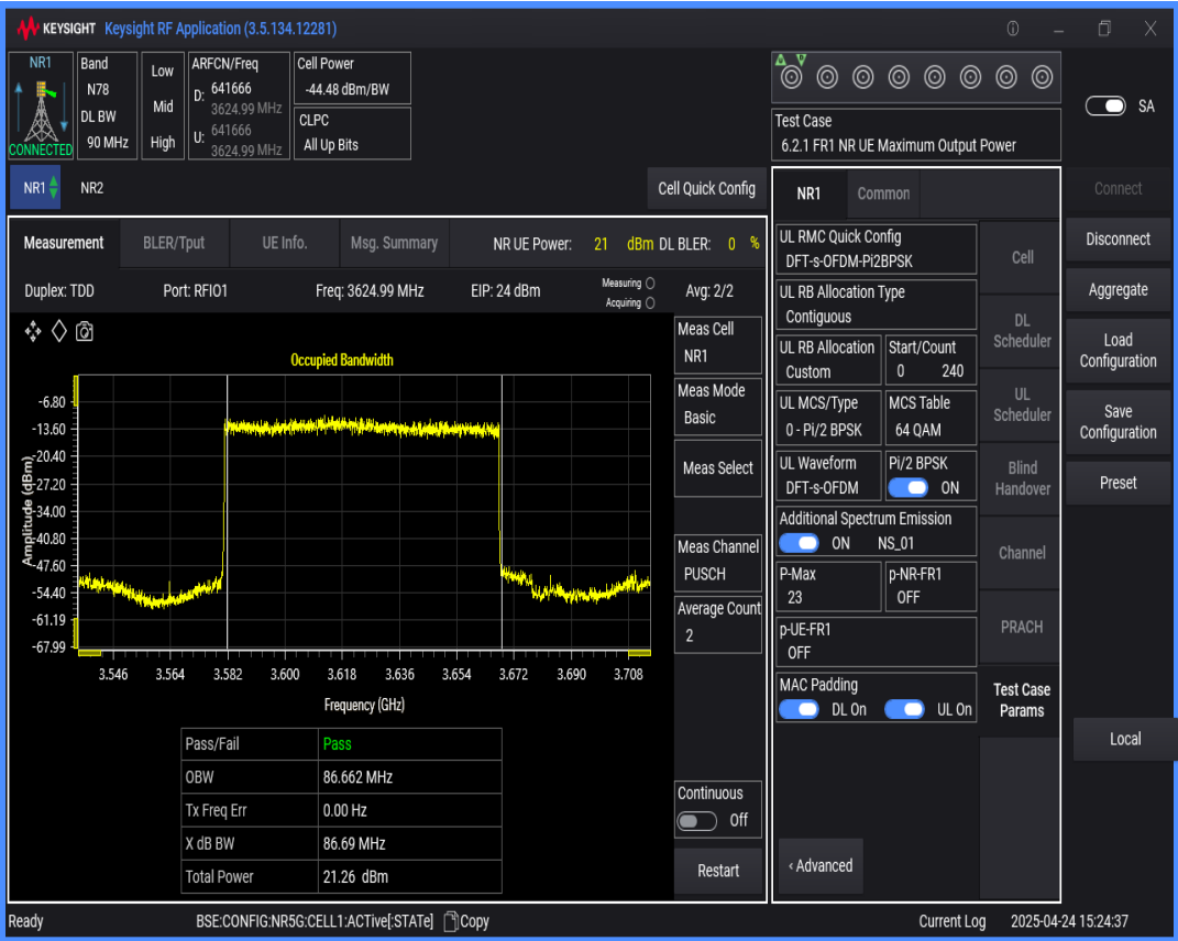
n78(3550-3700) SCS=30kHz DFT_QAM16 BW=10MHz Channel=641666 RB=24@0
