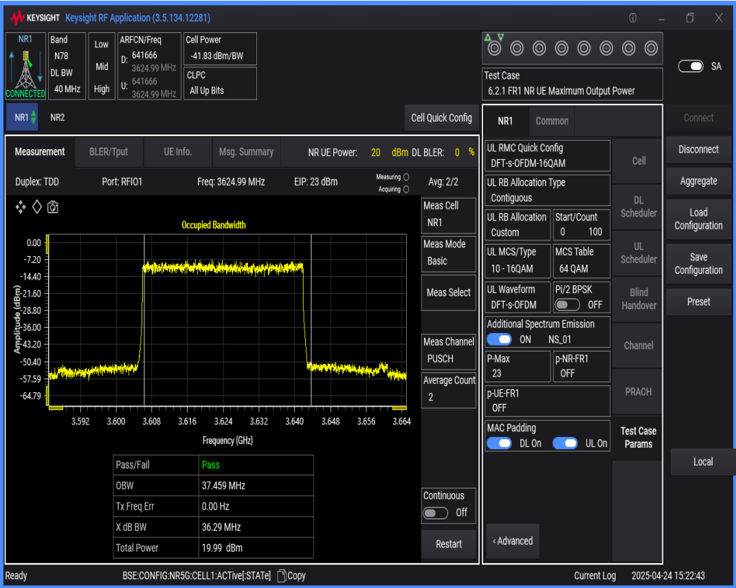
n78(3550-3700) SCS=30kHz DFT_QAM16 BW=90MHz Channel=641666 RB=240@0
