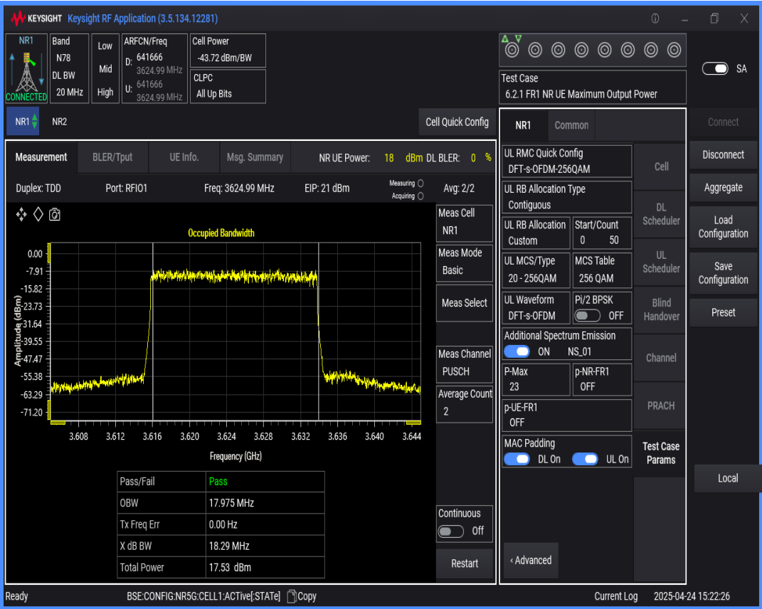
n78(3550-3700) SCS=30kHz DFT_QAM256 BW=10MHz Channel=641666 RB=24@0
