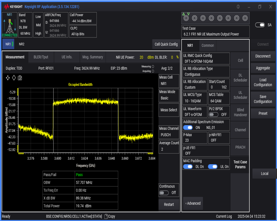
n78(3550-3700) SCS=30kHz DFT_QAM16 BW=70MHz Channel=641666 RB=180@0
