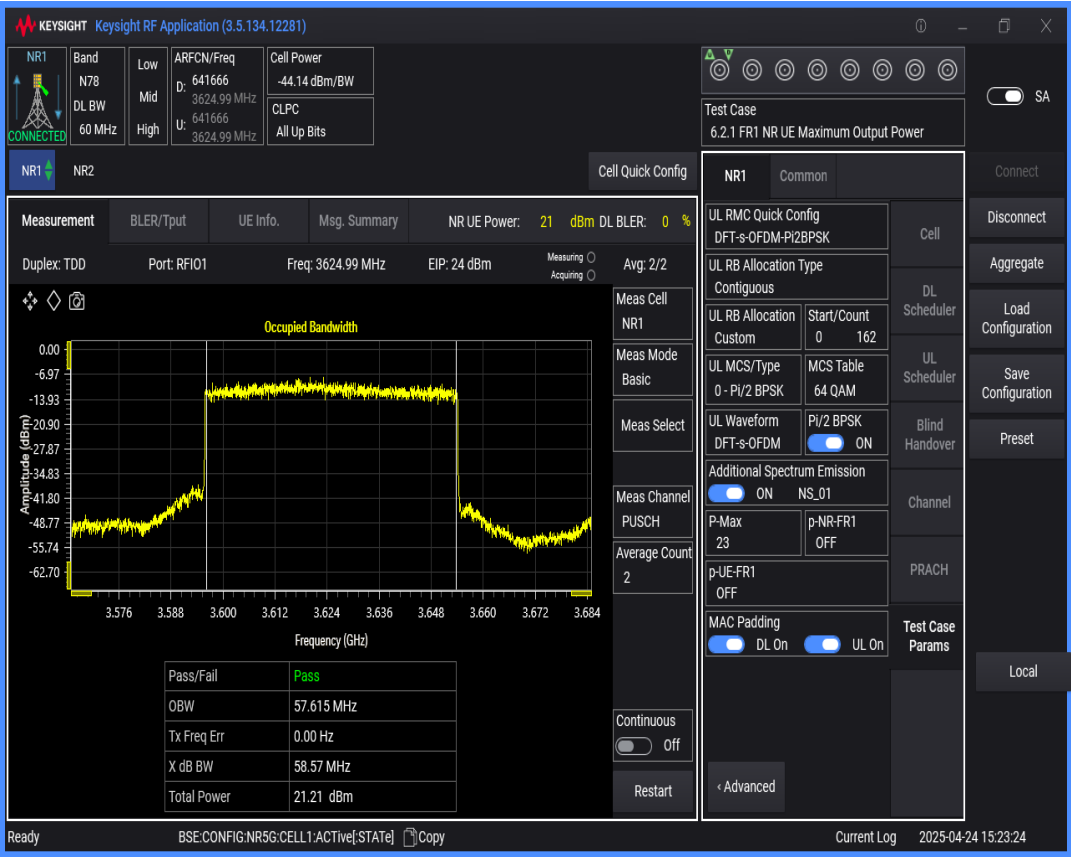
n78(3550-3700) SCS=30kHz DFT_BPSK BW=70MHz Channel=641666 RB=180@0
