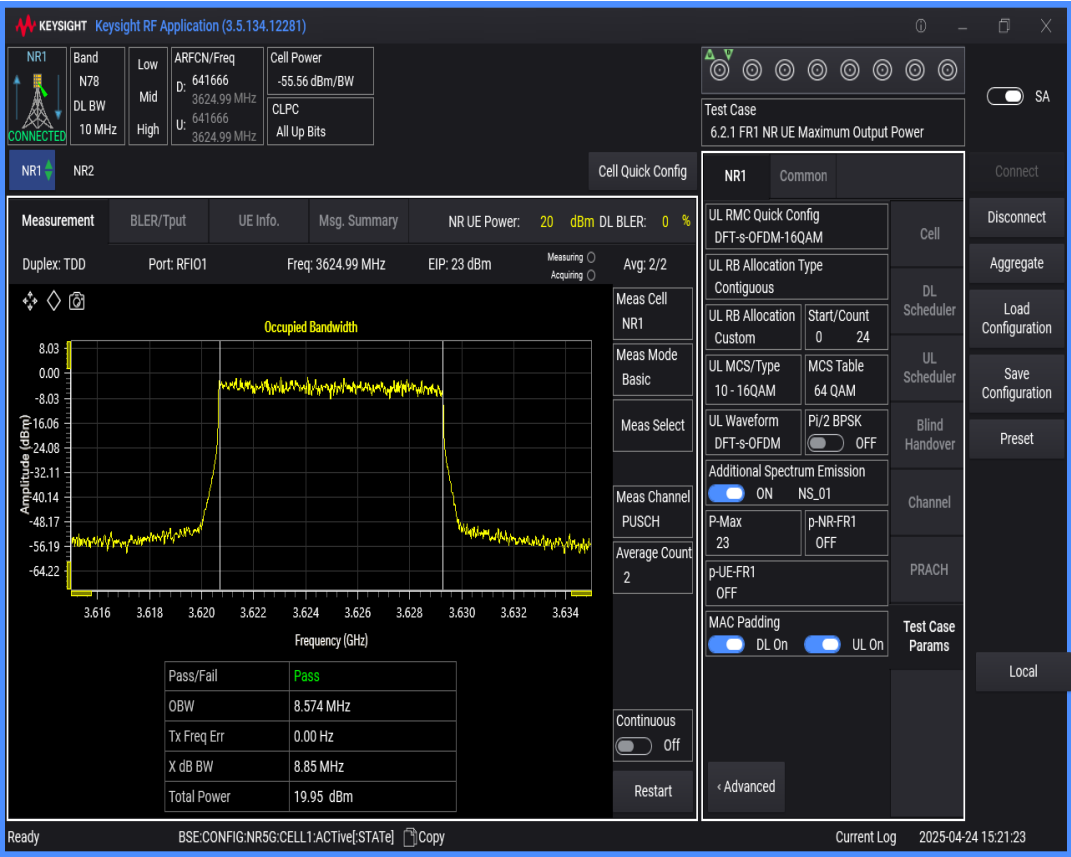
n78(3550-3700) SCS=30kHz DFT_QAM16 BW=100MHz Channel=641666 RB=270@0
