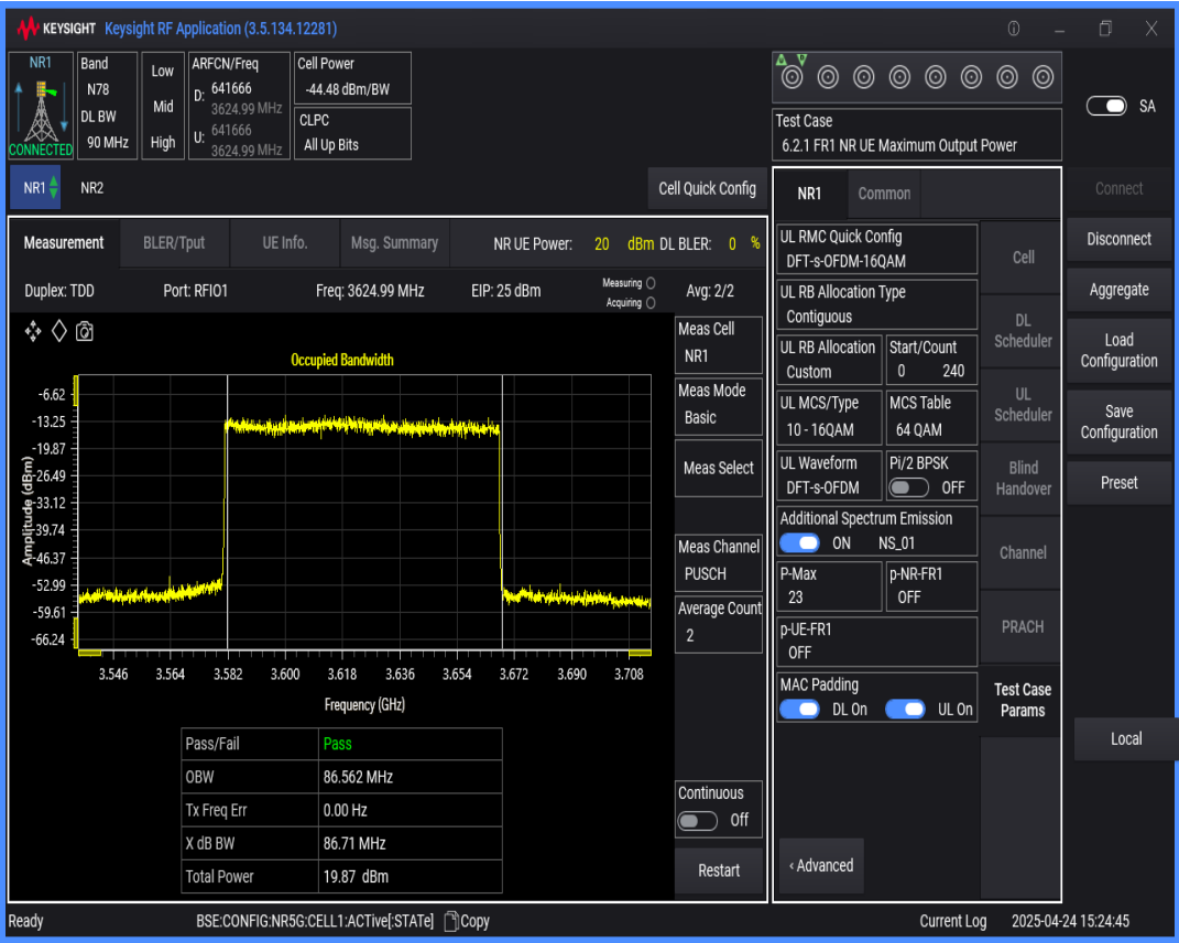
n78(3550-3700) SCS=30kHz DFT_QAM256 BW=100MHz Channel=641666 RB=270@0
