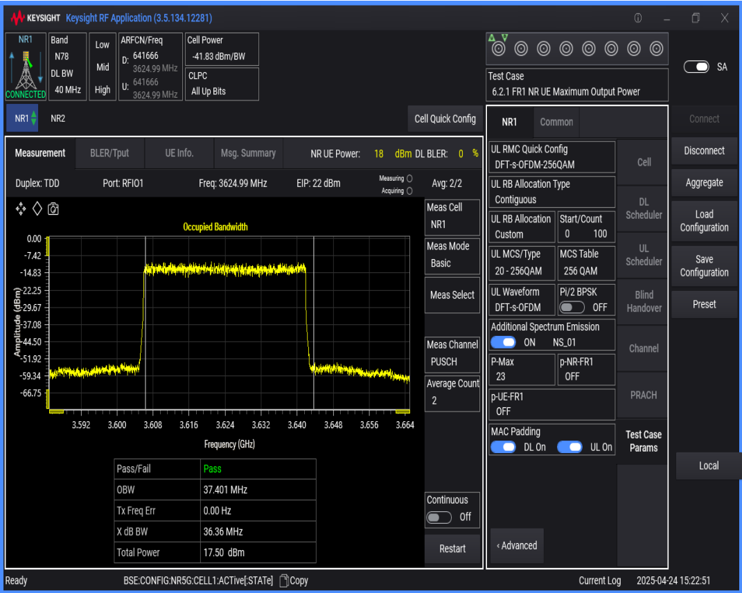
n78(3550-3700) SCS=30kHz DFT_QAM256 BW=50MHz Channel=641666 RB=128@0
