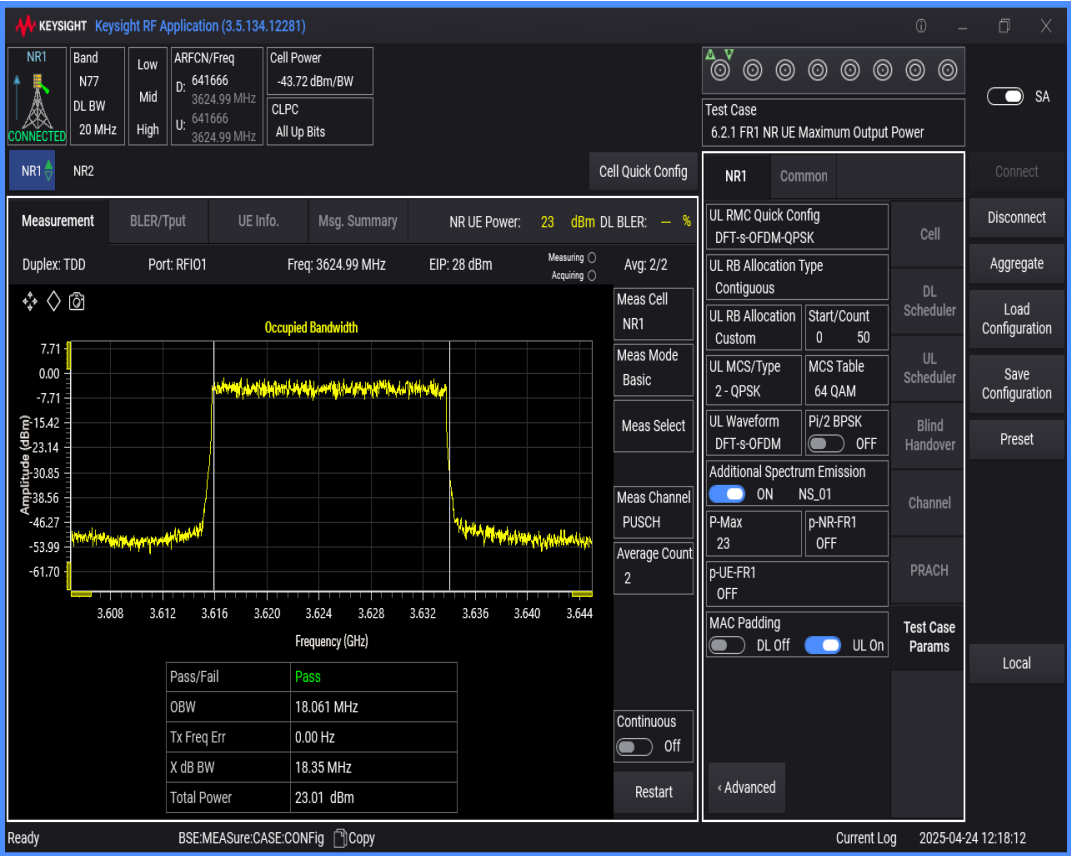
n77(3550-3700) SCS=30kHz DFT_QPSK BW=40MHz Channel=641666 RB=100@0
