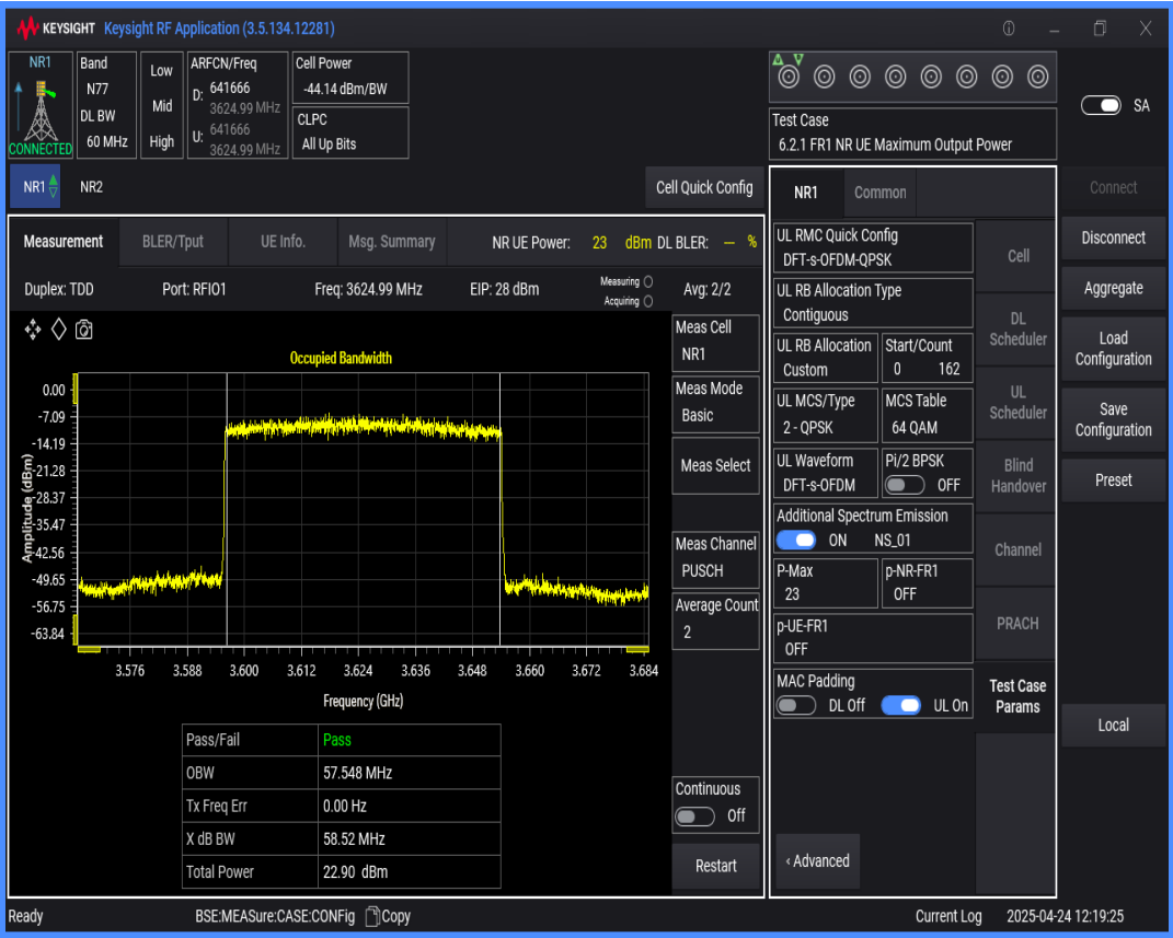
n77(3550-3700) SCS=30kHz DFT_QPSK BW=90MHz Channel=641666 RB=240@0
