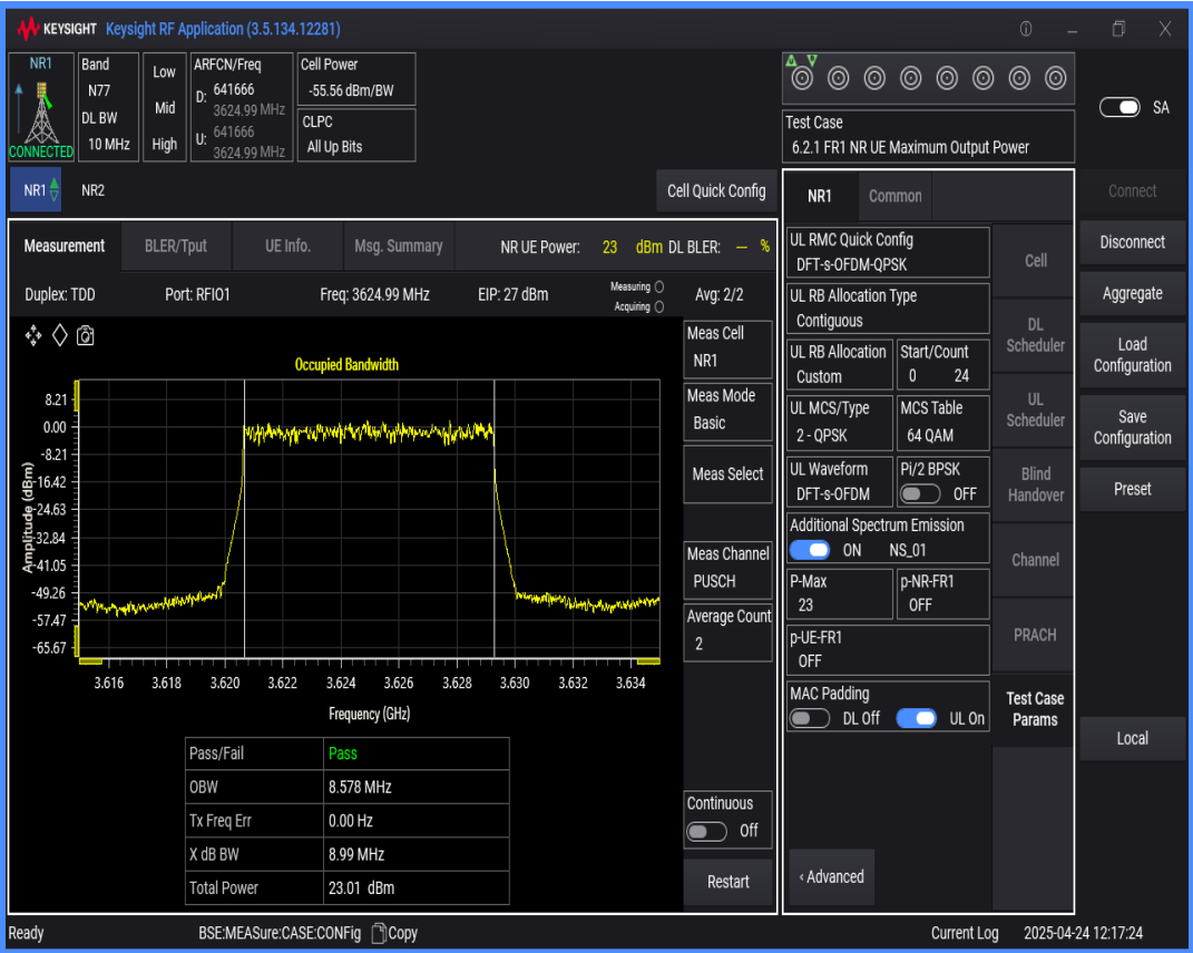
n77(3550-3700) SCS=30kHz DFT_QPSK BW=15MHz Channel=641666 RB=36@0
