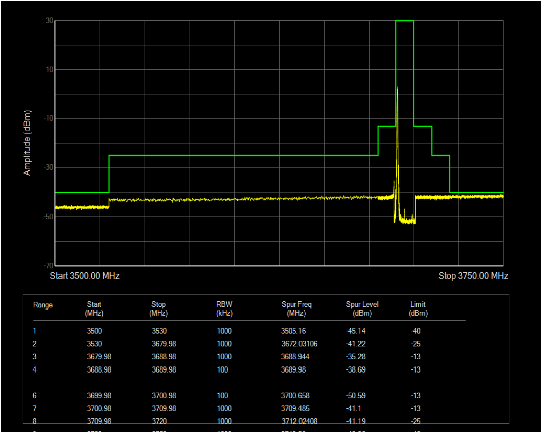
n77(3550-3700) SCS=30kHz CP_QPSK BW=10MHz Channel=646332 RB=1@23
