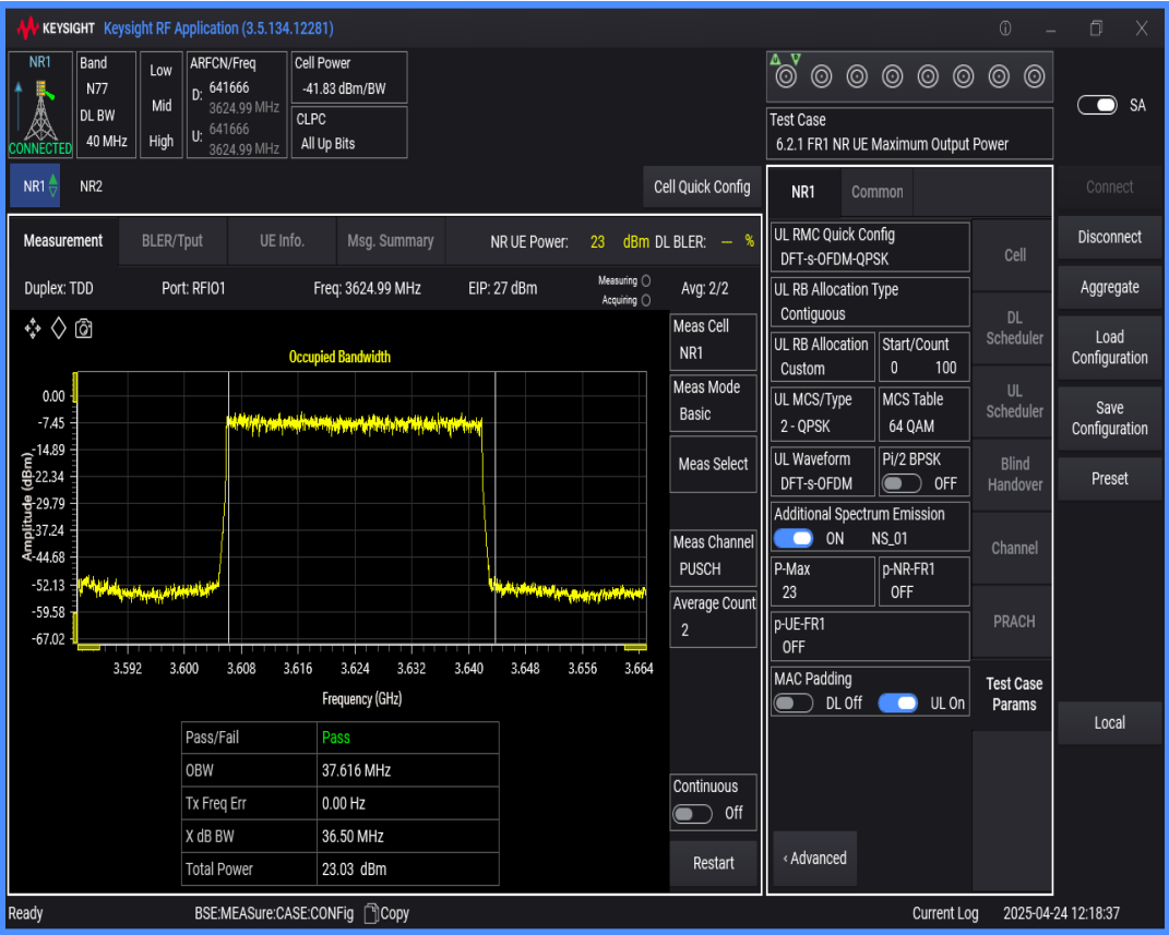
n77(3550-3700) SCS=30kHz DFT_QPSK BW=50MHz Channel=641666 RB=128@0
