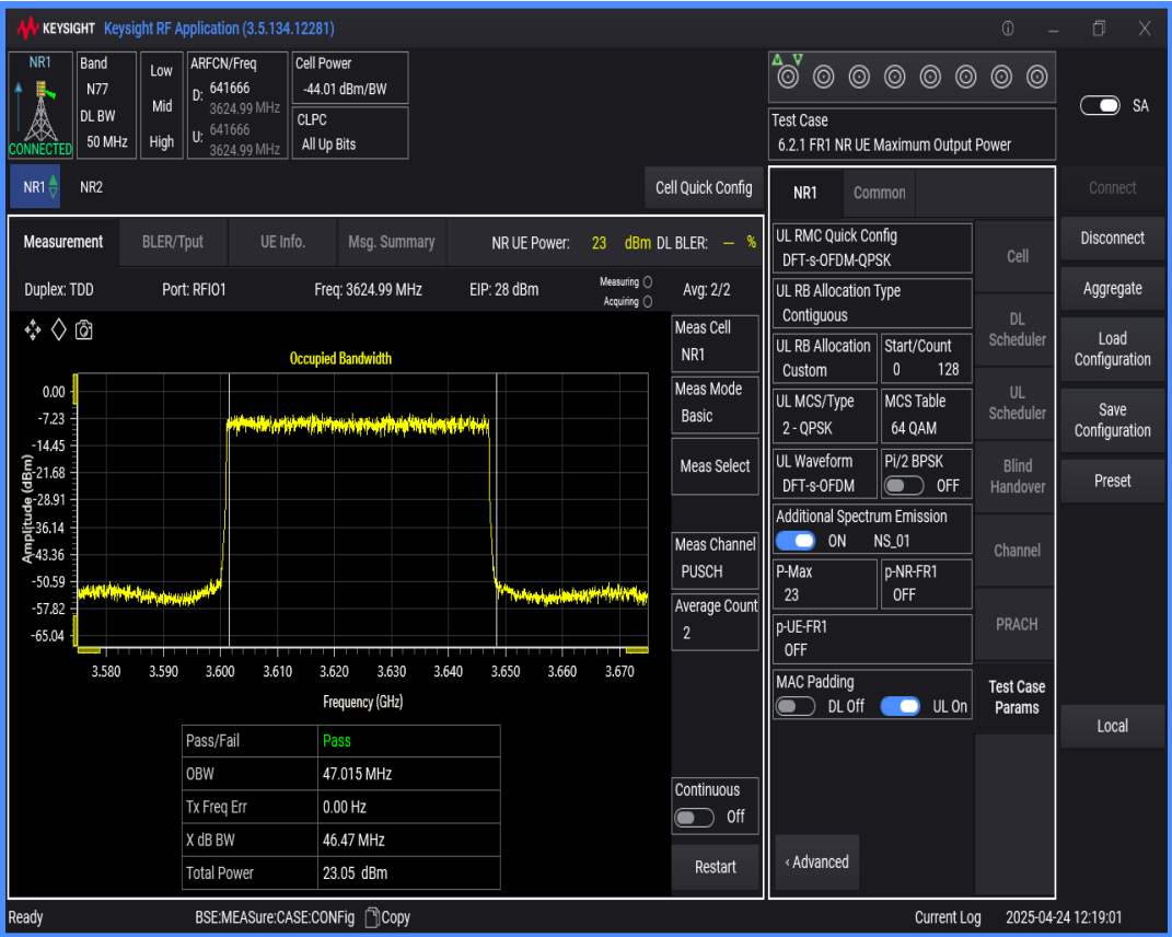
n77(3550-3700) SCS=30kHz DFT_QPSK BW=60MHz Channel=641666 RB=162@0
