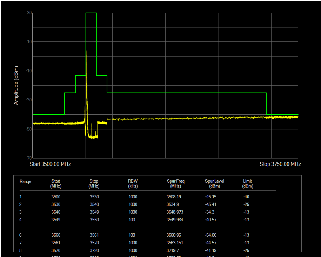
n77(3550-3700) SCS=30kHz CP_QPSK BW=10MHz Channel=637000 RB=1@23
