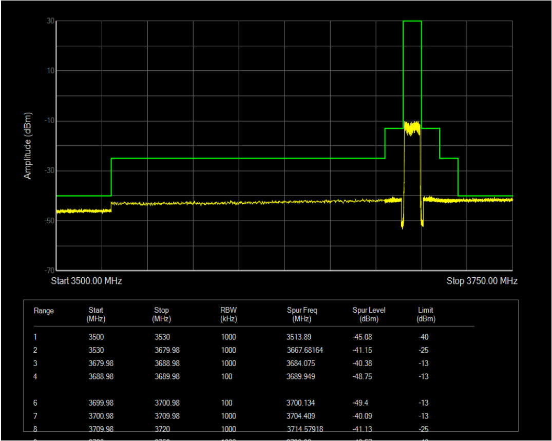
n77(3550-3700) SCS=30kHz CP_QPSK BW=50MHz Channel=638334 RB=133@0
