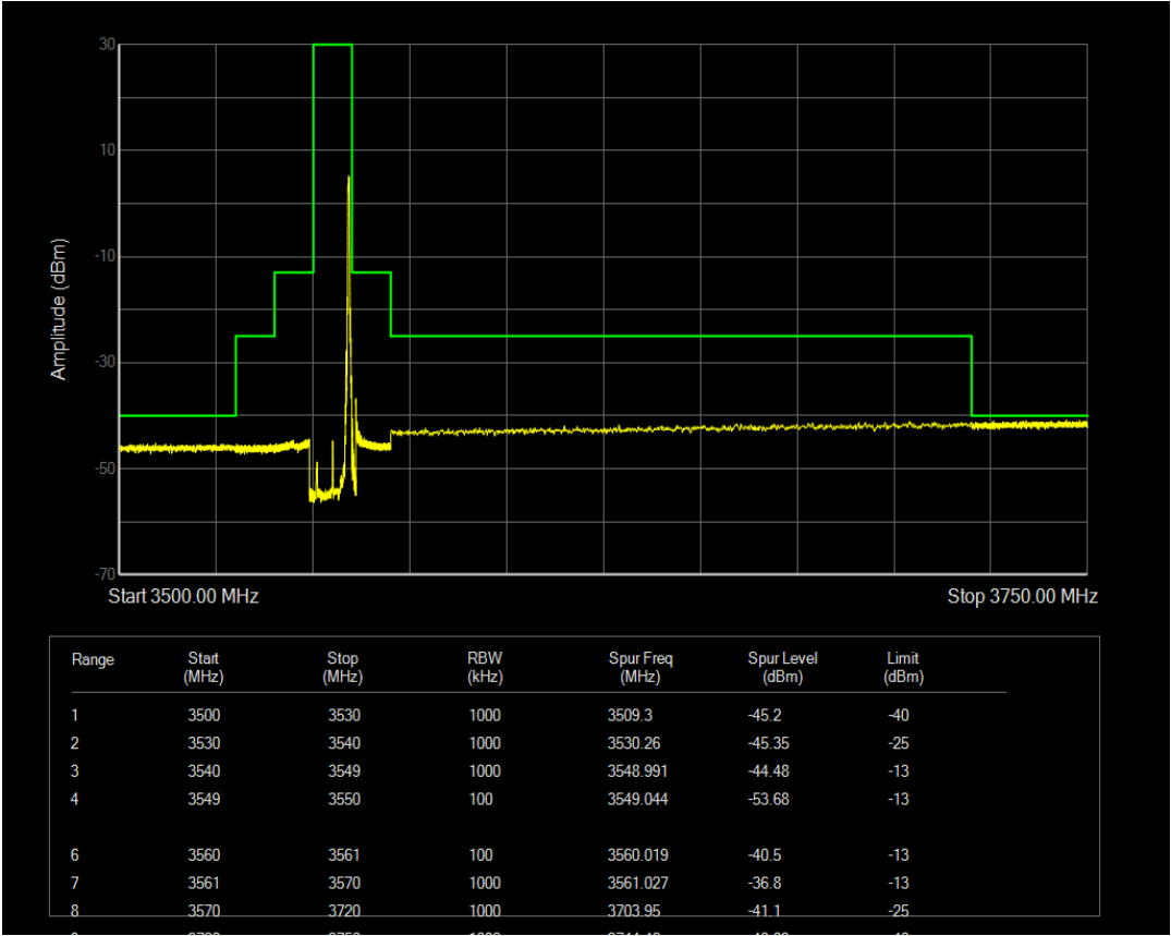
n77(3550-3700) SCS=30kHz CP_QPSK BW=10MHz Channel=637000 RB=24@0
