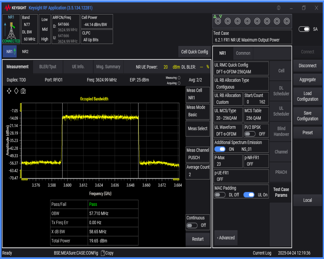
n77(3550-3700) SCS=30kHz DFT_QAM256 BW=90MHz Channel=641666 RB=240@0
