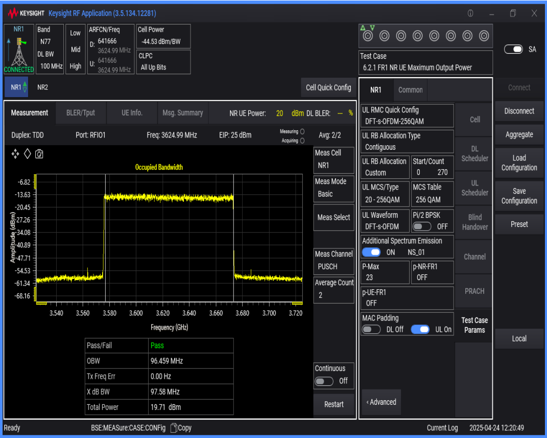
n77(3550-3700) SCS=30kHz DFT_QAM256 BW=10MHz Channel=641666 RB=24@0
