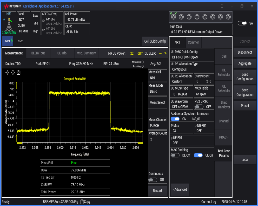
n77(3550-3700) SCS=30kHz DFT_QAM256 BW=100MHz Channel=641666 RB=270@0
