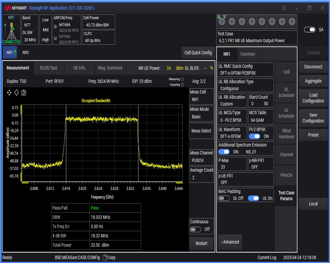
n77(3550-3700) SCS=30kHz DFT_BPSK BW=40MHz Channel=641666 RB=100@0
