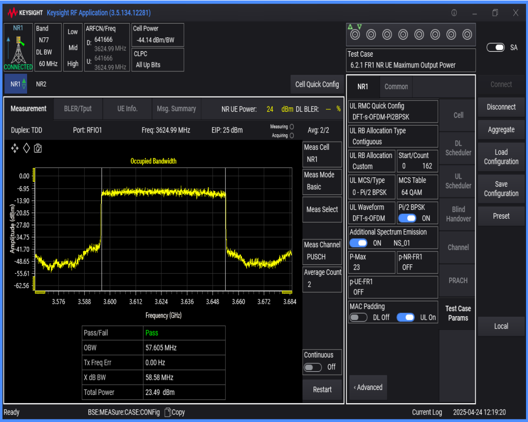
n77(3550-3700) SCS=30kHz DFT_BPSK BW=80MHz Channel=641666 RB=216@0
