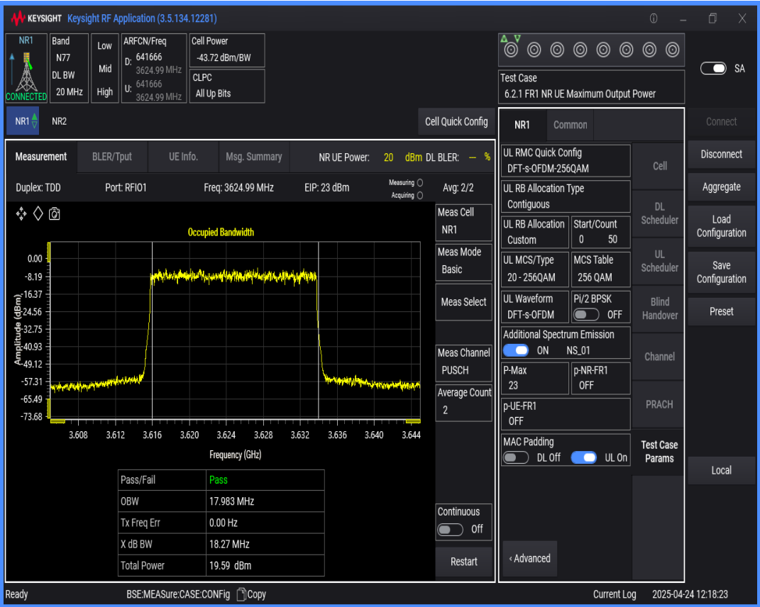
n77(3550-3700) SCS=30kHz DFT_QAM256 BW=50MHz Channel=641666 RB=128@0
