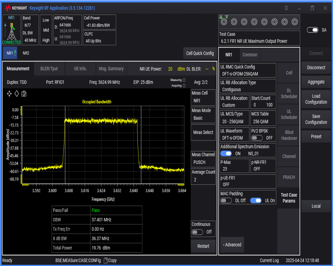
n77(3550-3700) SCS=30kHz DFT_QAM256 BW=60MHz Channel=641666 RB=162@0
