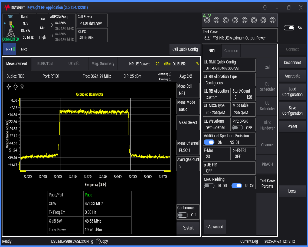
n77(3550-3700) SCS=30kHz DFT_QAM256 BW=40MHz Channel=641666 RB=100@0
