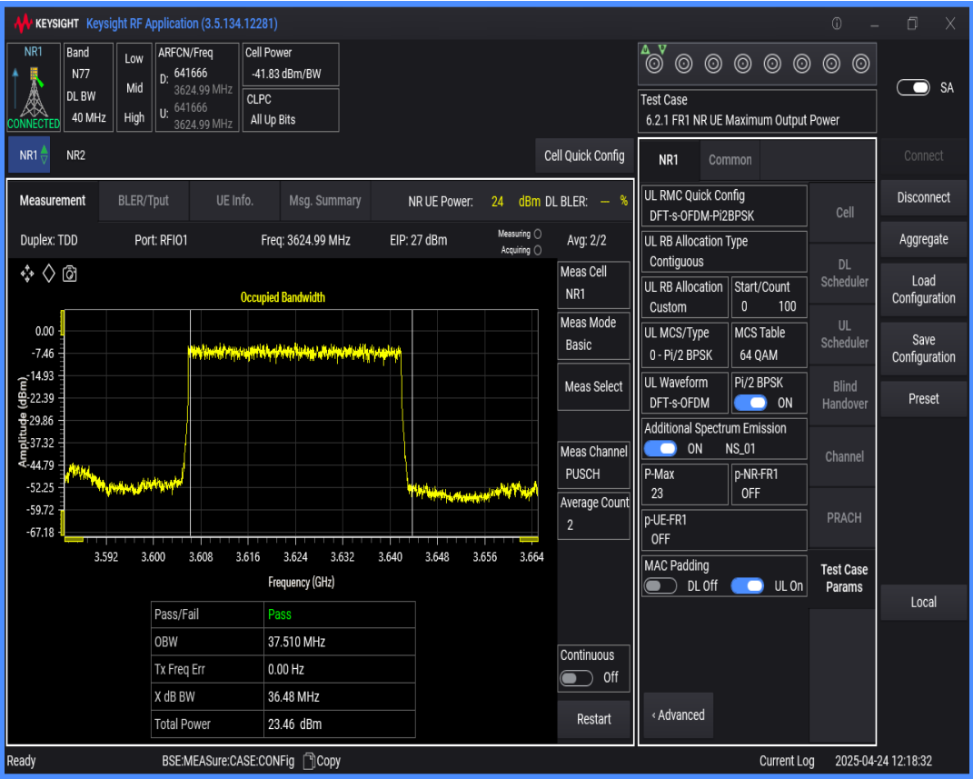
n77(3550-3700) SCS=30kHz DFT_BPSK BW=50MHz Channel=641666 RB=128@0
