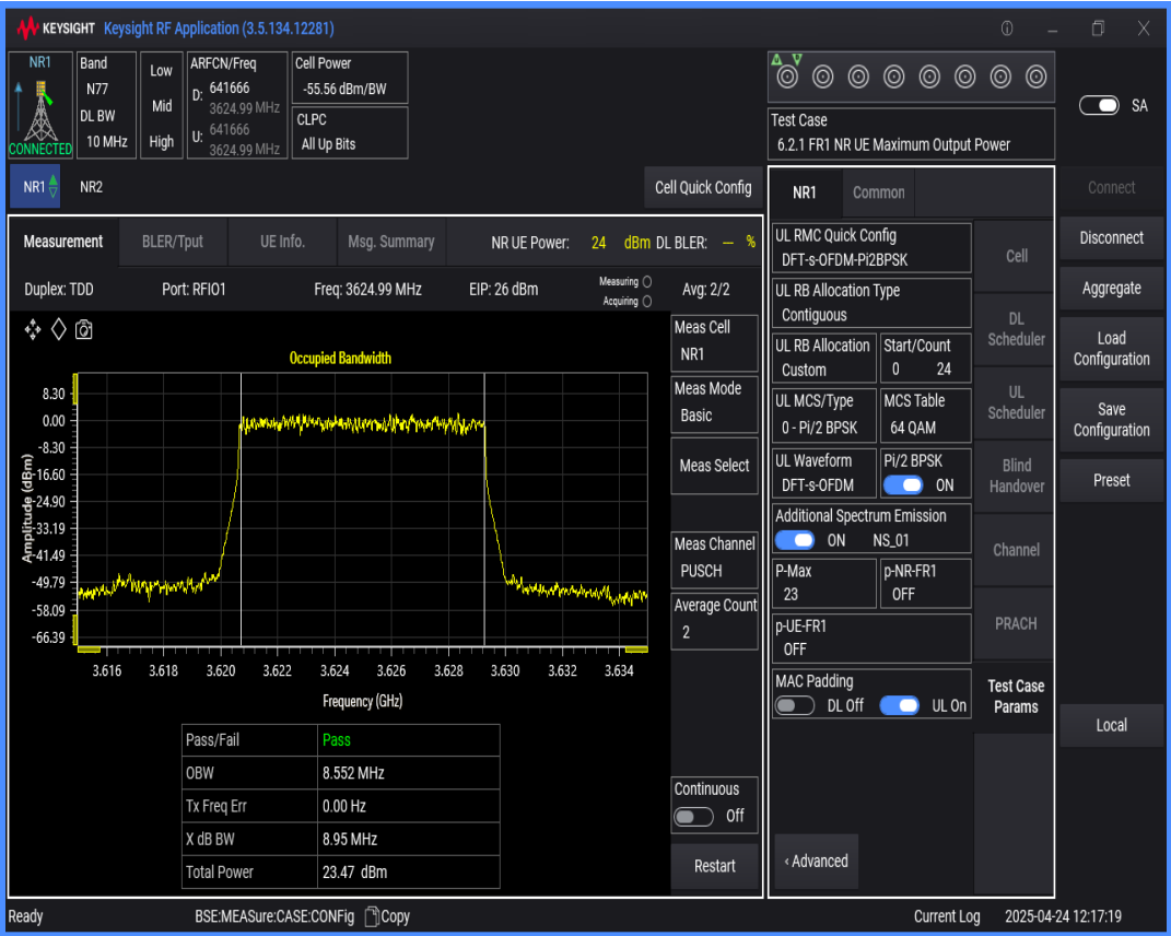
n77(3550-3700) SCS=30kHz DFT_BPSK BW=15MHz Channel=641666 RB=36@0
