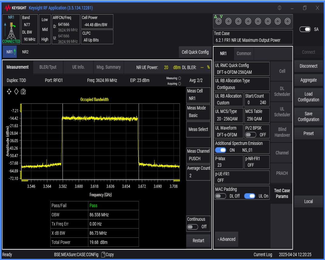
n77(3550-3700) SCS=30kHz DFT_QAM256 BW=80MHz Channel=641666 RB=216@0
