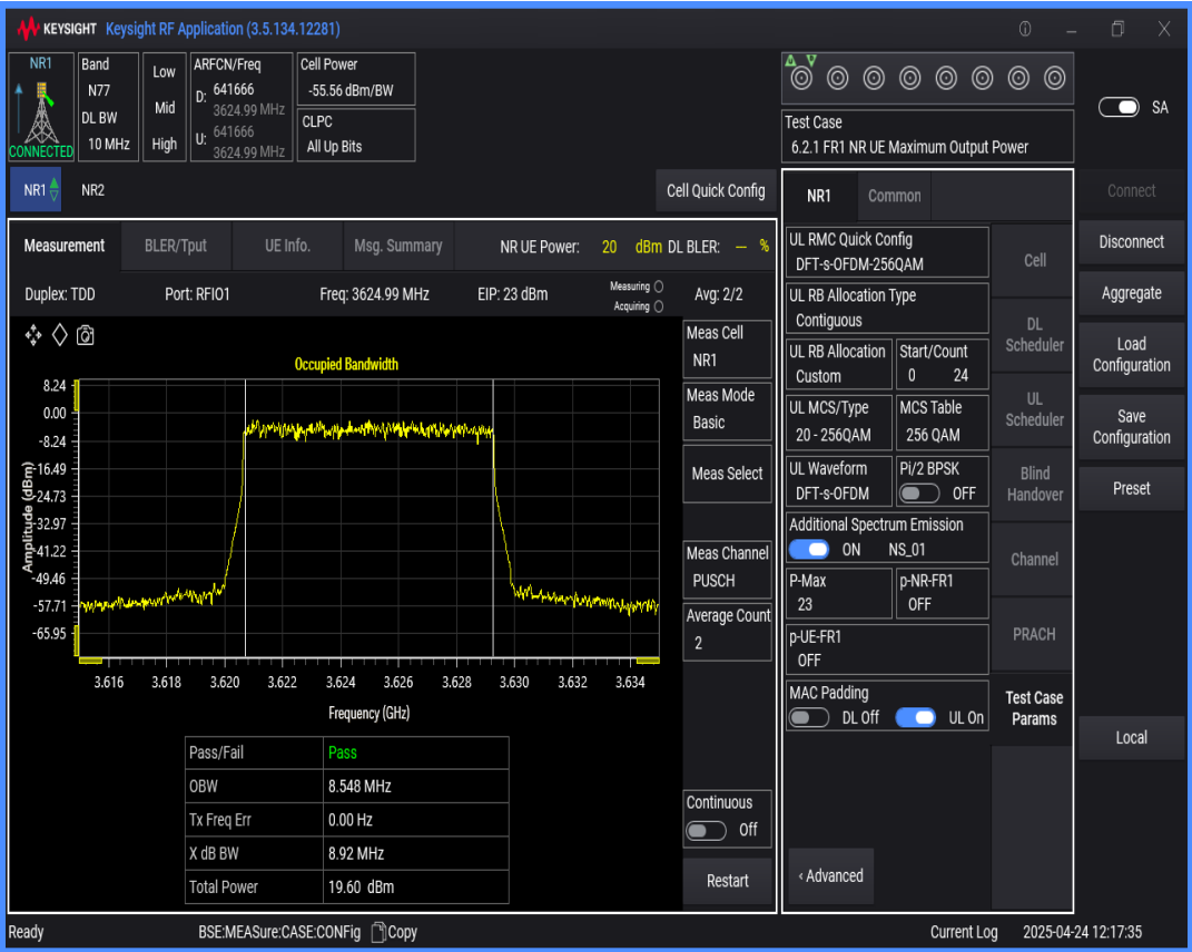
n77(3550-3700) SCS=30kHz DFT_QAM256 BW=15MHz Channel=641666 RB=36@0
