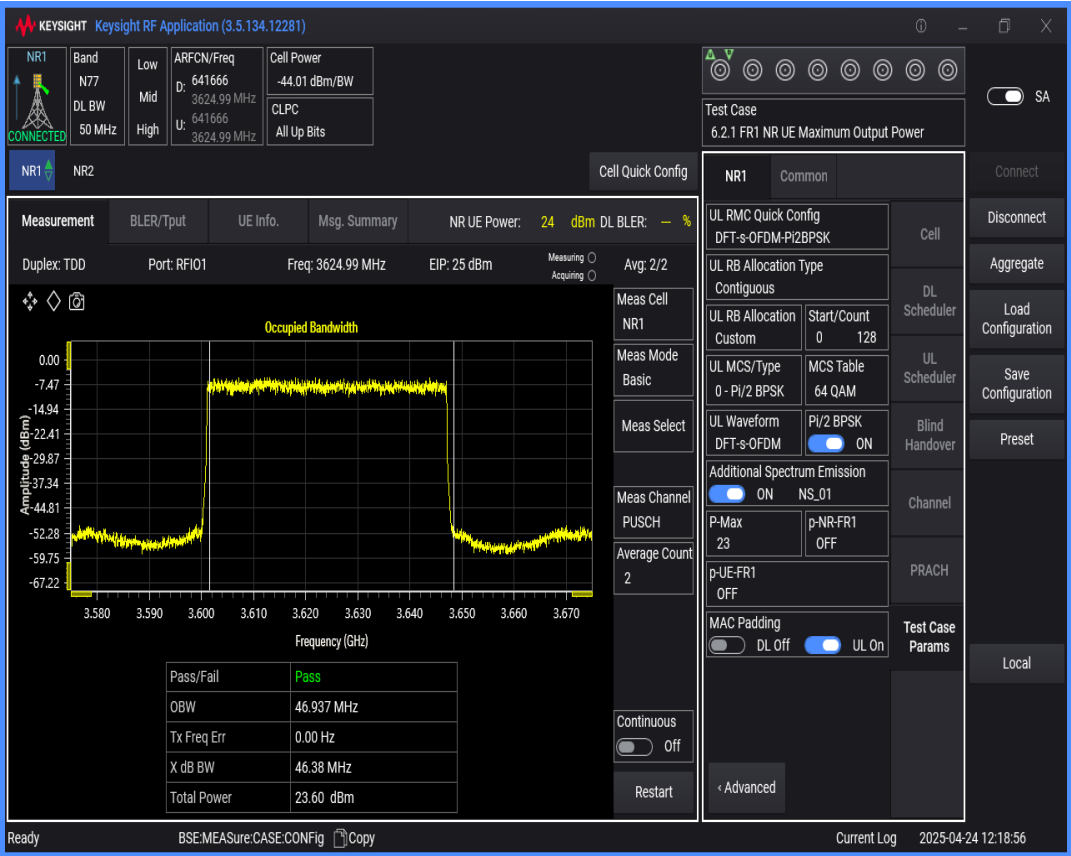
n77(3550-3700) SCS=30kHz DFT_BPSK BW=60MHz Channel=641666 RB=162@0
