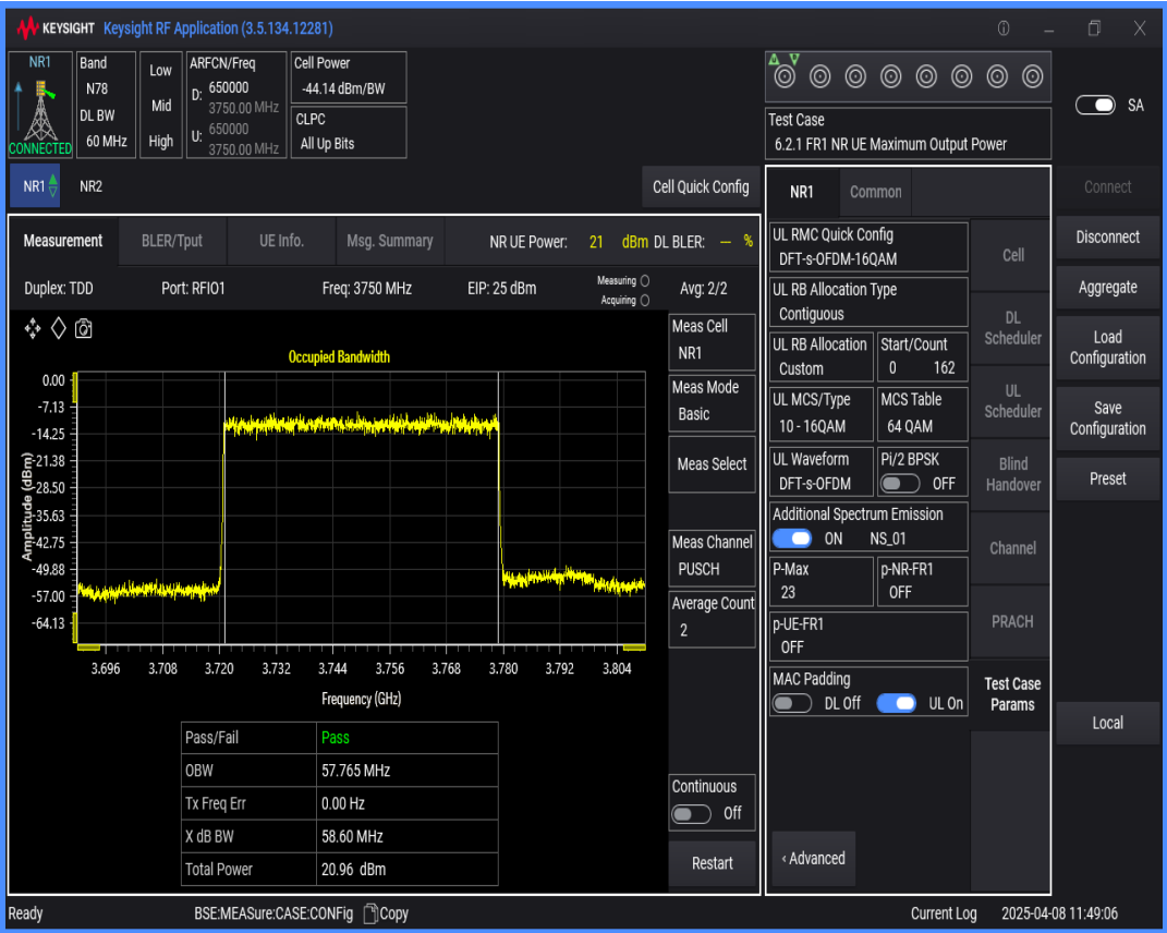
n78(3700-3800) SCS=30kHz DFT_QAM16 BW=80MHz Channel=650000 RB=216@0
