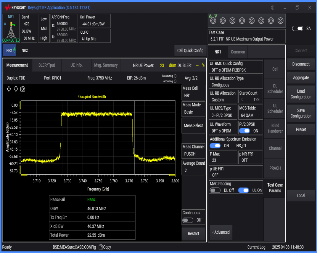
n78(3700-3800) SCS=30kHz DFT_BPSK BW=70MHz Channel=650000 RB=180@0
