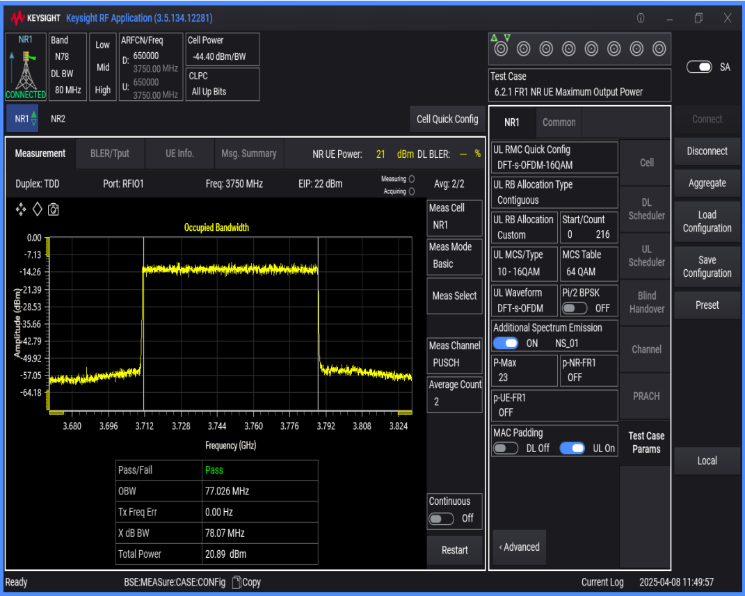
n78(3700-3800) SCS=30kHz DFT_QAM16 BW=90MHz Channel=650000 RB=240@0
