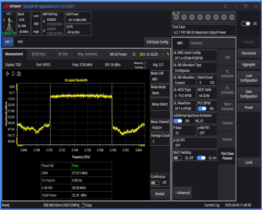
n78(3700-3800) SCS=30kHz DFT_BPSK BW=80MHz Channel=650000 RB=216@0
