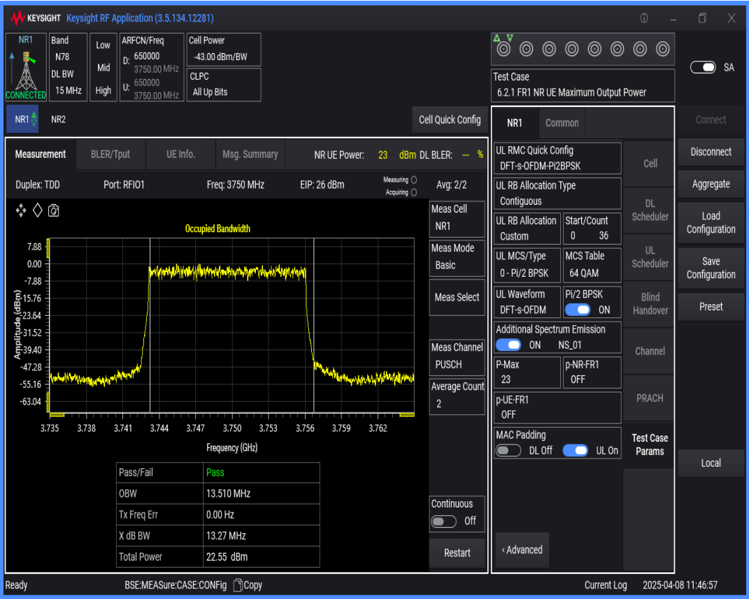
n78(3700-3800) SCS=30kHz DFT_BPSK BW=30MHz Channel=650000 RB=75@0
