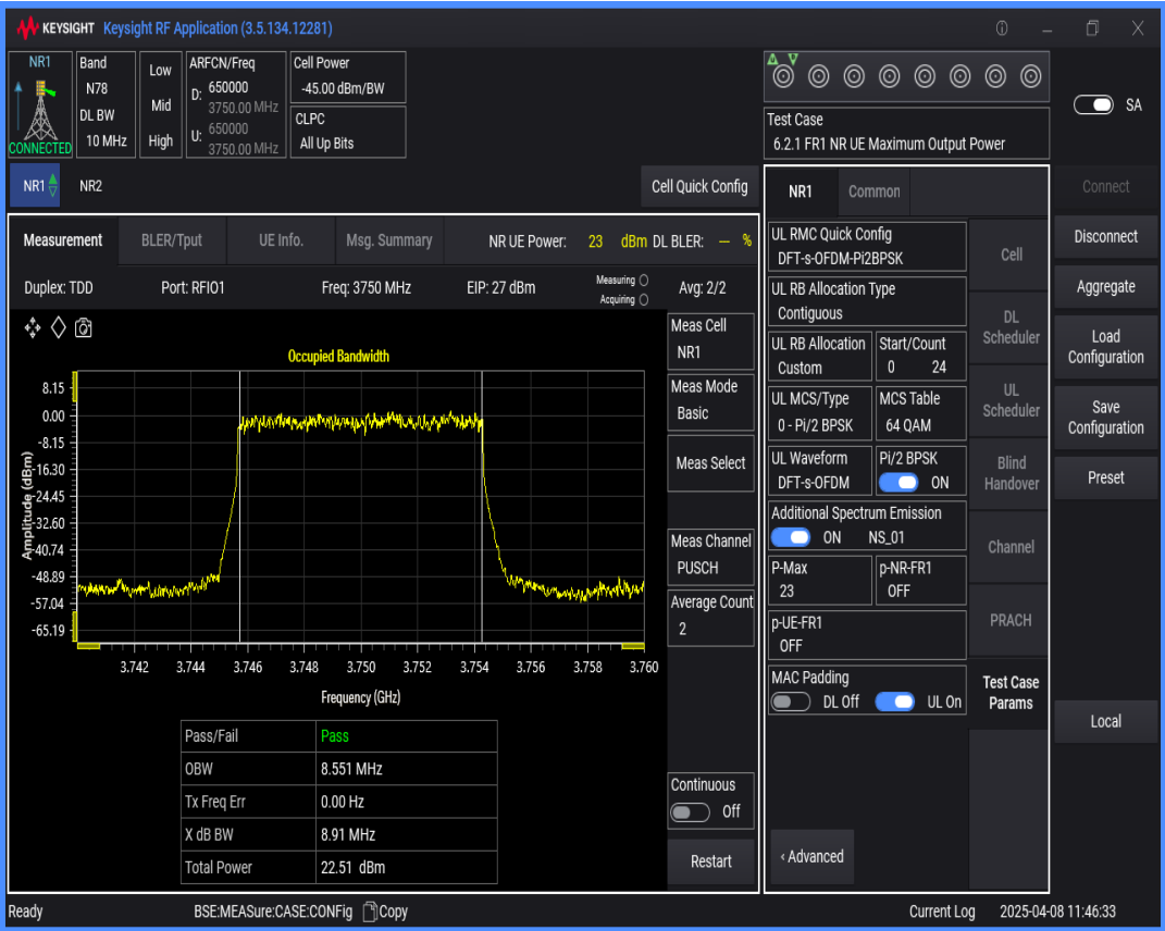
n78(3700-3800) SCS=30kHz DFT_BPSK BW=15MHz Channel=650000 RB=36@0
