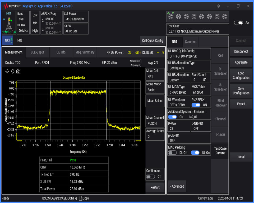
n78(3700-3800) SCS=30kHz DFT_BPSK BW=40MHz Channel=650000 RB=100@0
