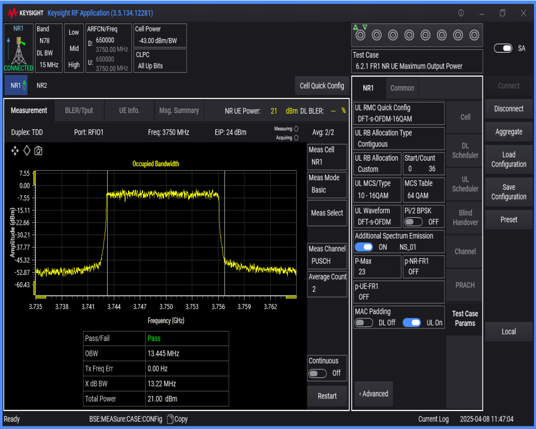
n78(3700-3800) SCS=30kHz DFT_QAM16 BW=30MHz Channel=650000 RB=75@0
