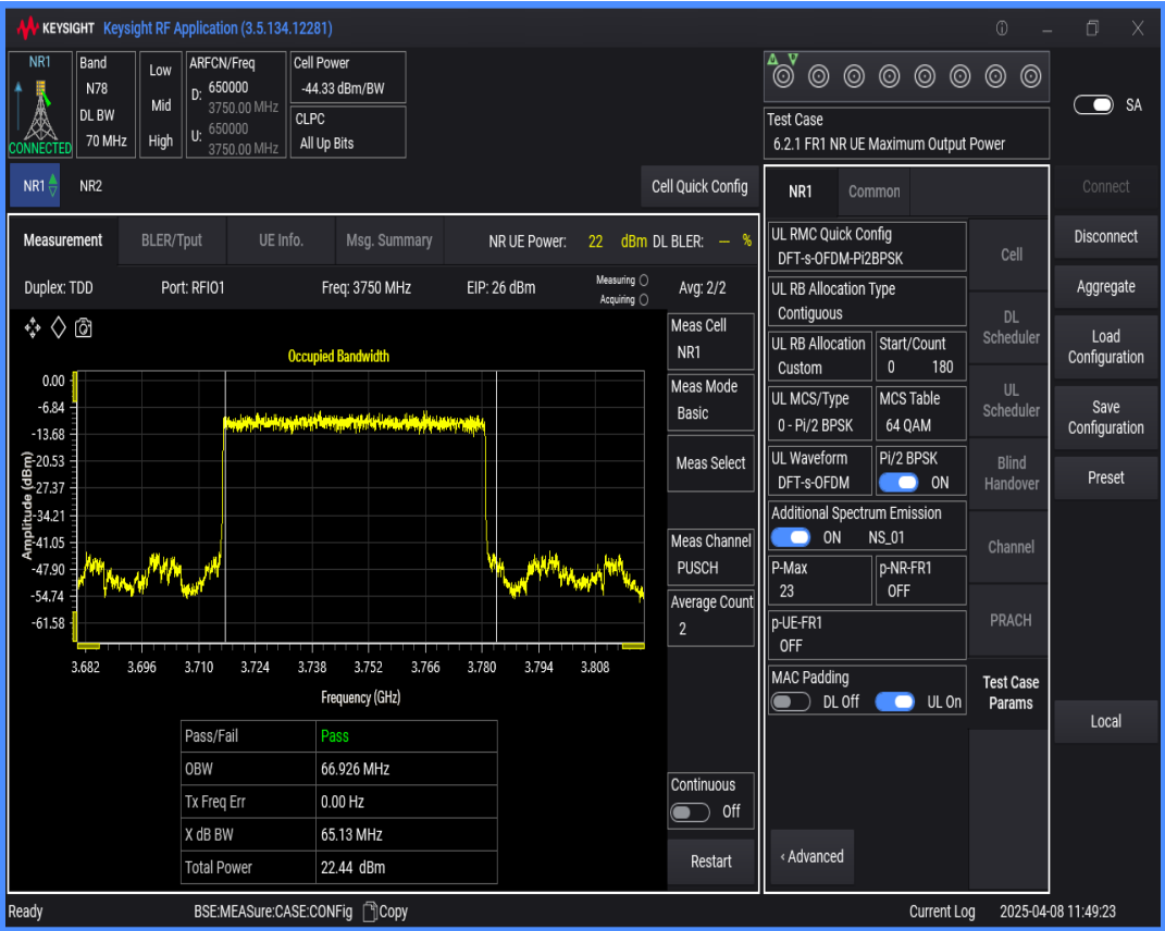
n78(3700-3800) SCS=30kHz DFT_BPSK BW=60MHz Channel=650000 RB=162@0
