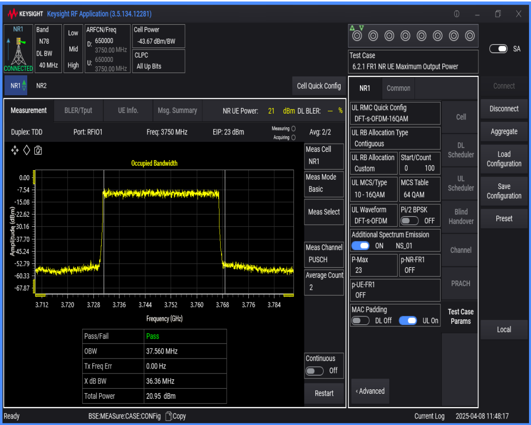
n78(3700-3800) SCS=30kHz DFT_QAM16 BW=50MHz Channel=650000 RB=128@0
