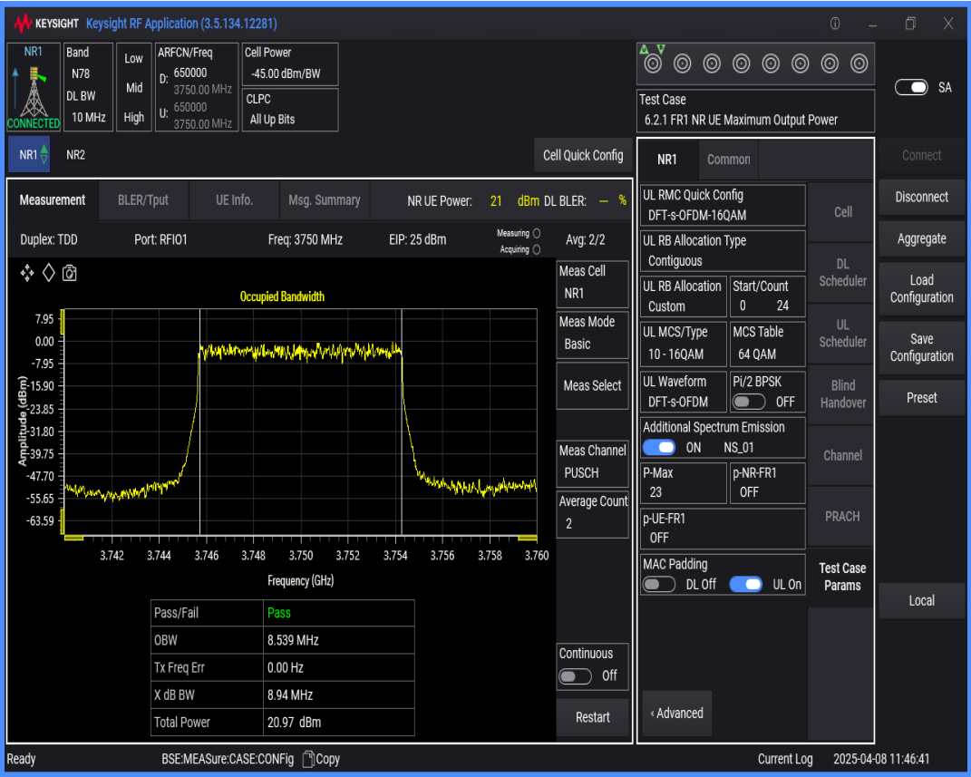
n78(3700-3800) SCS=30kHz DFT_QAM16 BW=20MHz Channel=650000 RB=50@0
