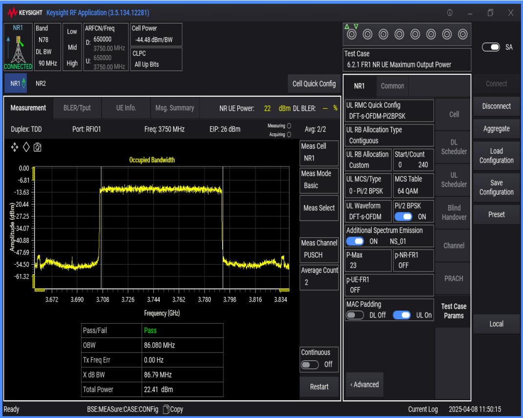
n78(3700-3800) SCS=30kHz DFT_QAM16 BW=10MHz Channel=650000 RB=24@0
