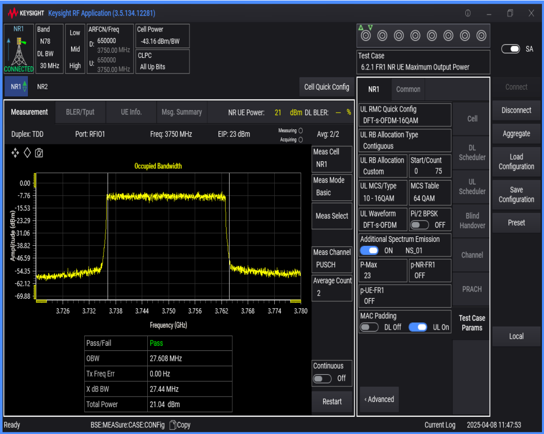
n78(3700-3800) SCS=30kHz DFT_QAM16 BW=40MHz Channel=650000 RB=100@0
