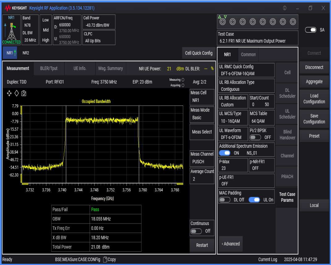
n78(3700-3800) SCS=30kHz DFT_QAM16 BW=15MHz Channel=650000 RB=36@0
