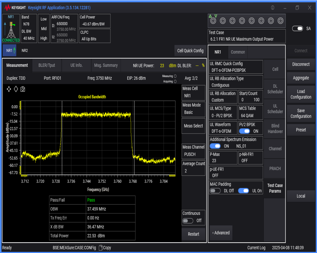
n78(3700-3800) SCS=30kHz DFT_BPSK BW=50MHz Channel=650000 RB=128@0
