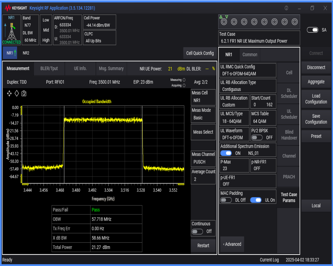
n77(3450-3550) SCS=30kHz DFT_QAM64 BW=50MHz Channel=633334 RB=128@0
