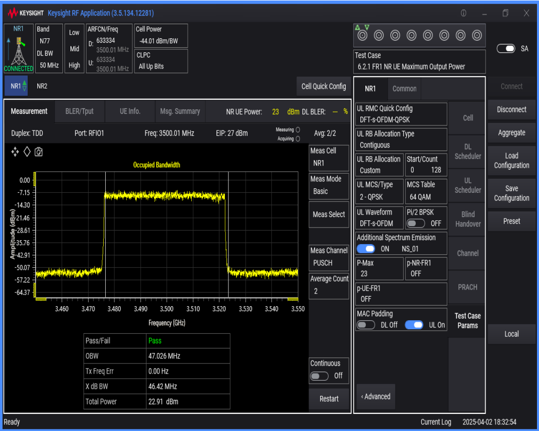
n77(3450-3550) SCS=30kHz DFT_QPSK BW=40MHz Channel=633334 RB=100@0
