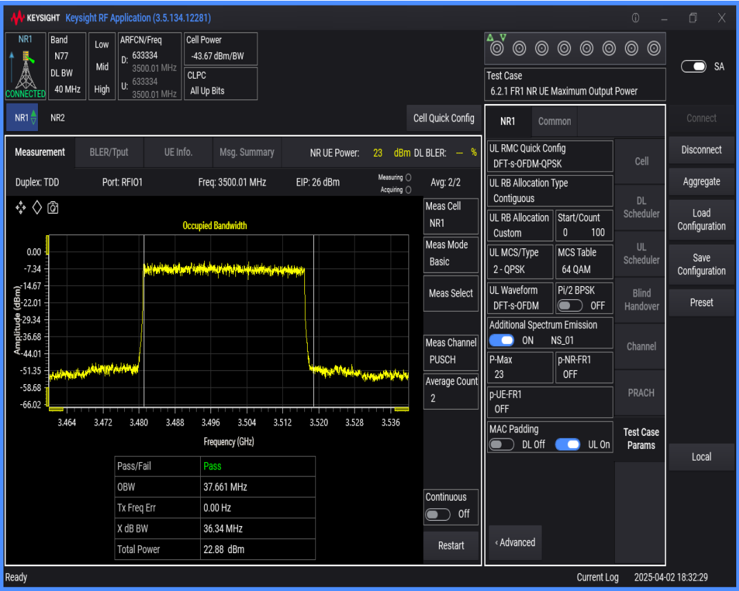
n77(3450-3550) SCS=30kHz DFT_QPSK BW=60MHz Channel=633334 RB=162@0
