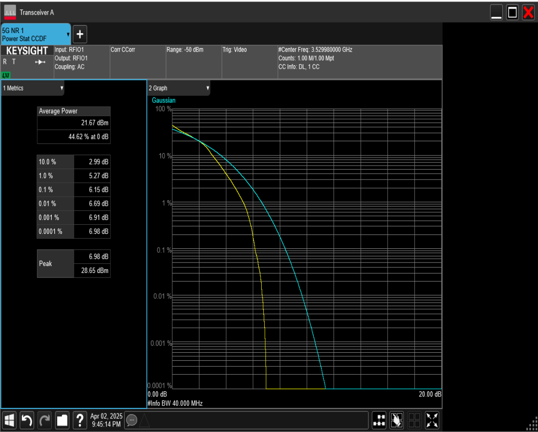
n77(3450-3550) SCS=30kHz DFT_QAM16 BW=50MHz Channel=635000 RB=128@0
