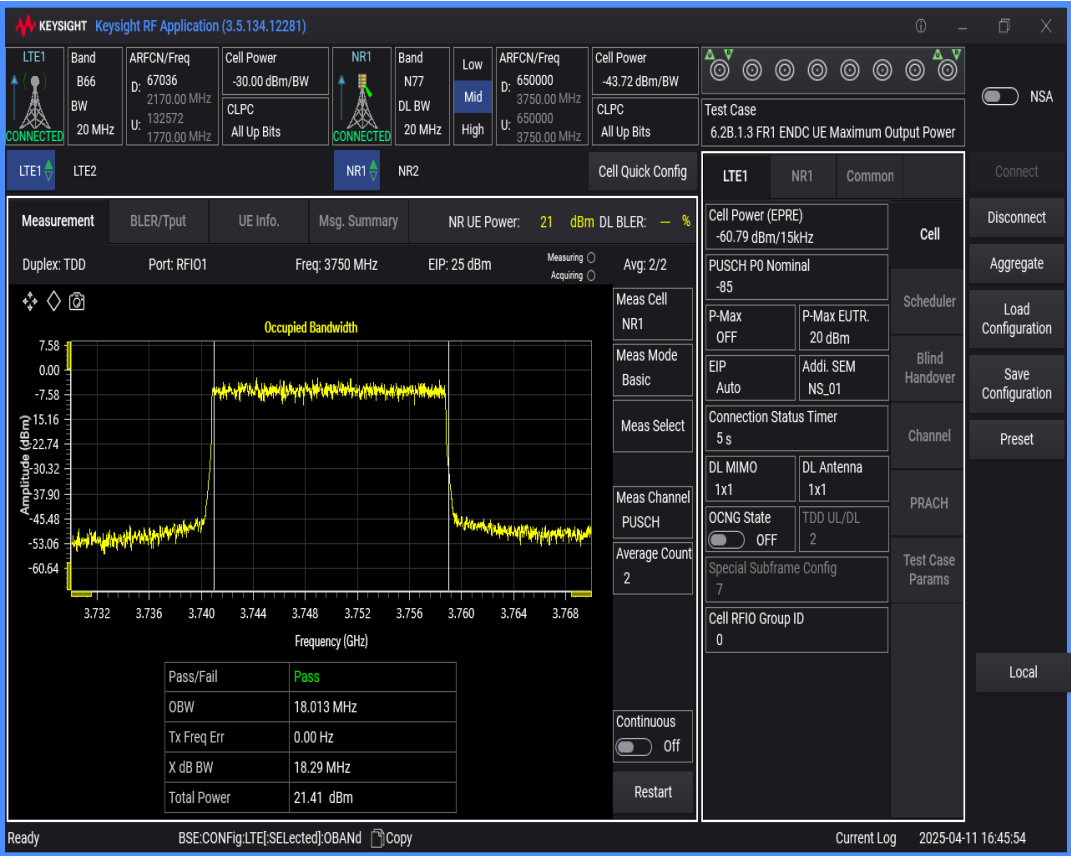
n77 SCS=30kHz DFT_QAM64 BW=50MHz Channel=650000 RB=128@0
