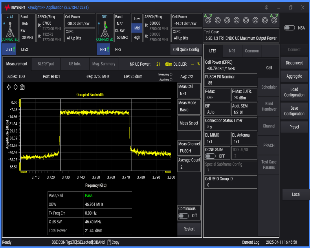
n77 SCS=30kHz DFT_QAM64 BW=80MHz Channel=650000 RB=216@0
