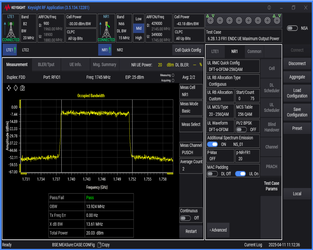
n66 SCS=15kHz DFT_QAM16 BW=15MHz Channel=349000 RB=75@0
