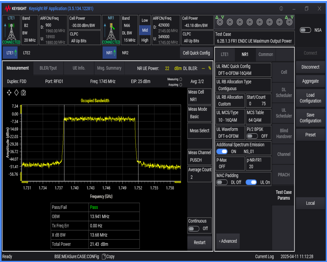
n66 SCS=15kHz DFT_QAM16 BW=20MHz Channel=349000 RB=100@0
