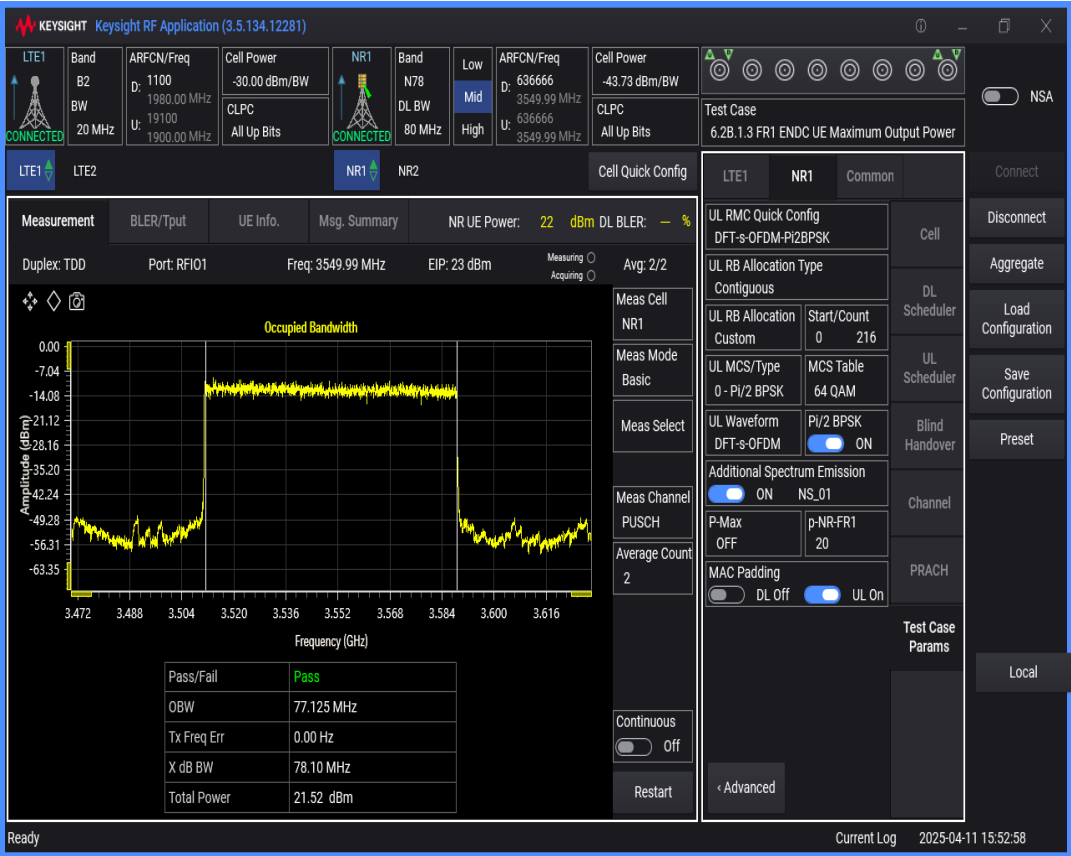
n78 SCS=30kHz DFT_BPSK BW=90MHz Channel=636666 RB=240@0
