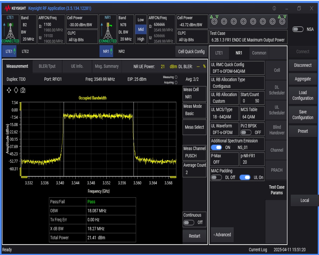
n78 SCS=30kHz DFT_QAM64 BW=15MHz Channel=636666 RB=36@0
