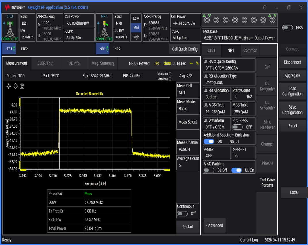
n78 SCS=30kHz DFT_QAM64 BW=80MHz Channel=636666 RB=216@0
