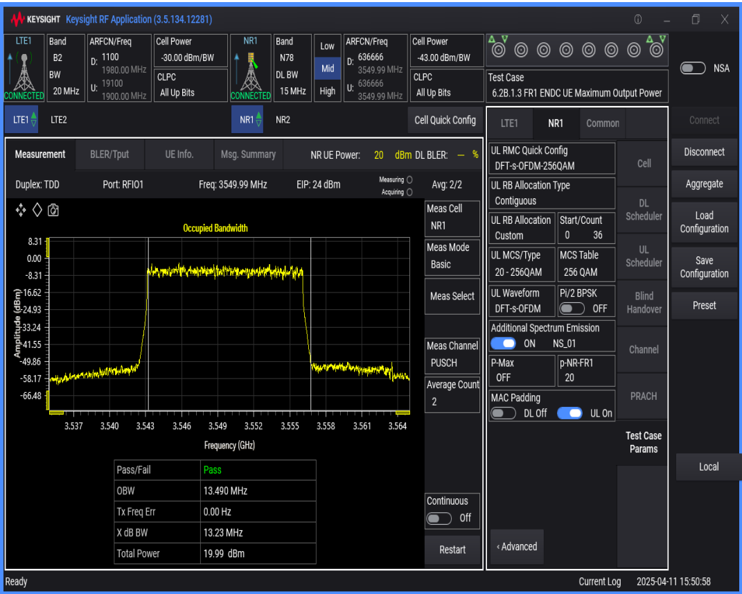
n78 SCS=30kHz DFT_QAM256 BW=10MHz Channel=636666 RB=24@0
