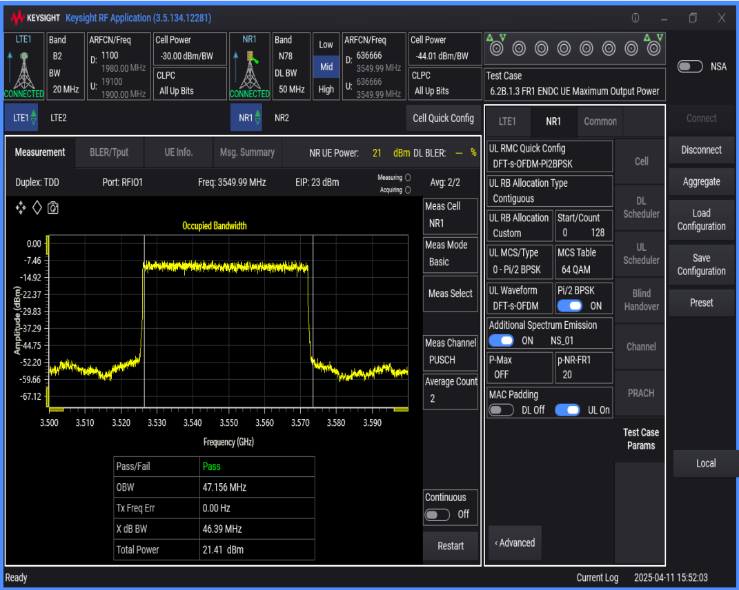
n78 SCS=30kHz DFT_BPSK BW=60MHz Channel=636666 RB=162@0
