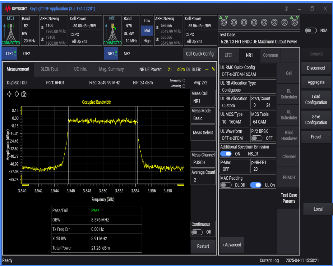
n78 SCS=30kHz DFT_QAM16 BW=80MHz Channel=636666 RB=216@0
