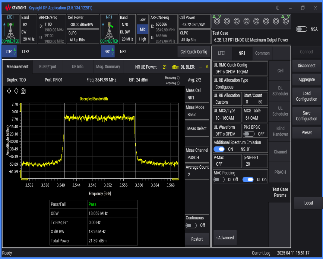
n78 SCS=30kHz DFT_QAM16 BW=100MHz Channel=636666 RB=270@0
