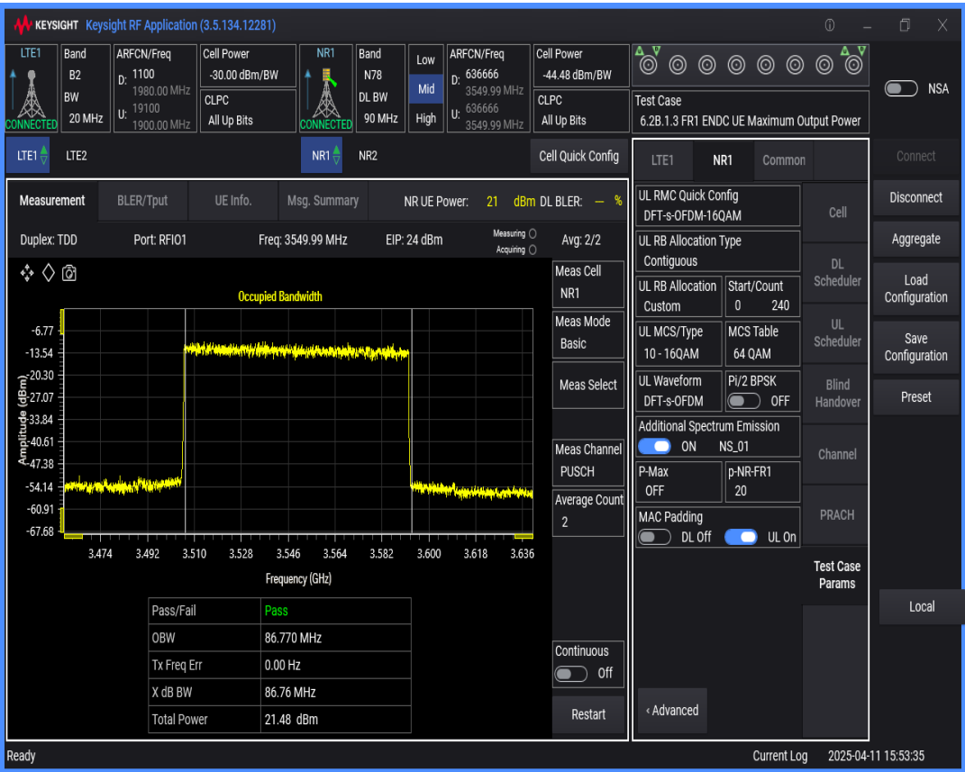
n78 SCS=30kHz DFT_QAM16 BW=60MHz Channel=636666 RB=162@0
