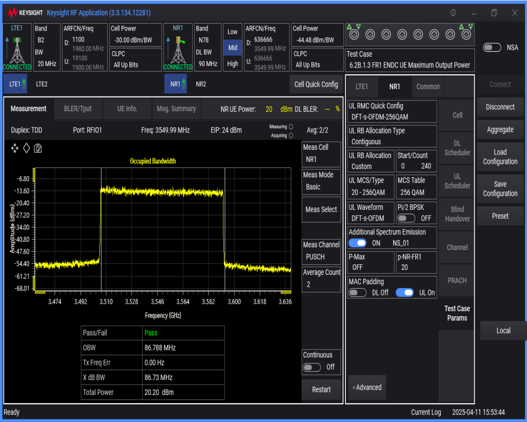
n78 SCS=30kHz DFT_QAM256 BW=50MHz Channel=636666 RB=128@0
