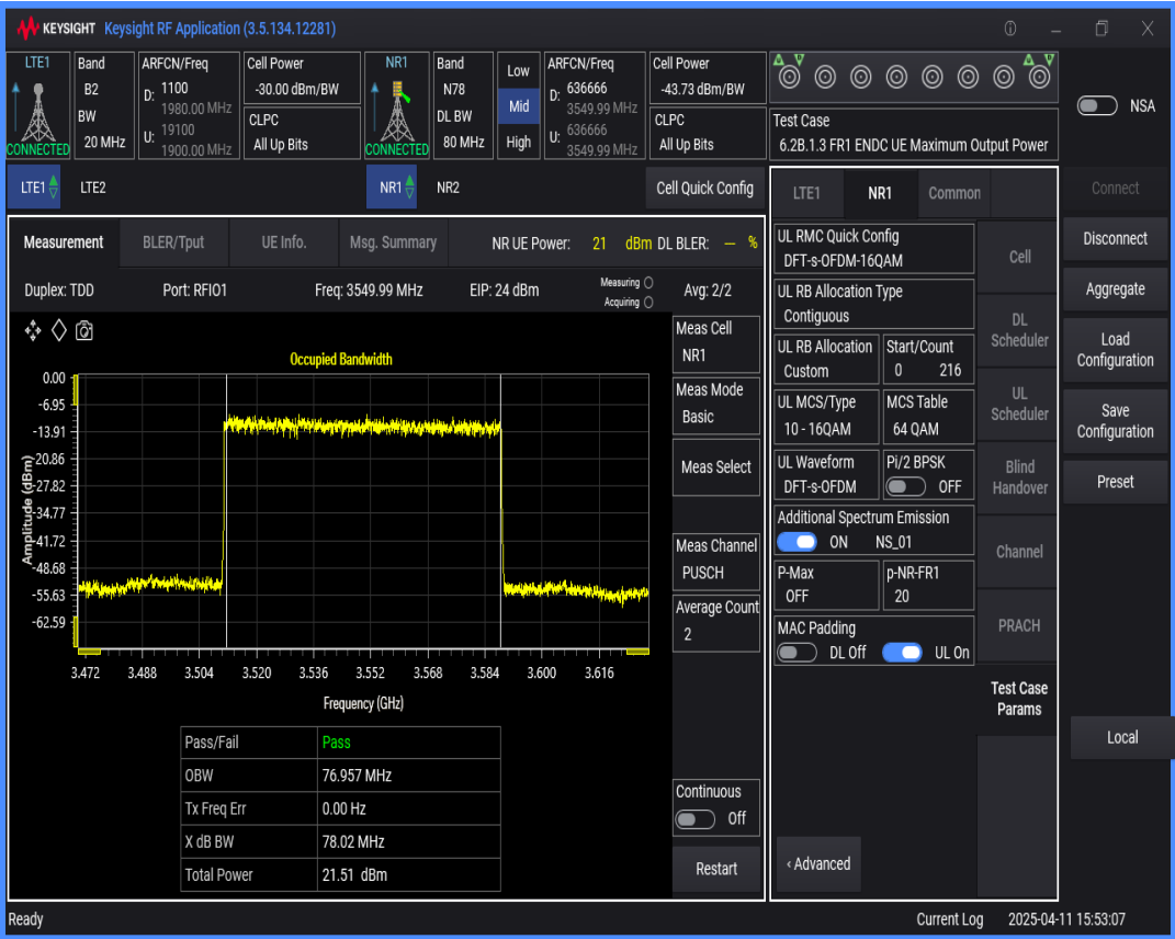
n78 SCS=30kHz DFT_QAM16 BW=90MHz Channel=636666 RB=240@0
