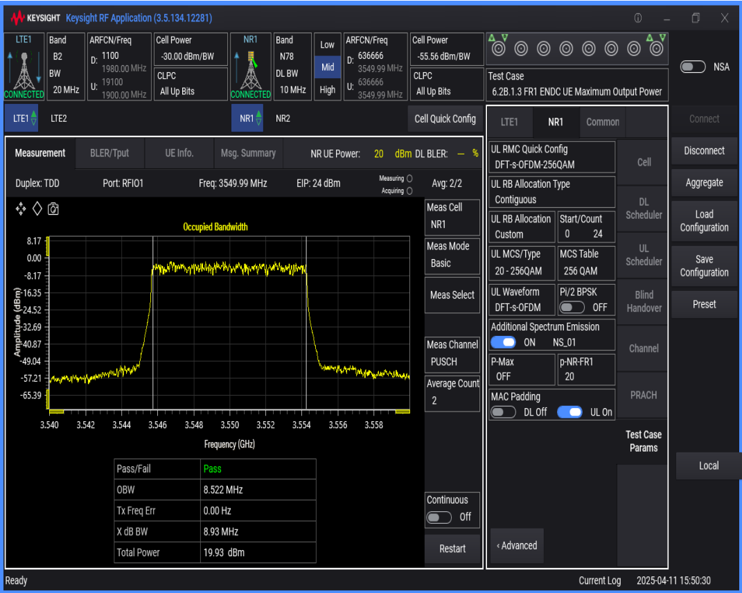
n78 SCS=30kHz DFT_QAM256 BW=100MHz Channel=636666 RB=270@0
