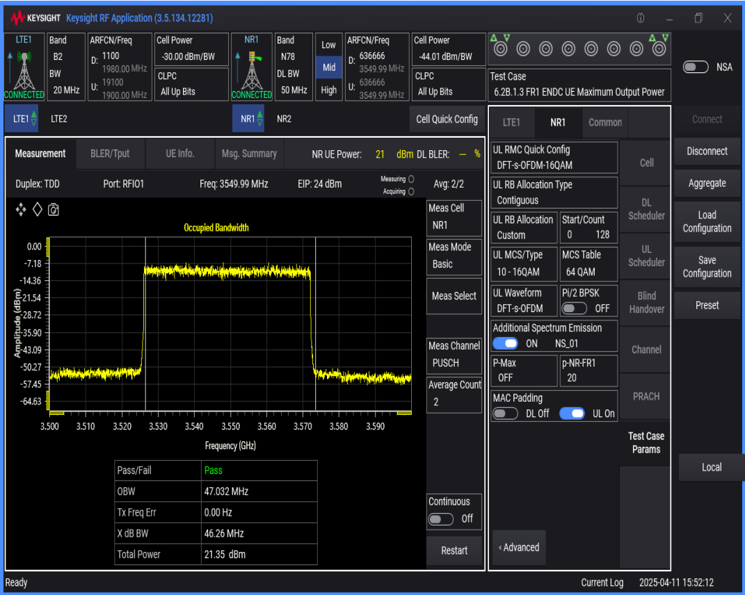
n78 SCS=30kHz DFT_QAM256 BW=15MHz Channel=636666 RB=36@0
