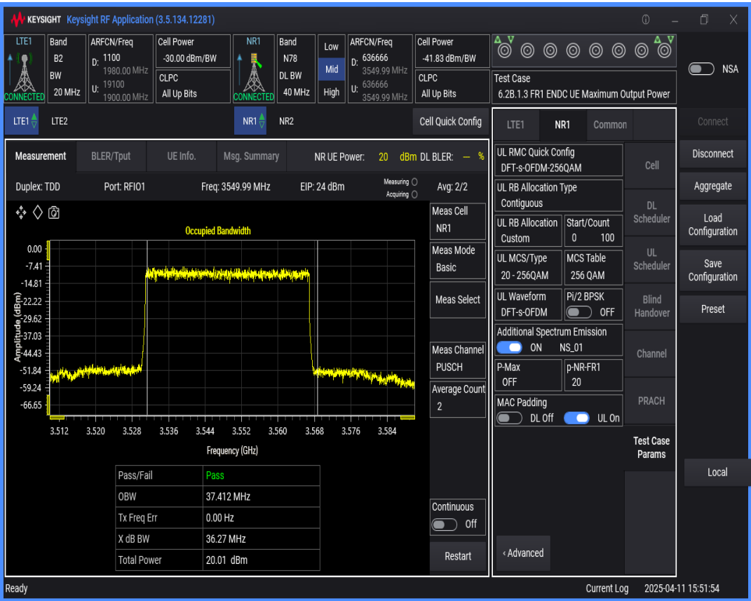
n78 SCS=30kHz DFT_QAM256 BW=80MHz Channel=636666 RB=216@0
