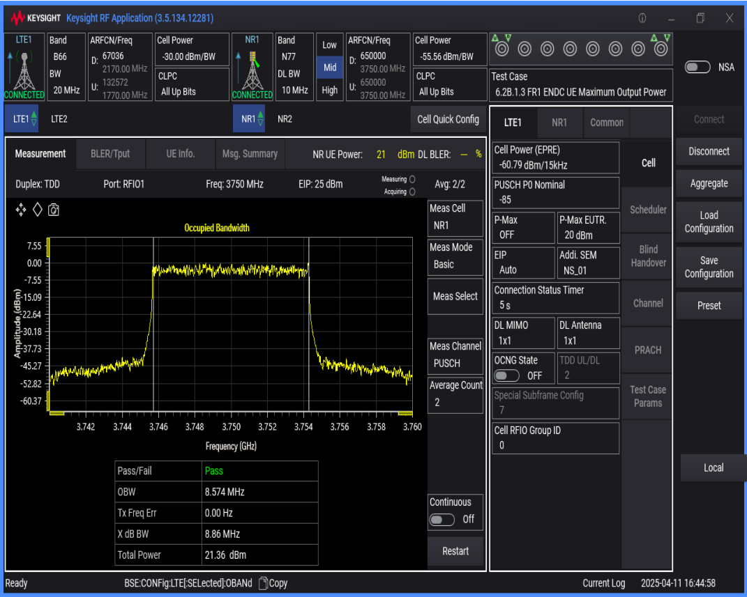
n77 SCS=30kHz DFT_QAM256 BW=80MHz Channel=650000 RB=216@0
