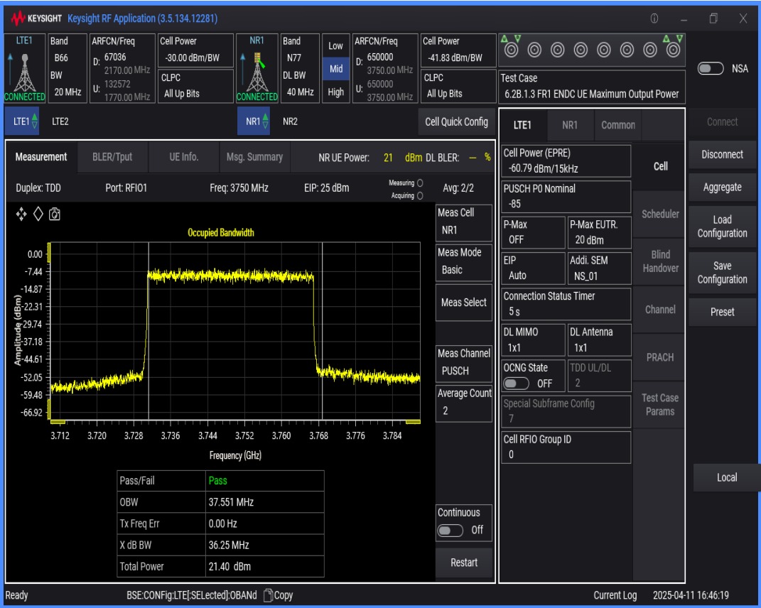
n77 SCS=30kHz DFT_QAM16 BW=20MHz Channel=650000 RB=50@0
