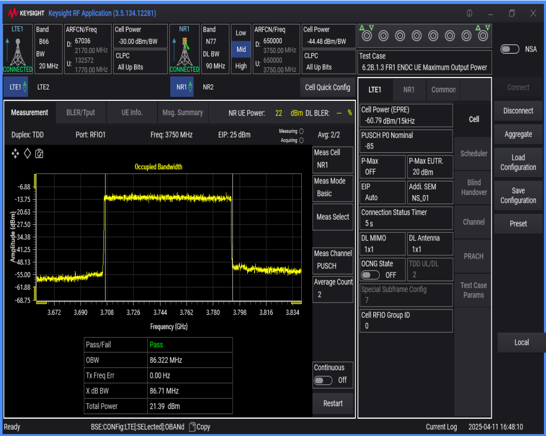
n77 SCS=30kHz DFT_QAM64 BW=20MHz Channel=650000 RB=50@0
