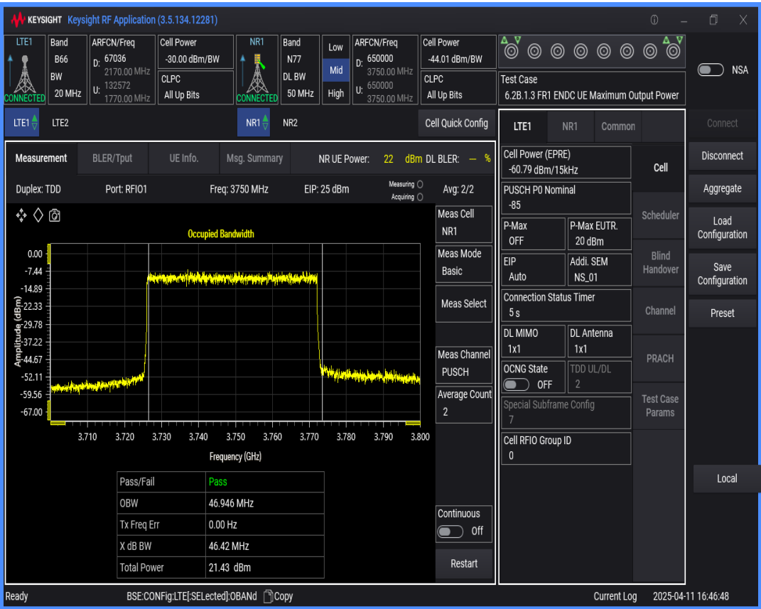
n77 SCS=30kHz DFT_QAM16 BW=80MHz Channel=650000 RB=216@0
