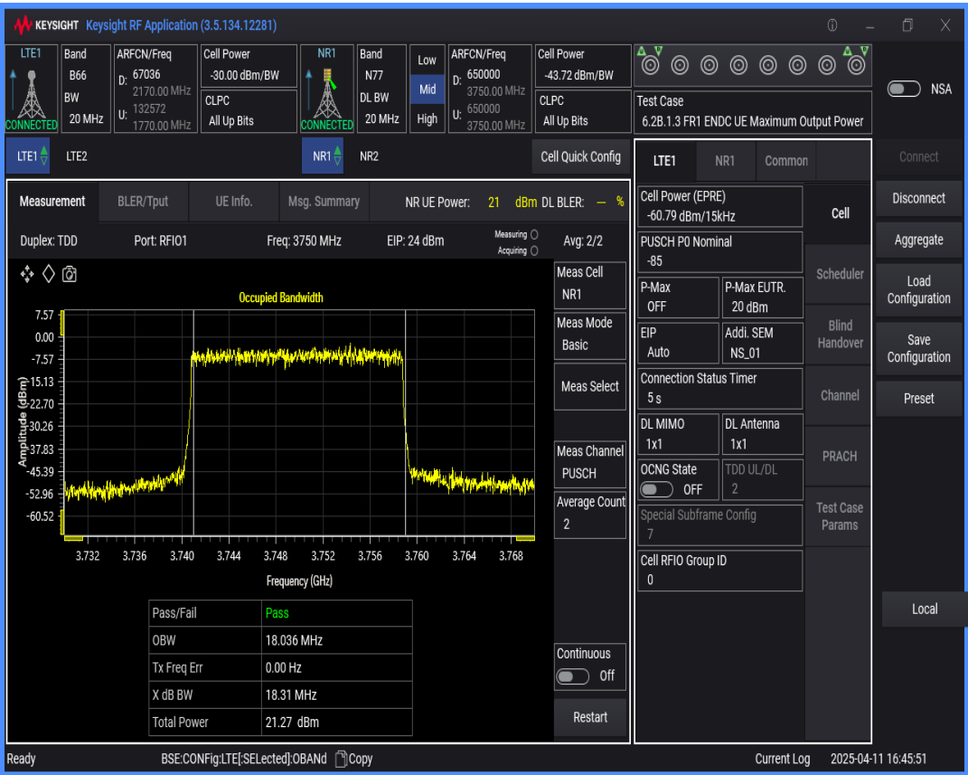
n77 SCS=30kHz DFT_BPSK BW=50MHz Channel=650000 RB=128@0
