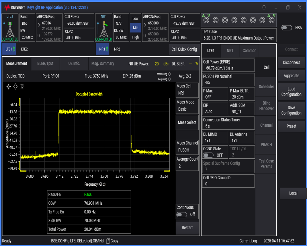
n77 SCS=30kHz DFT_QAM256 BW=60MHz Channel=650000 RB=162@0
