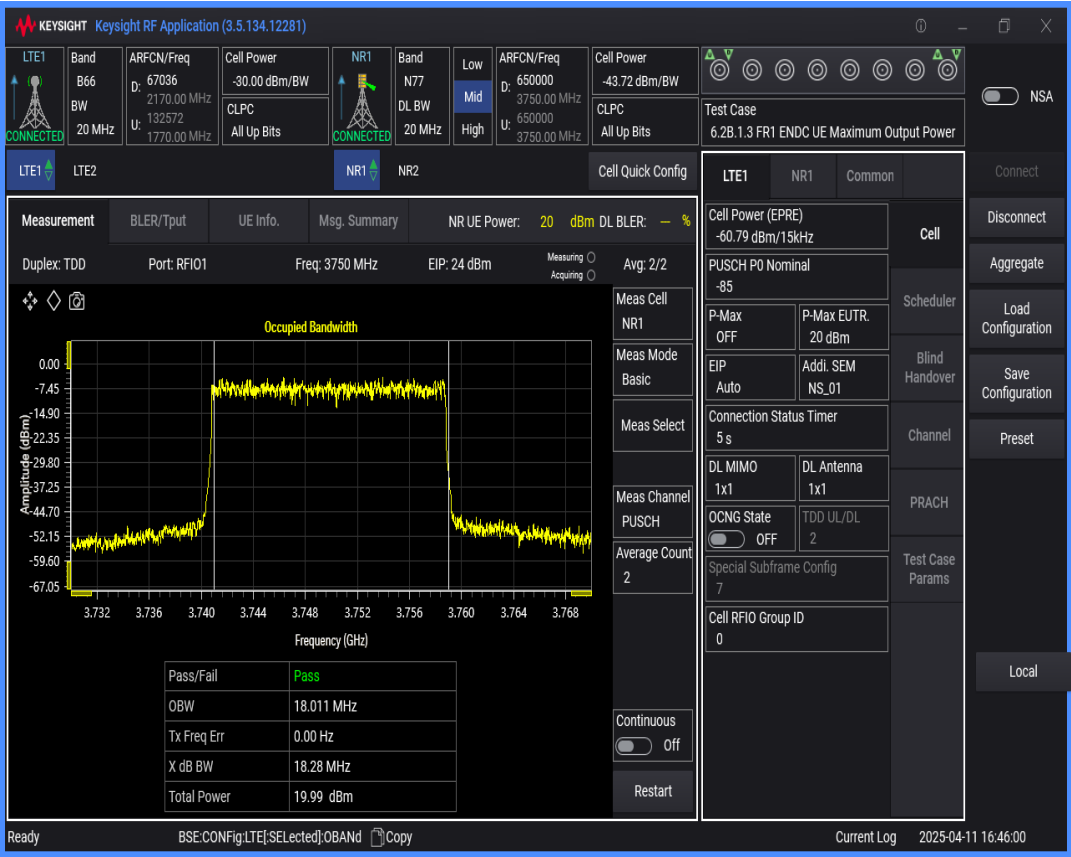
n77 SCS=30kHz DFT_QAM256 BW=50MHz Channel=650000 RB=128@0
