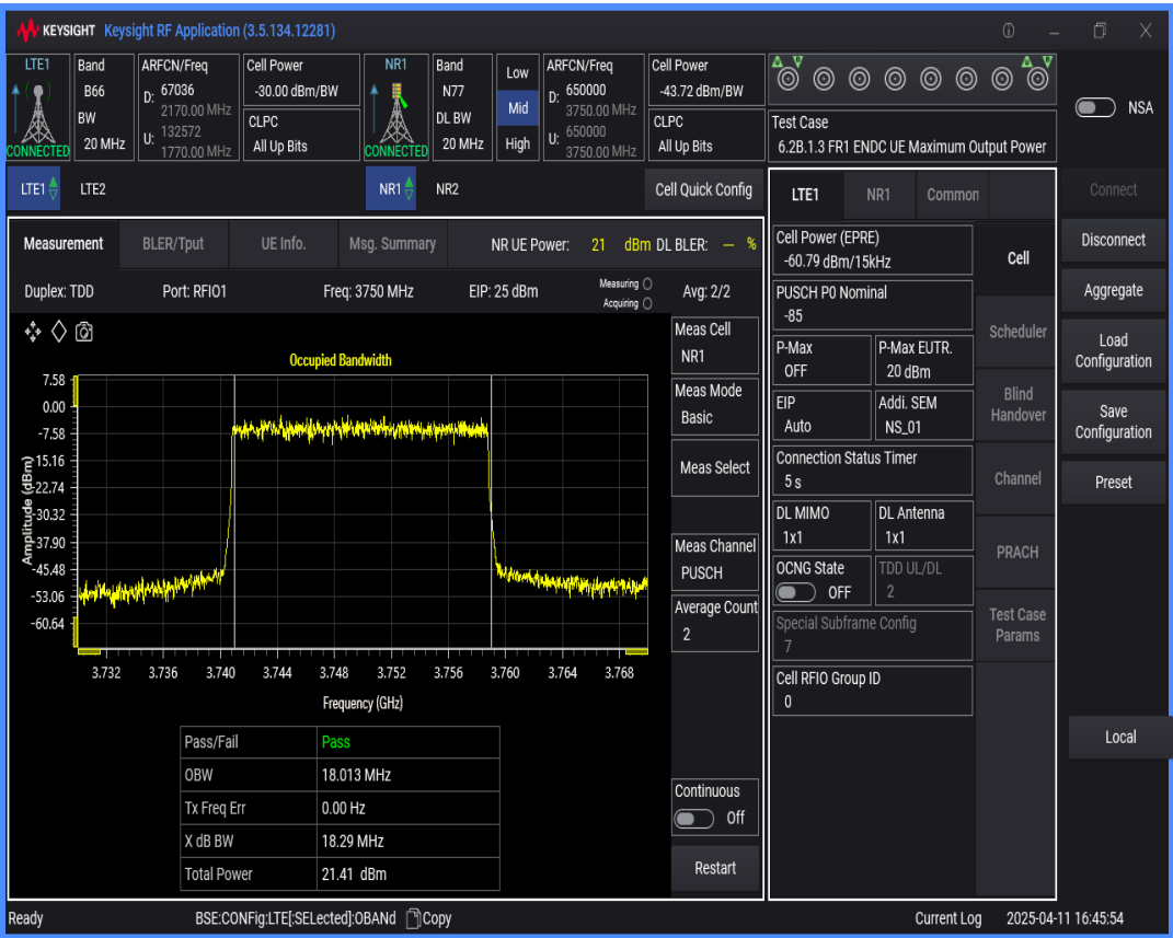
n77 SCS=30kHz DFT_QAM64 BW=15MHz Channel=650000 RB=36@0
