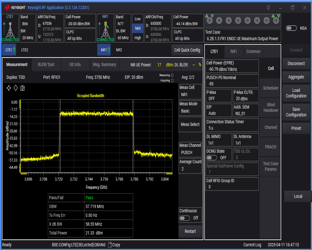
n77 SCS=30kHz DFT_QAM16 BW=50MHz Channel=650000 RB=128@0
