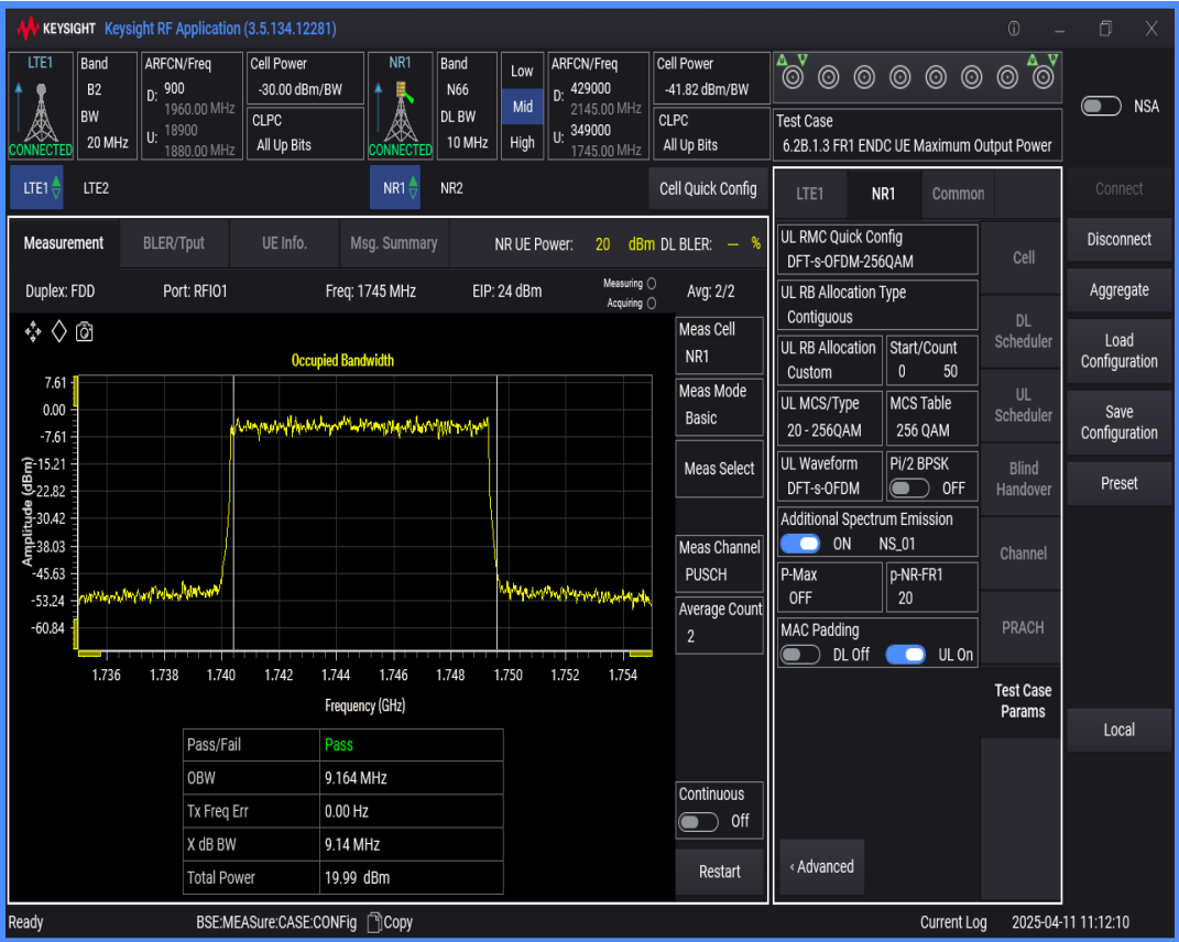
n66 SCS=15kHz DFT_QAM16 BW=20MHz Channel=349000 RB=100@0
