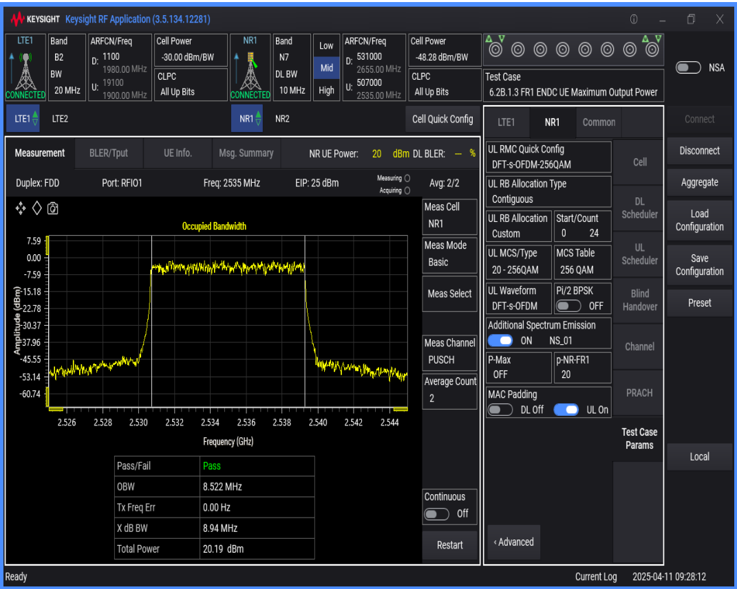
n7 SCS=30kHz DFT_QAM256 BW=15MHz Channel=507000 RB=36@0
