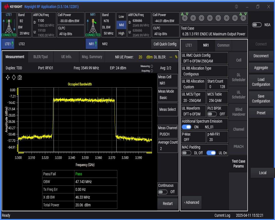
n78 SCS=30kHz DFT_QAM256 BW=60MHz Channel=636666 RB=162@0
