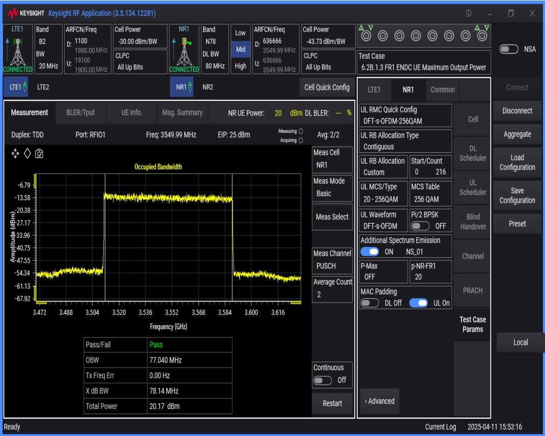
n78 SCS=30kHz DFT_QAM256 BW=90MHz Channel=636666 RB=240@0
