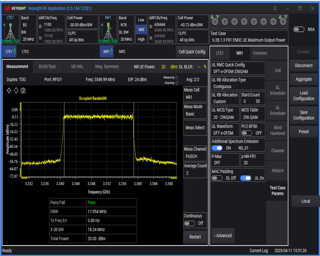
n78 SCS=30kHz DFT_QAM256 BW=40MHz Channel=636666 RB=100@0
