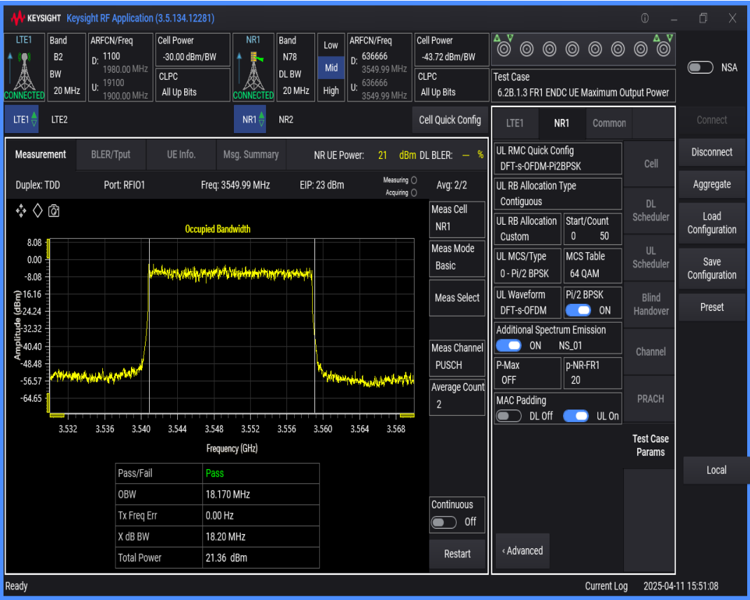
n78 SCS=30kHz DFT_BPSK BW=40MHz Channel=636666 RB=100@0
