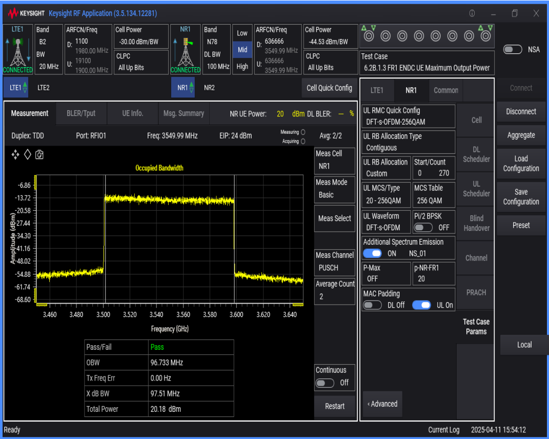
n78 SCS=30kHz DFT_QAM256 BW=10MHz Channel=636666 RB=24@0
