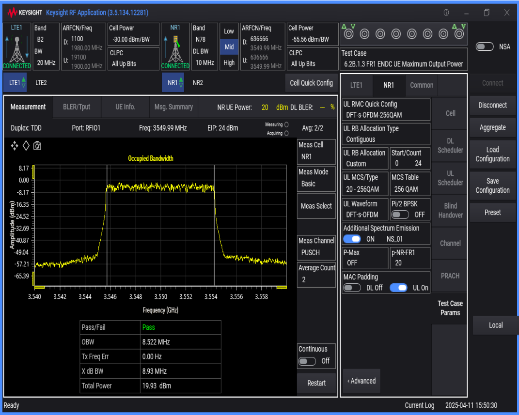
n78 SCS=30kHz DFT_QAM256 BW=80MHz Channel=636666 RB=216@0
