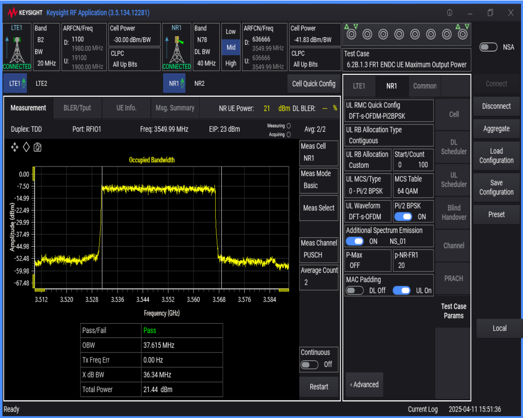
n78 SCS=30kHz DFT_QAM16 BW=50MHz Channel=636666 RB=128@0
