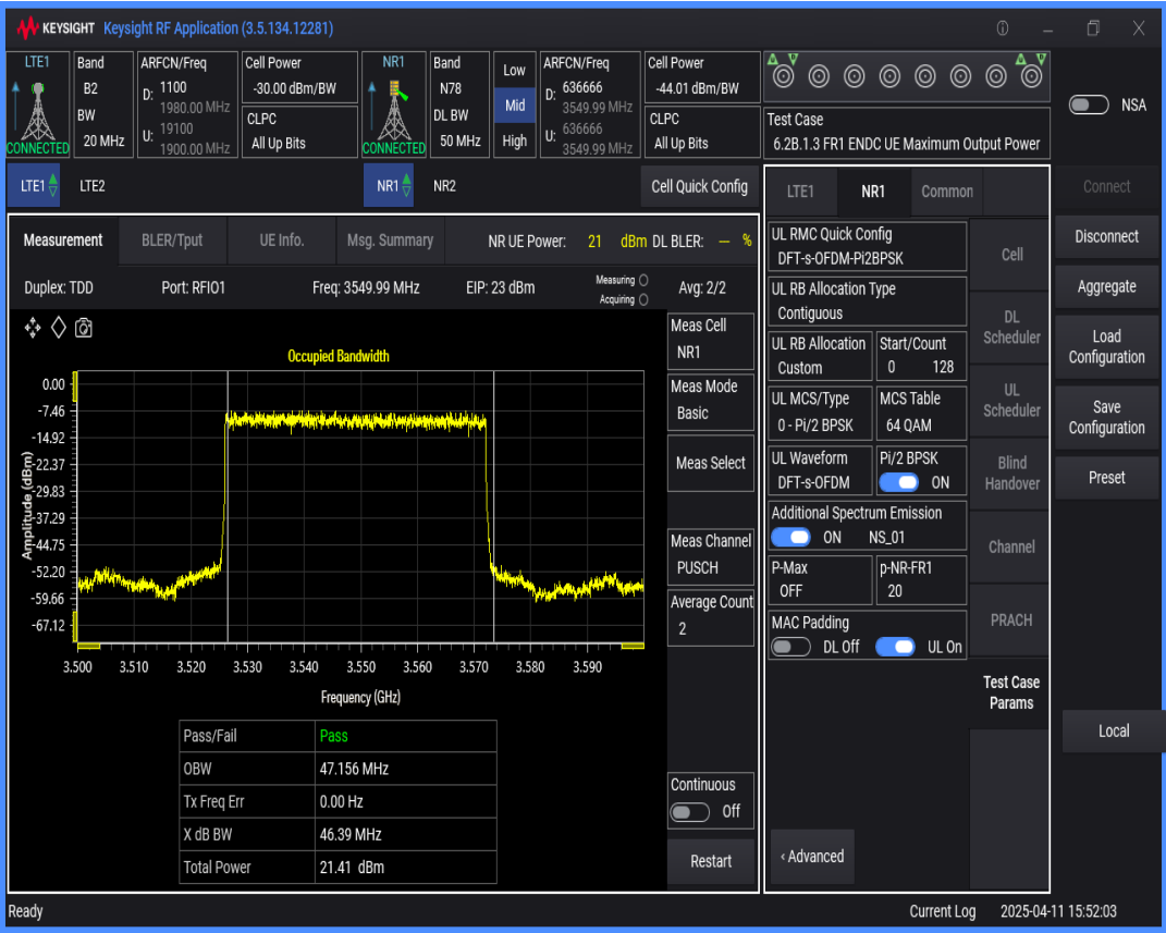
n78 SCS=30kHz DFT_BPSK BW=60MHz Channel=636666 RB=162@0
