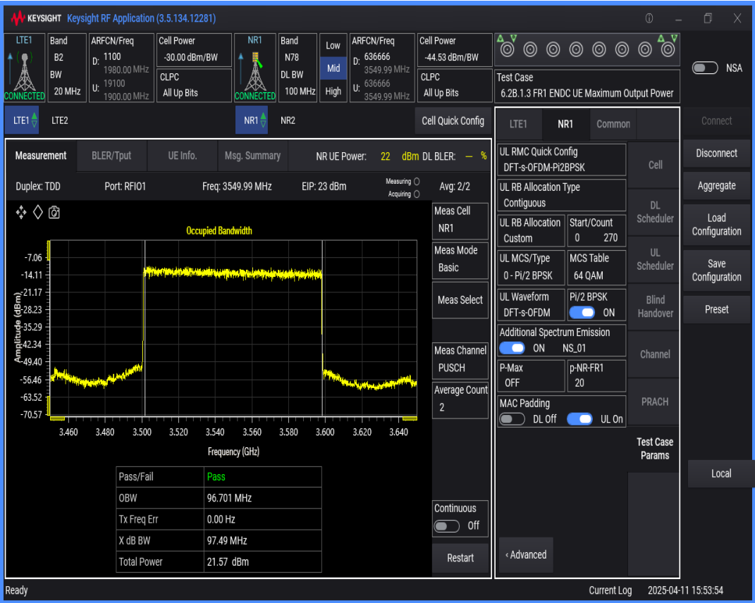
n78 SCS=30kHz DFT_BPSK BW=50MHz Channel=636666 RB=128@0
