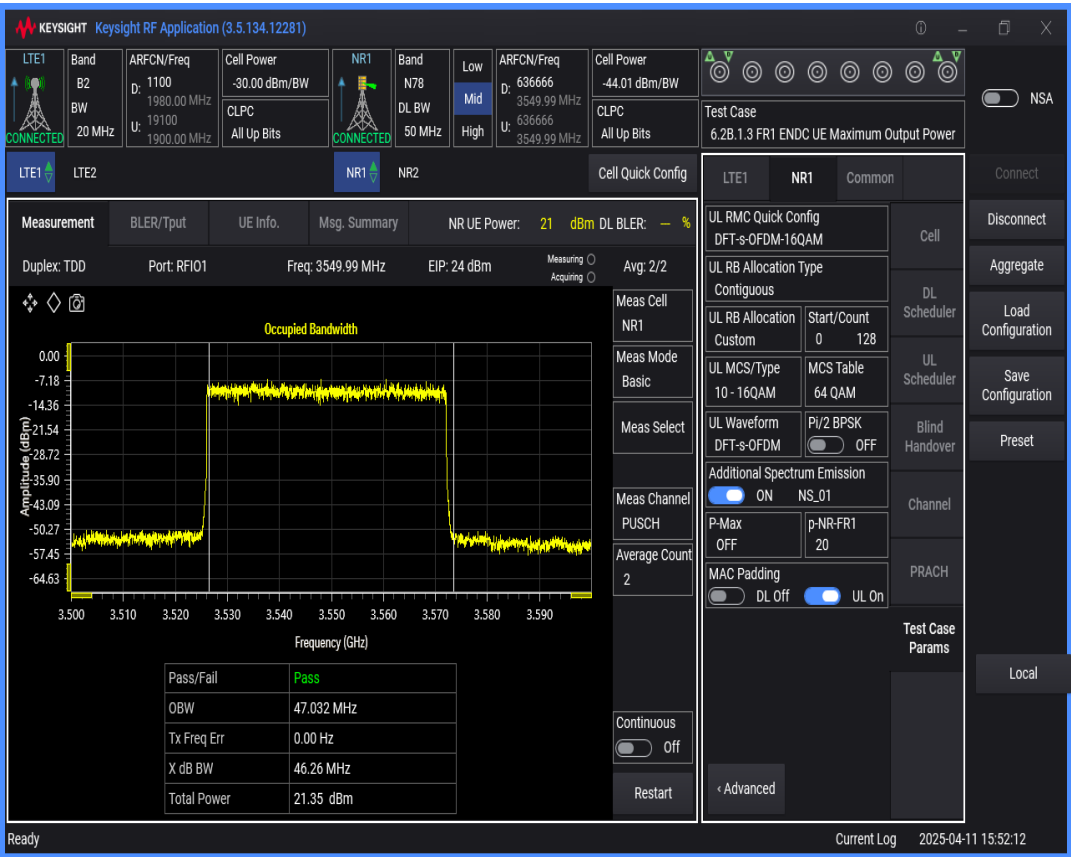
n78 SCS=30kHz DFT_QAM16 BW=40MHz Channel=636666 RB=100@0
