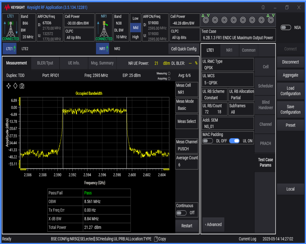
n38 SCS=30kHz DFT_BPSK BW=15MHz Channel=519000 RB=36@0
