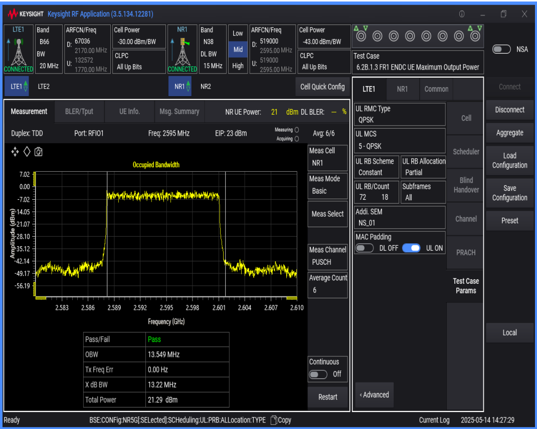
n38 SCS=30kHz DFT_QAM64 BW=10MHz Channel=519000 RB=24@0
