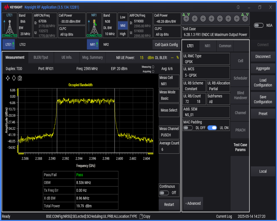
n38 SCS=30kHz DFT_QAM256 BW=15MHz Channel=519000 RB=36@0
