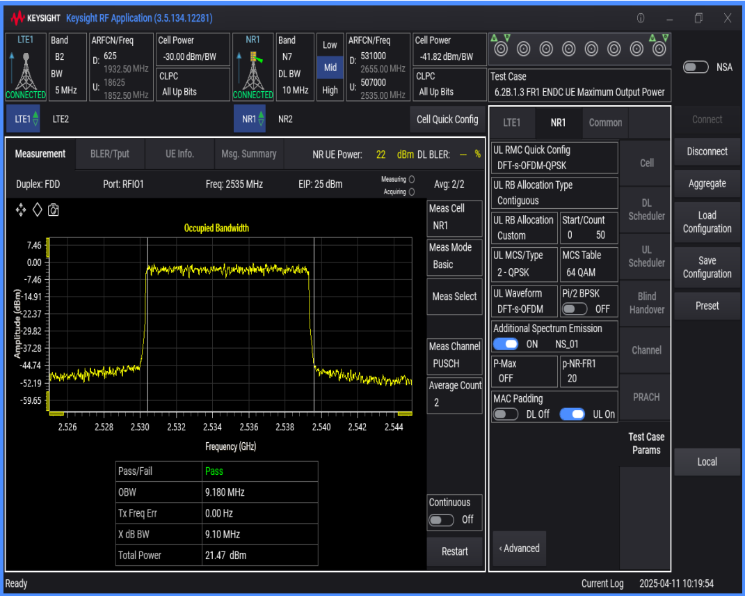
n7 SCS=30kHz DFT_BPSK BW=15MHz Channel=507000 RB=36@0
