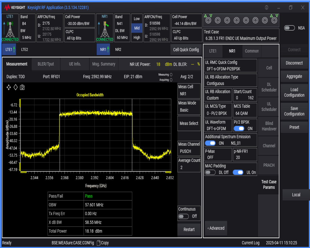
n41 SCS=30kHz DFT_BPSK BW=50MHz Channel=518598 RB=128@0
