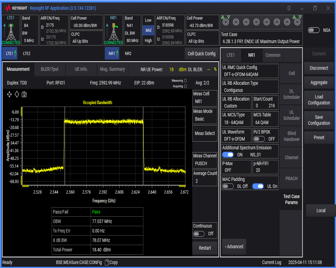
n41 SCS=30kHz DFT_QPSK BW=100MHz Channel=518598 RB=270@0
