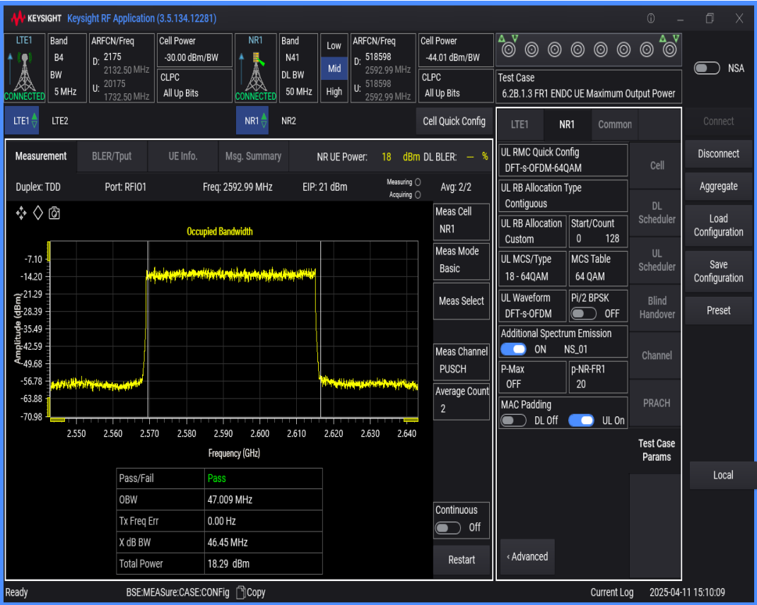
n41 SCS=30kHz DFT_QPSK BW=80MHz Channel=518598 RB=216@0
