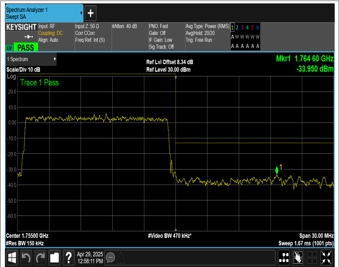
Band4 QPSK BW=15MHz Channel=20325 RB Size=75 Position=#0
