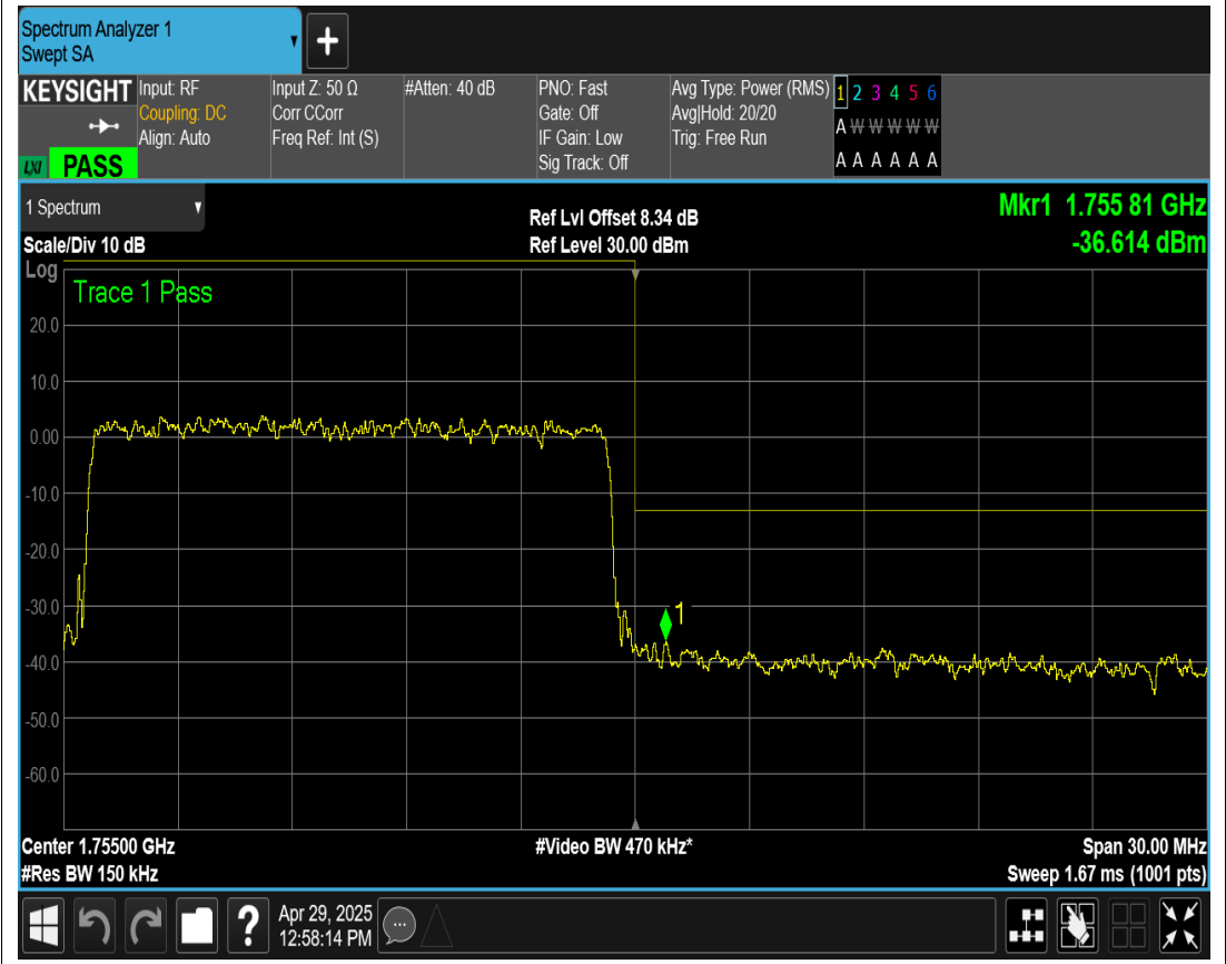
Band4 16QAM BW=15MHz Channel=20325 RB Size=75 Position=#0
