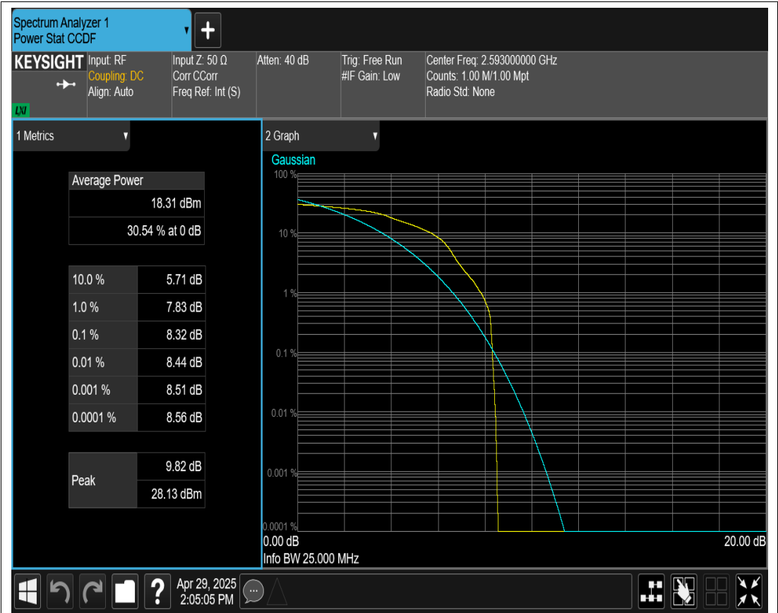
Band41 16QAM BW=15MHz Channel=40620 RB Size=1 Position=#0
