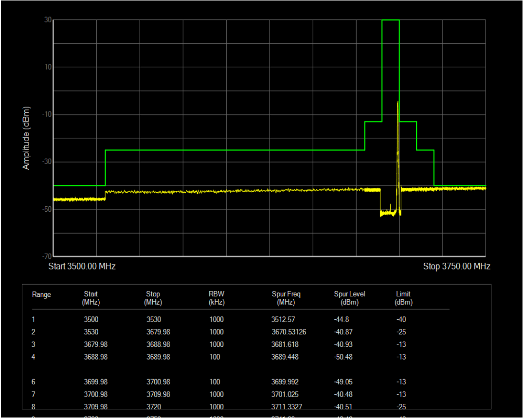
n78(3550-3700) SCS=30kHz CP_QPSK BW=50MHz Channel=638334 RB=133@0
