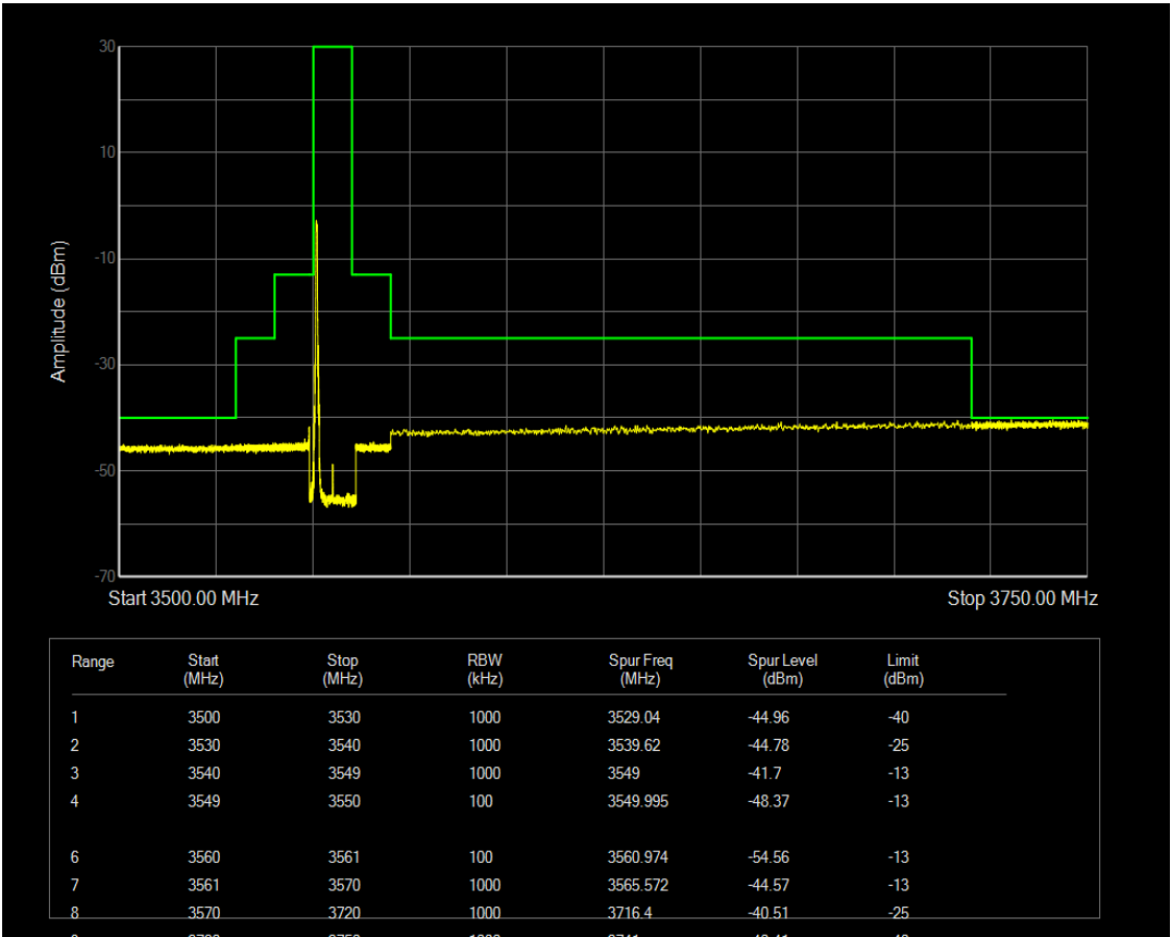
n78(3550-3700) SCS=30kHz CP_QPSK BW=10MHz Channel=637000 RB=1@23
