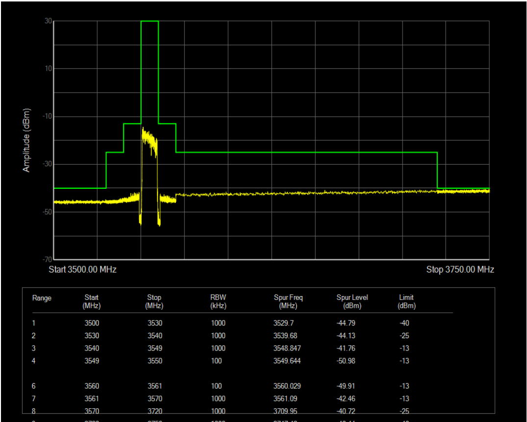
n78(3550-3700) SCS=30kHz CP_QPSK BW=10MHz Channel=646332 RB=1@0
