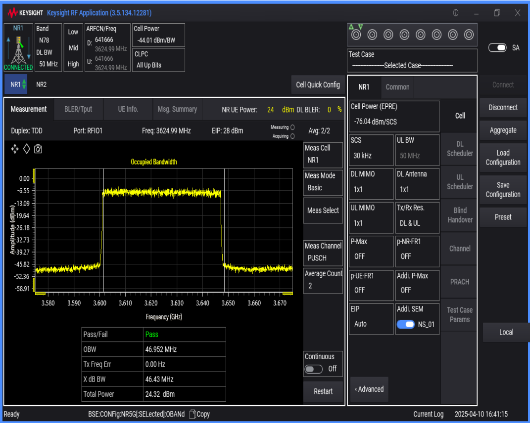
n78(3550-3700) SCS=30kHz DFT_QPSK BW=60MHz Channel=641666 RB=162@0
