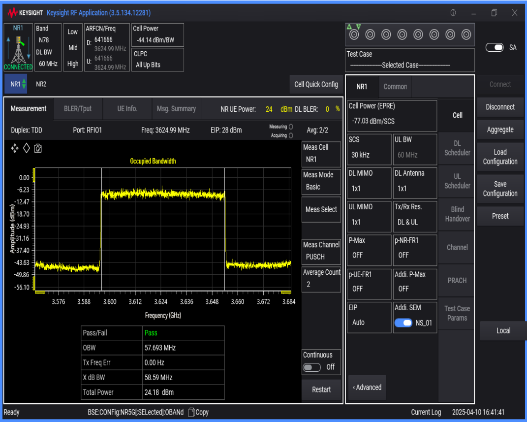
n78(3550-3700) SCS=30kHz DFT_QPSK BW=70MHz Channel=641666 RB=180@0
