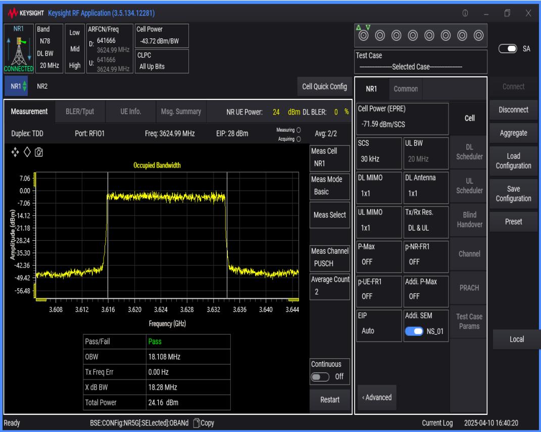
n78(3550-3700) SCS=30kHz DFT_QPSK BW=40MHz Channel=641666 RB=100@0
