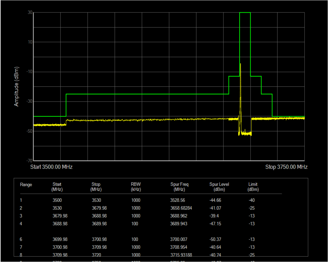
n78(3550-3700) SCS=30kHz CP_QPSK BW=10MHz Channel=646332 RB=24@0
