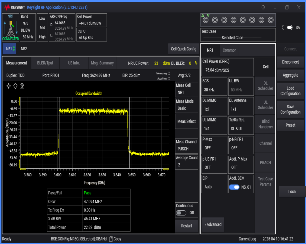
n78(3550-3700) SCS=30kHz DFT_QAM64 BW=60MHz Channel=641666 RB=162@0
