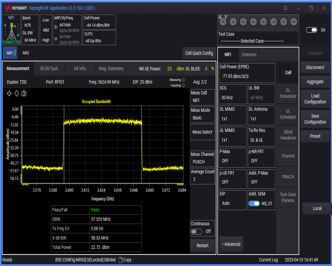
n78(3550-3700) SCS=30kHz DFT_QAM64 BW=80MHz Channel=641666 RB=216@0
