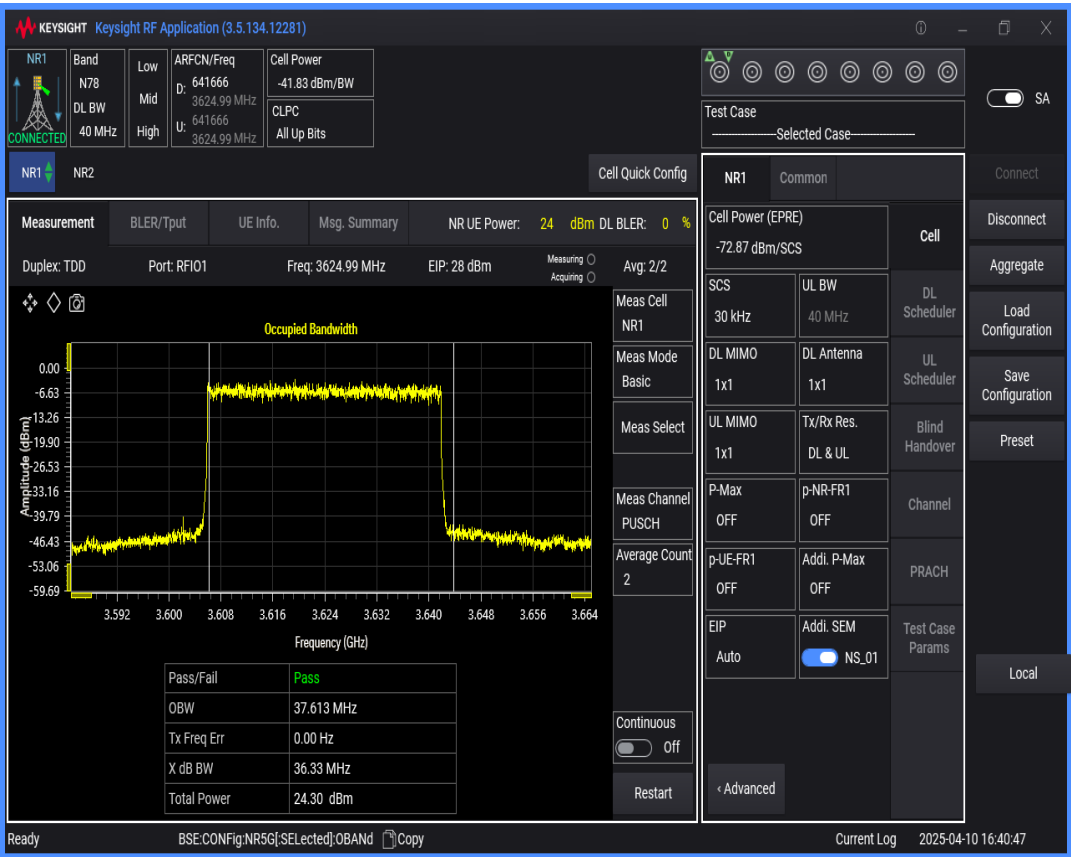
n78(3550-3700) SCS=30kHz DFT_QPSK BW=50MHz Channel=641666 RB=128@0
