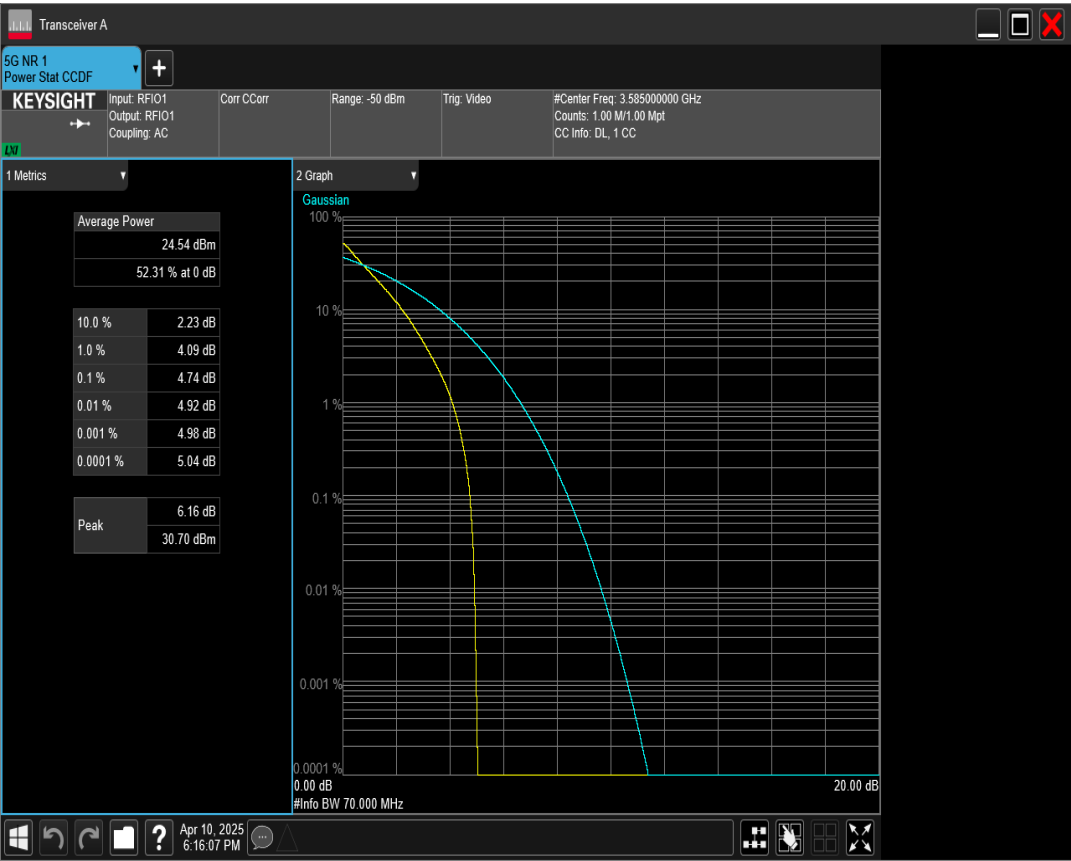
n78(3550-3700) SCS=30kHz DFT_BPSK BW=60MHz Channel=644666 RB=162@0
