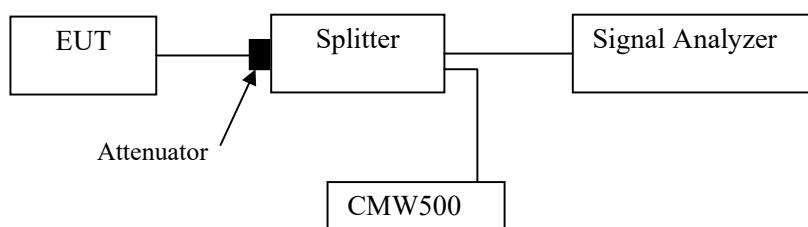
**Transmitter unwanted emissions-at antenna terminals**
