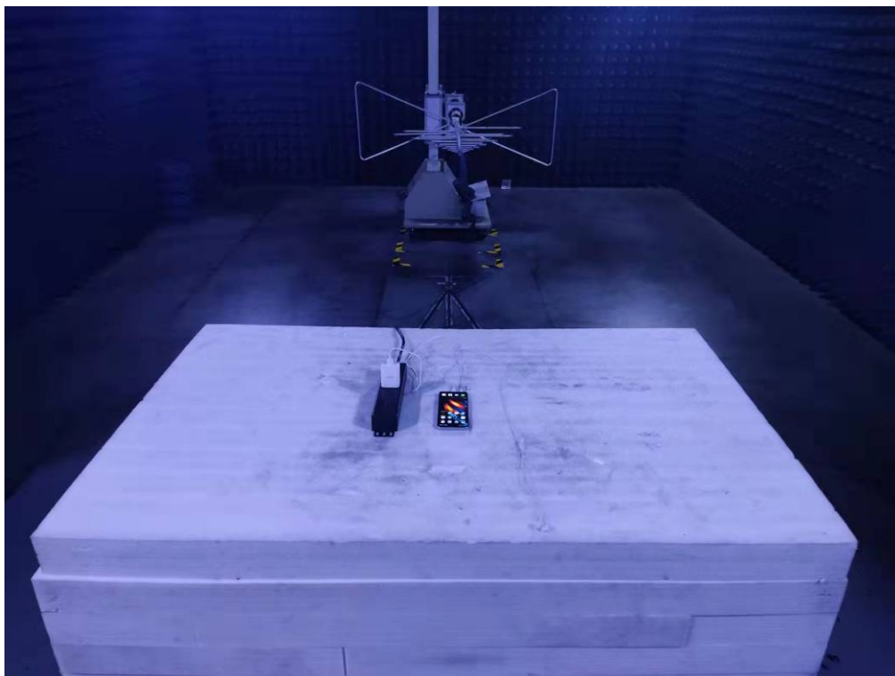
Photo of Radiated Emission Measurement (Below 1G)
