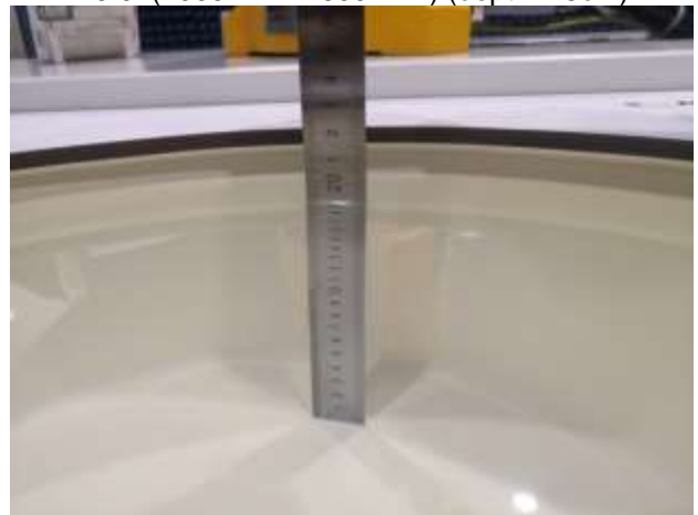
Fig. 9.8 Photo of Liquid Height for Body SAR of Twin Phantom (5200MHz~5800MHz) (depth>15cm)
