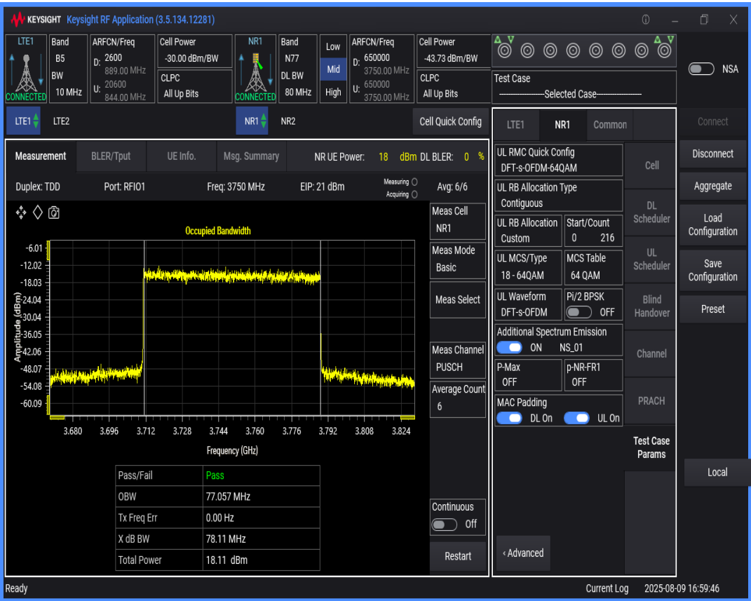
n77 SCS=30kHz DFT_QPSK BW=60MHz Channel=650000 RB=162@0
