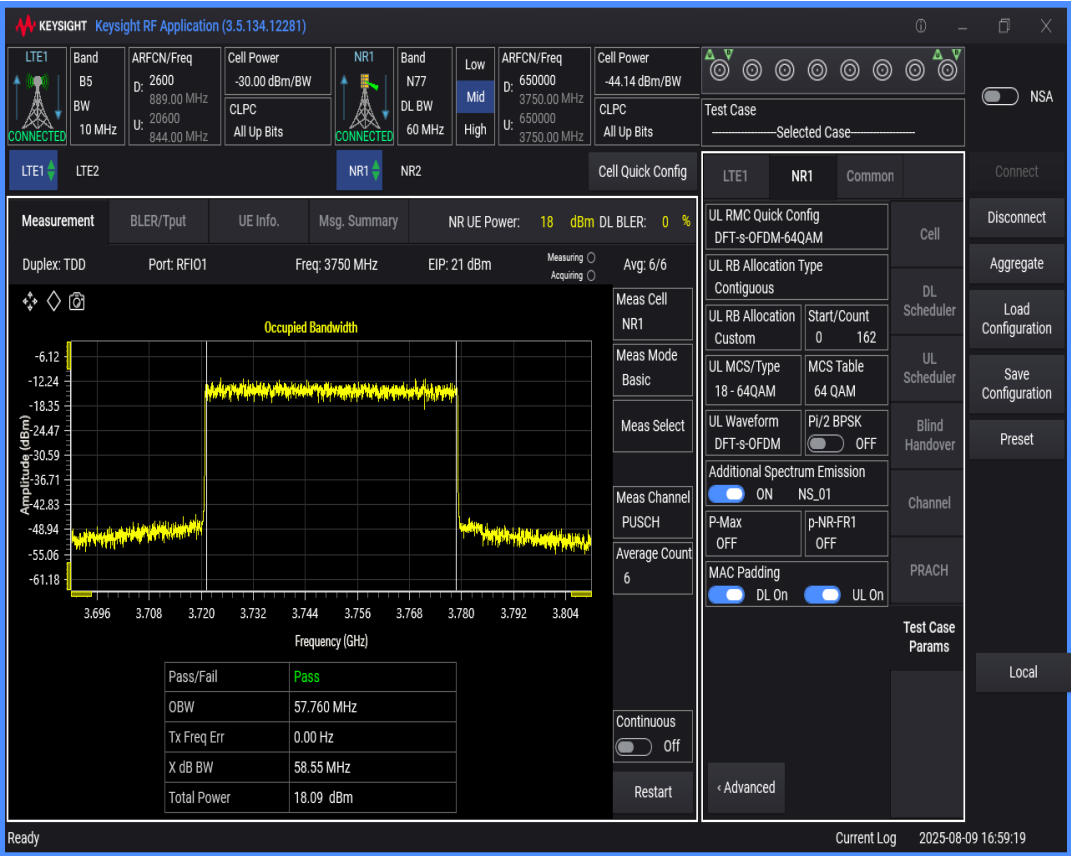
n77 SCS=30kHz DFT_QAM64 BW=80MHz Channel=650000 RB=216@0
