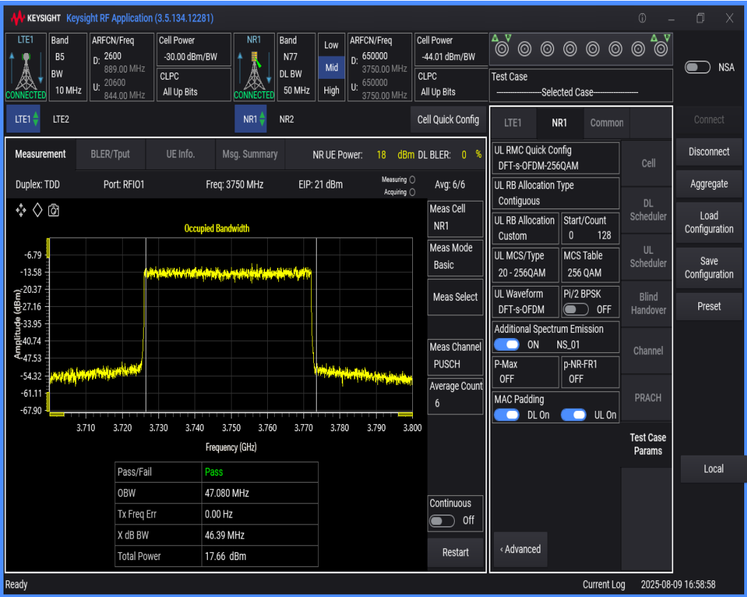
n77 SCS=30kHz DFT_QAM256 BW=60MHz Channel=650000 RB=162@0
