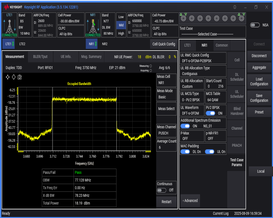
n77 SCS=30kHz DFT_BPSK BW=90MHz Channel=650000 RB=240@0
