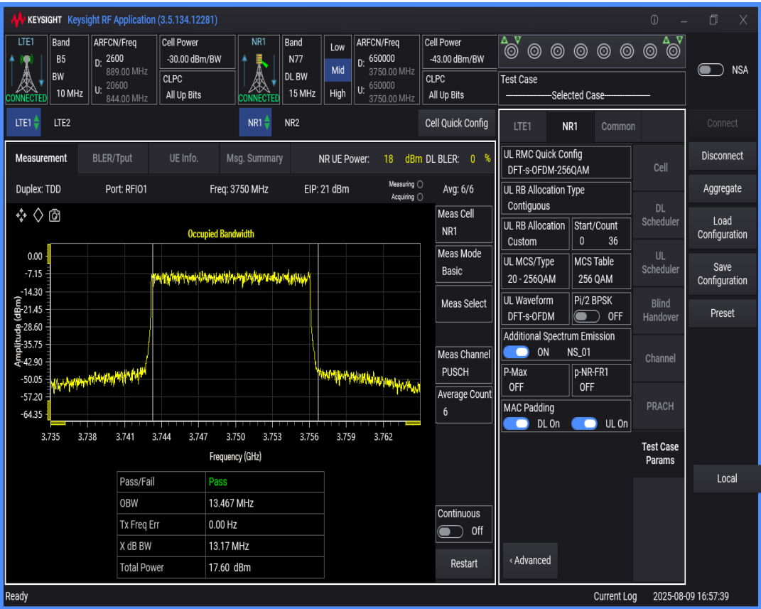
n77 SCS=30kHz DFT_QAM64 BW=15MHz Channel=650000 RB=36@0
