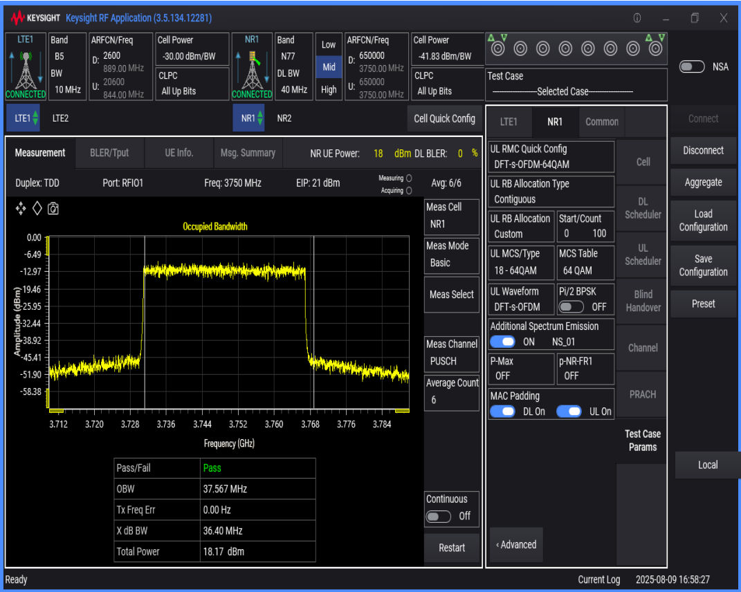
n77 SCS=30kHz DFT_QAM64 BW=10MHz Channel=650000 RB=24@0
