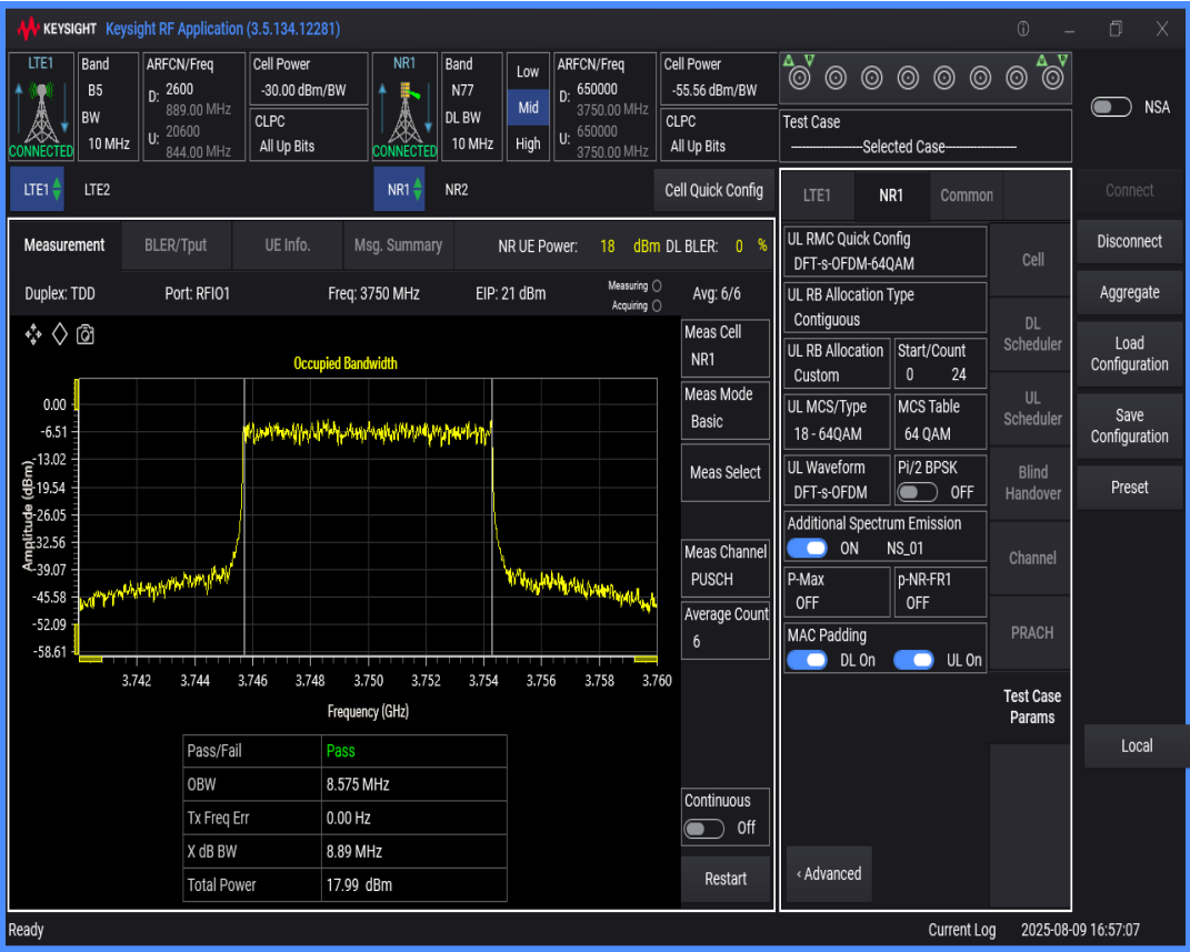
n77 SCS=30kHz DFT_QAM256 BW=80MHz Channel=650000 RB=216@0
