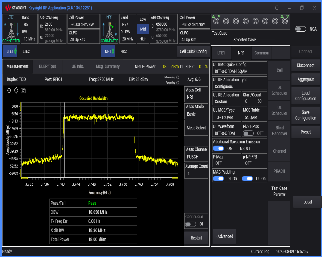
n77 SCS=30kHz DFT_BPSK BW=80MHz Channel=650000 RB=216@0
