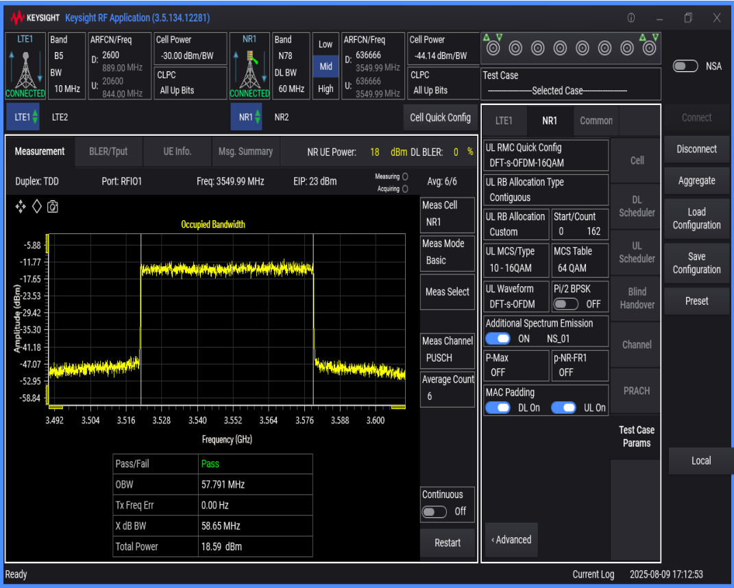
n78 SCS=30kHz DFT_QAM256 BW=80MHz Channel=636666 RB=216@0
