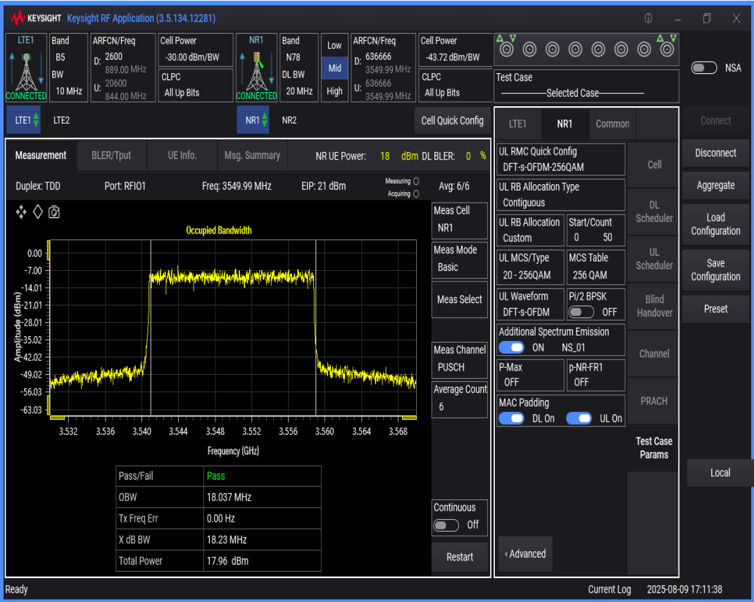
n78 SCS=30kHz DFT_QAM256 BW=40MHz Channel=636666 RB=100@0
