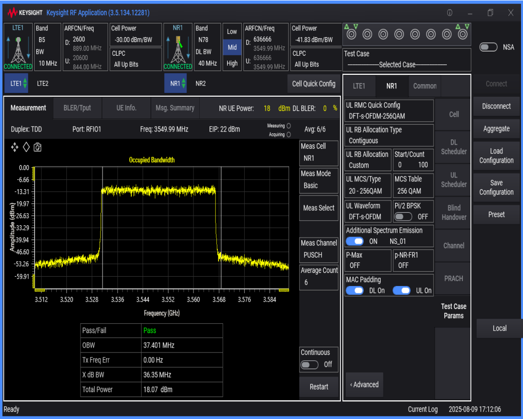
n78 SCS=30kHz DFT_QAM256 BW=50MHz Channel=636666 RB=128@0
