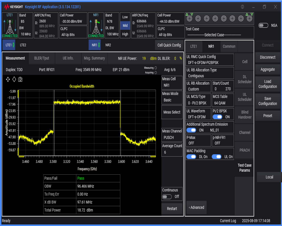
n78 SCS=30kHz DFT_BPSK BW=10MHz Channel=636666 RB=24@0
