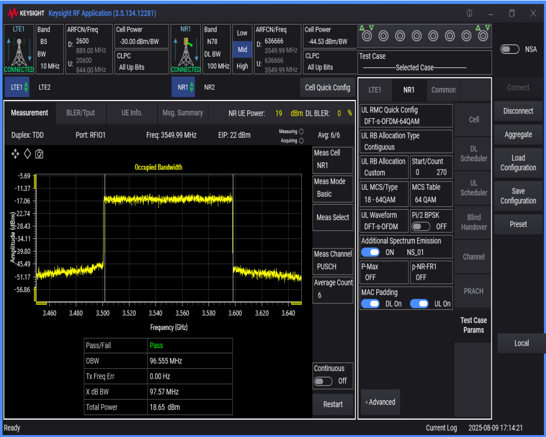
n78 SCS=30kHz DFT_QAM256 BW=60MHz Channel=636666 RB=162@0
