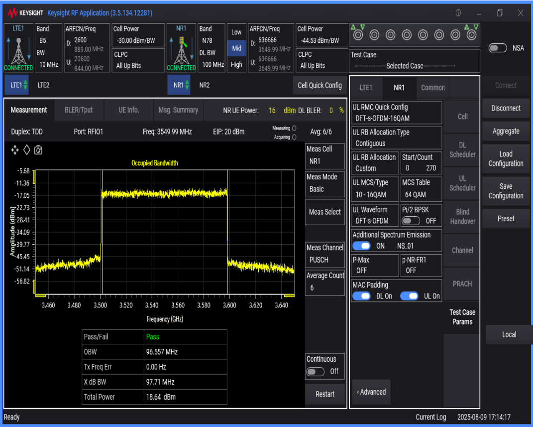
n78 SCS=30kHz DFT_BPSK BW=90MHz Channel=636666 RB=240@0
