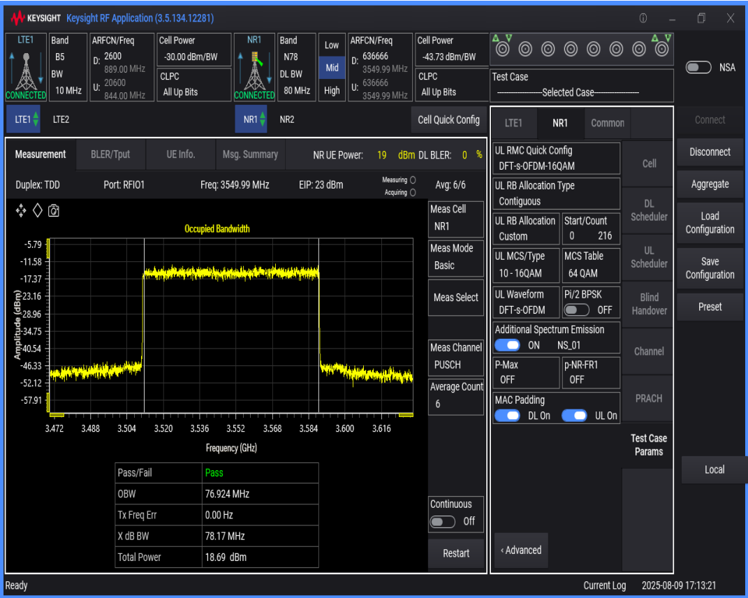
n78 SCS=30kHz DFT_QAM16 BW=60MHz Channel=636666 RB=162@0
