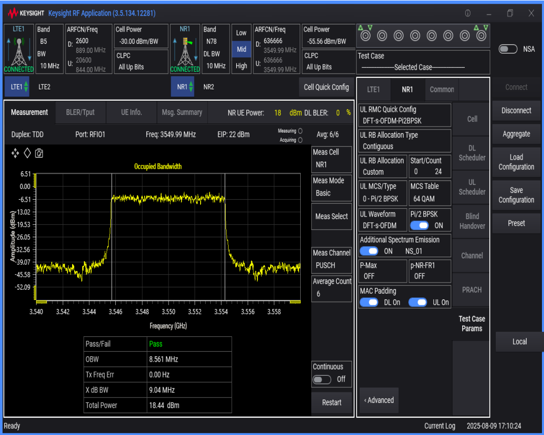
n78 SCS=30kHz DFT_QAM16 BW=100MHz Channel=636666 RB=270@0
