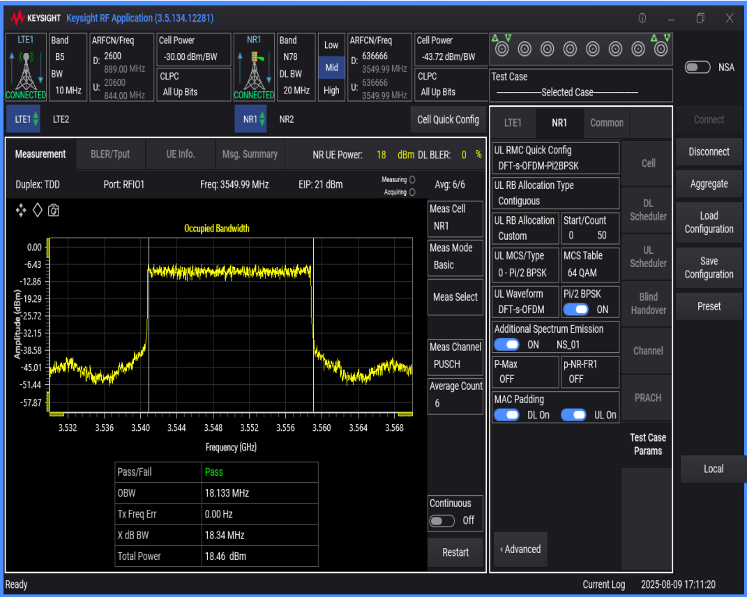
n78 SCS=30kHz DFT_BPSK BW=100MHz Channel=636666 RB=270@0
